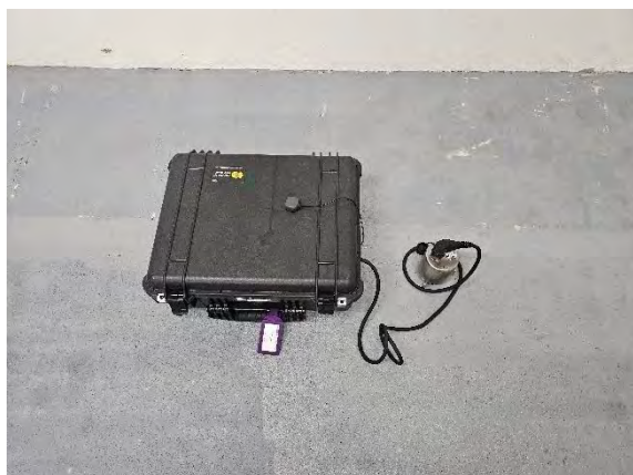
(a) Photo of the typical placement of a broadband seismometer at the foundation level of a building on a concrete pad. The silver cylinder is a three-component seismometer, and the data logger is inside the black case.
