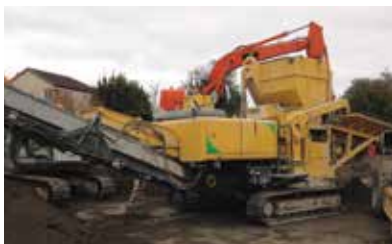
A pug mill as sometimes used to mix soil and cement together
