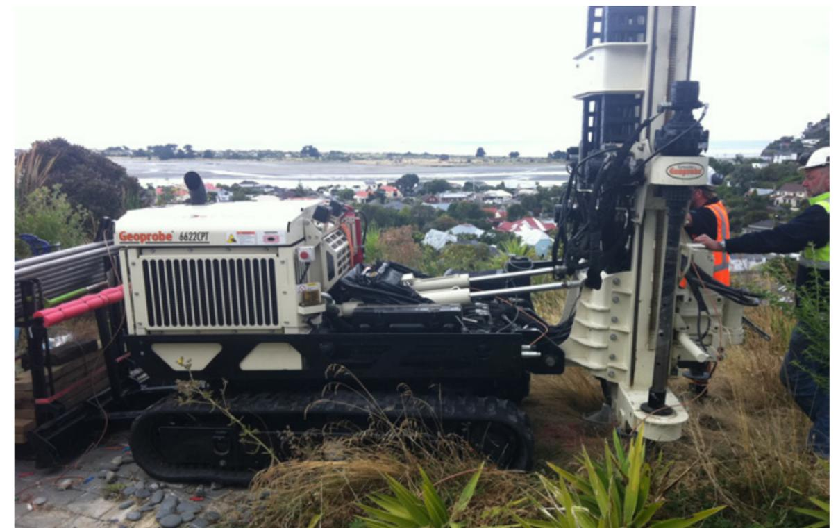
A machine drilling a borehole to assist in geological profiling of land in Canterbury affected by the earthquakes. Photo: Tonkin & Taylor.
