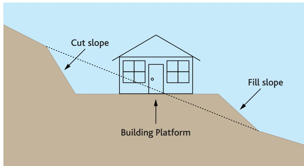
Figure 3.1 shows how a slope is cut into the hill on the upslope side of a hillside house and filled out to make a level platform on the down slope side.
