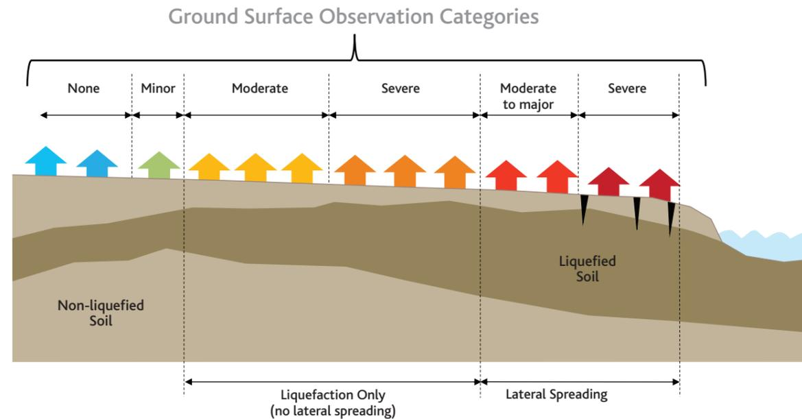
Figure 4.1 Schematic section of spatial distribution of categories of the Plains liquefaction and lateral spread observations
