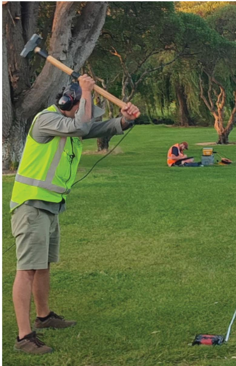
RESEARCHERS FROM THE UNIVERSITY OF CANTERBURY USE A SLEDGEHAMMER TO CREATE VIBRATIONS WHICH ARE RECORDED BY THE SENSORS TO DETERMINE THE COMPOSITION OF THE SOILS BELOW
