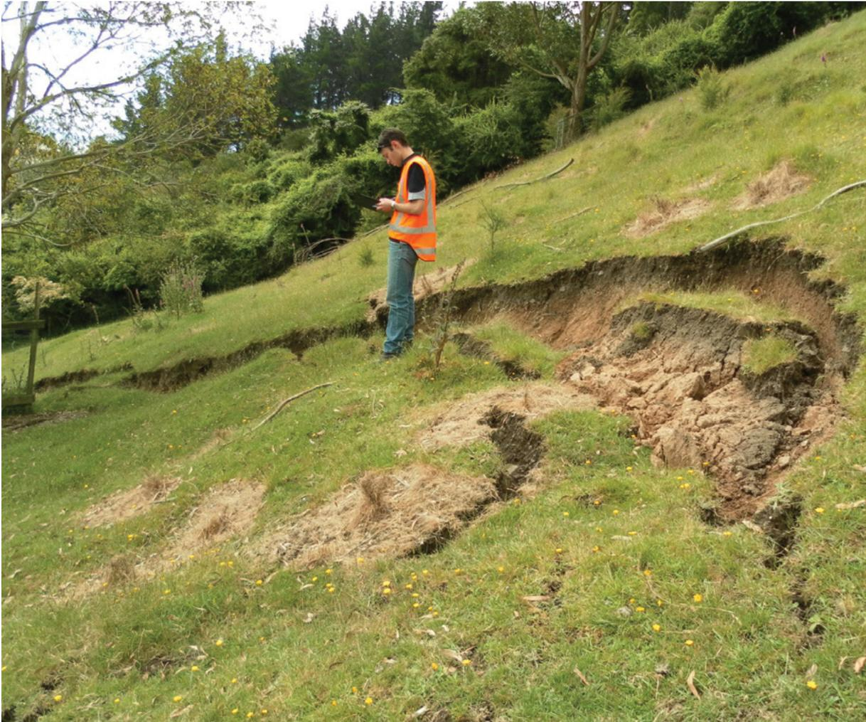
A GEOLOGIST MAPPING A LANDSLIDE
