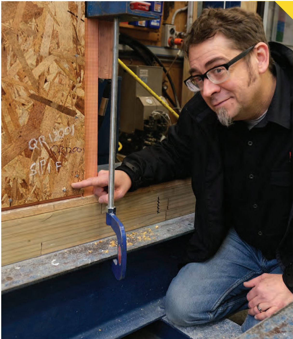
▶ Dr David Carradine checks SIPs panel performance after a test round
