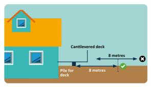
Residential land covered - start point of measurement of the 8 metres. Cantilevered deck example.
