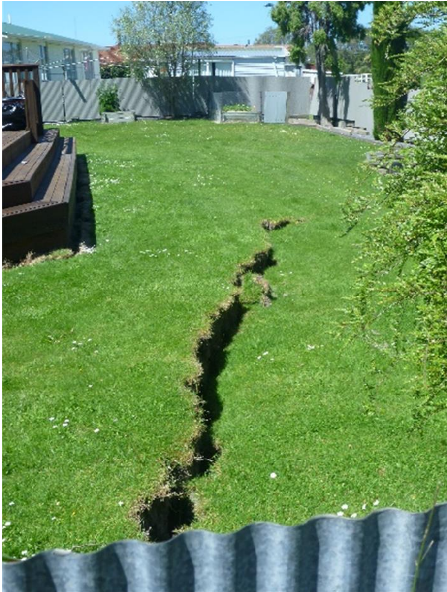
Figure 33 Cracking (lateral spreading) due to earthquake
