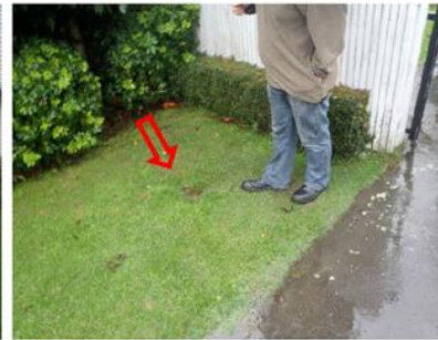
Figure 4: Depression in ground where fissure extends
