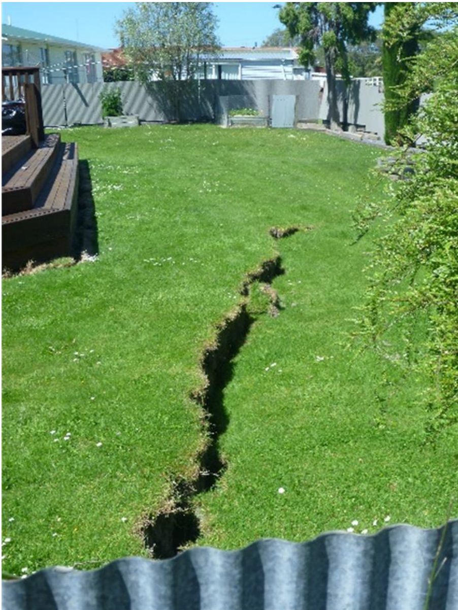
Figure 32 Cracking (lateral spreading) due to earthquake
