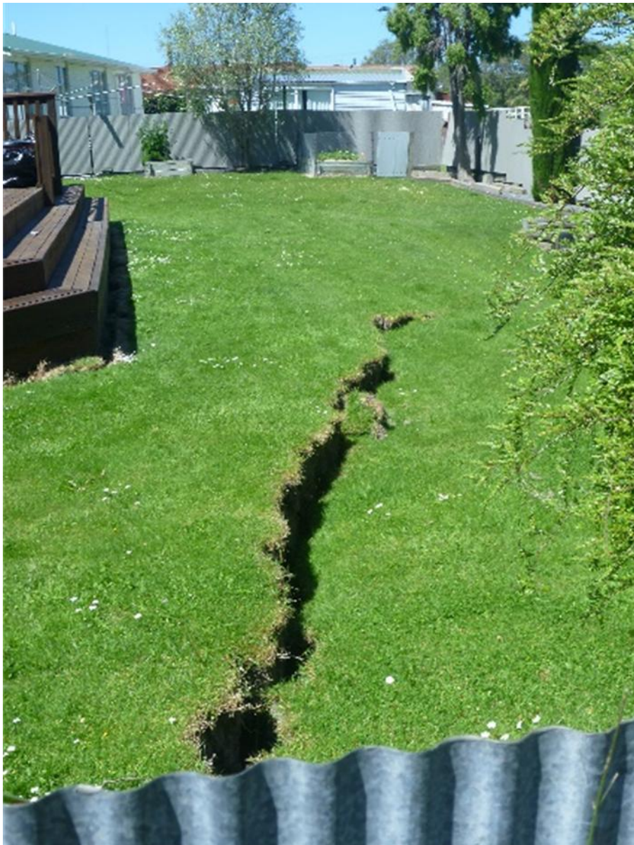
Figure 32 Cracking (lateral spreading) due to earthquake
