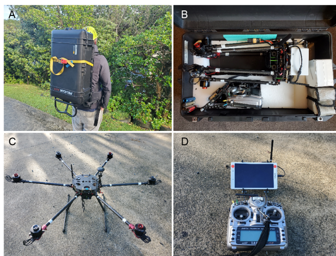
Figure 1. UAS system. A. Operator with full UAS and all modules carried comfortably in a single box. B. Interior of the box, with UAS, controller, multiple instruments and batteries. C. The hexacopter (without instrument) that is the final design from this work. D. The pilot's transmitter, with tablet for flight data and receiving radio for Universal Data Telemetry system.
