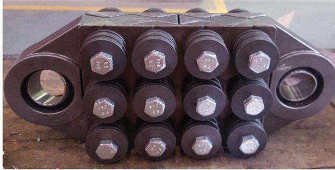
**Figure 16: RSFJ for column testing**
