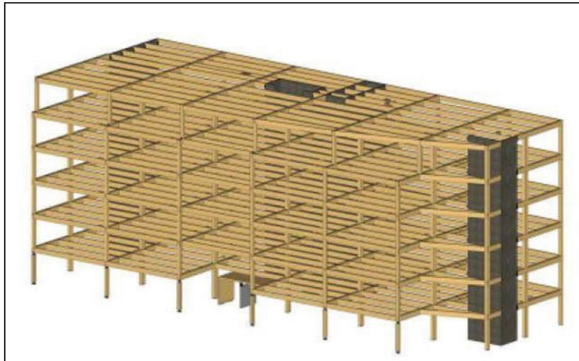
Figure 5: Six storey wood and concrete hybrid building structure [16]
