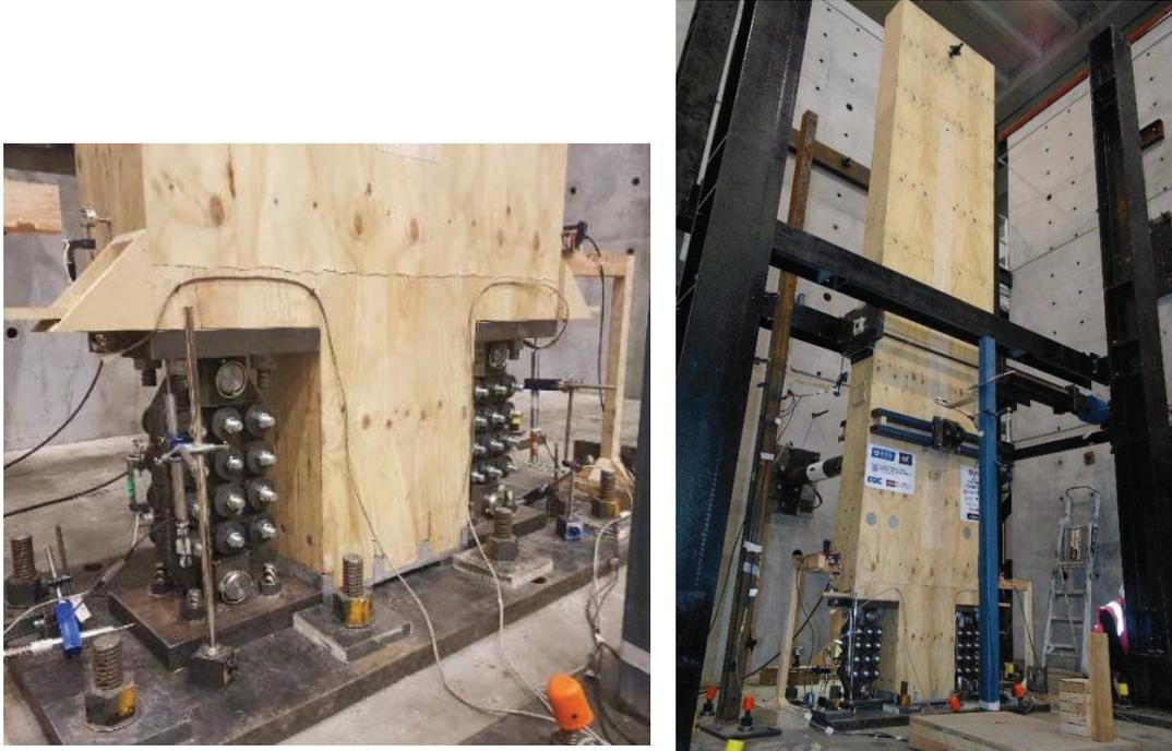
**Figure 17: Experimental setup for testing the column**
