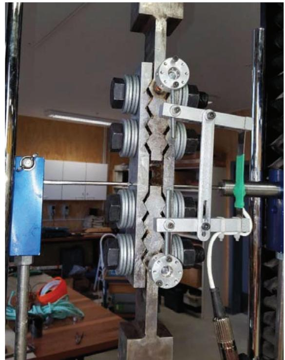
**Figure 11: The RSF joint lubricated with grease 1000 kN joint**
