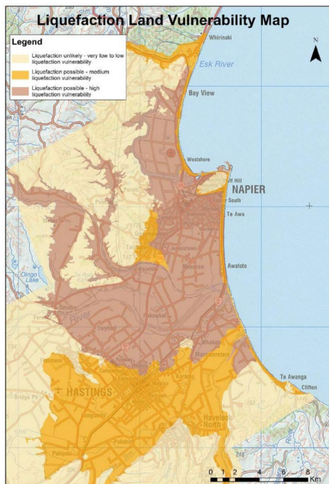
Figure 1: Liquefaction land vulnerability map showing areas of high, medium and low vulnerability (GNS Science, 2007, p87).
