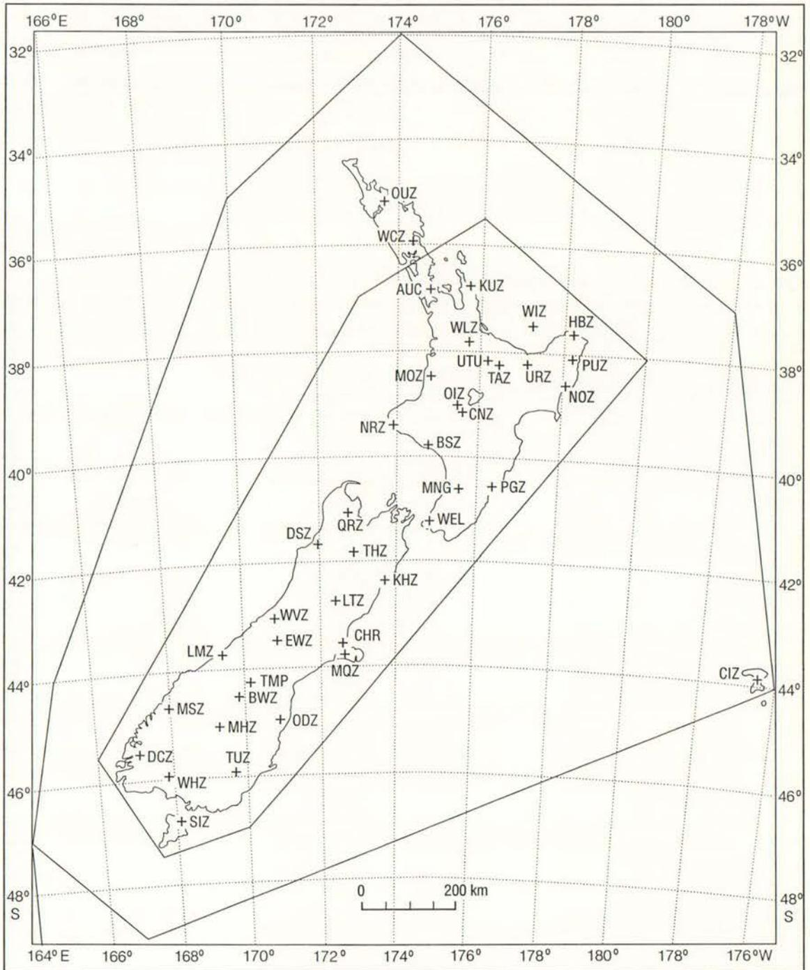
**Figure 2.** Local networks at Wellington, Hawke's Bay, Chateau, Rotorua and Clyde are too closely spaced to be shown on this map. The inner and outer polygons define three areas where accuracy of epicentre locations is considered reliable, less reliable and inadequate.
