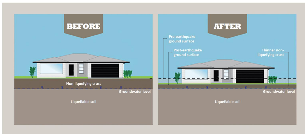
Figure 3: Increased Liquefaction Vulnerability – how ground surface subsidence made some properties more vulnerable to liquefaction
