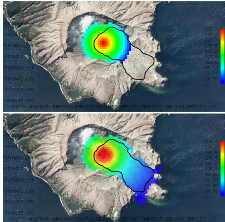
**Figure 8. (top)** Energy grade line surge propagation for White Island case study with  $\alpha = 35^\circ$  using equation 5, **(bottom)** energy grade line surge propagation for White Island case study with  $\alpha = 35^\circ$  using equation 6.
