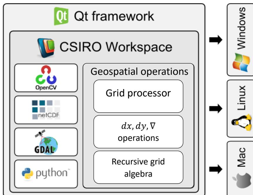
**Figure 11.** Architecture underlying the level set simulator and surge modelling framework. Built on the multi-platform Qt framework and CSIRO Workspace scientific workflow tool enables leveraging of open libraries (e.g. OpenCV, netCDF, GDAL) and already build components (e.g. Geospatial operations from other funded projects).
