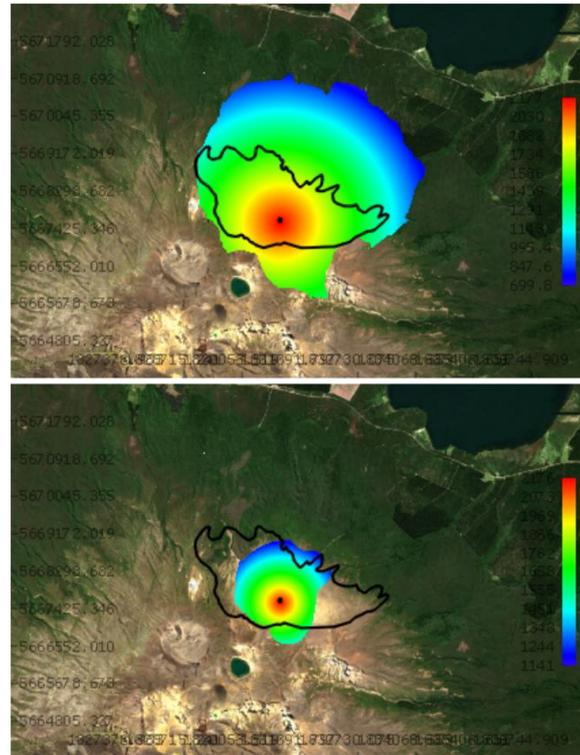
**Figure 7. (top)** Energy grade line surge propagation for Te Maari case study with  $\alpha = 22^\circ$ , **(bottom)** energy grade line surge propagation for Te Maari case study with  $\alpha = 35^\circ$ .
