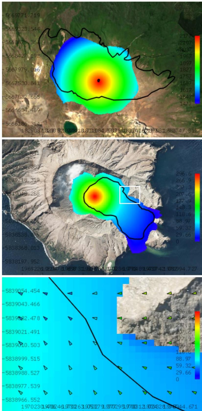
**Figure 10. (top)** Energy grade line surge propagation for Te Maari case study with  $\alpha = 22^\circ$  using the potential flow terrain correction, **(middle)** energy grade line surge propagation for White Island case study with  $\alpha = 35^\circ$  using equation 6 and potential flow correctin. **(bottom)** zoom of boxed area in middle showing vectors that act as a sink to surge energy.
