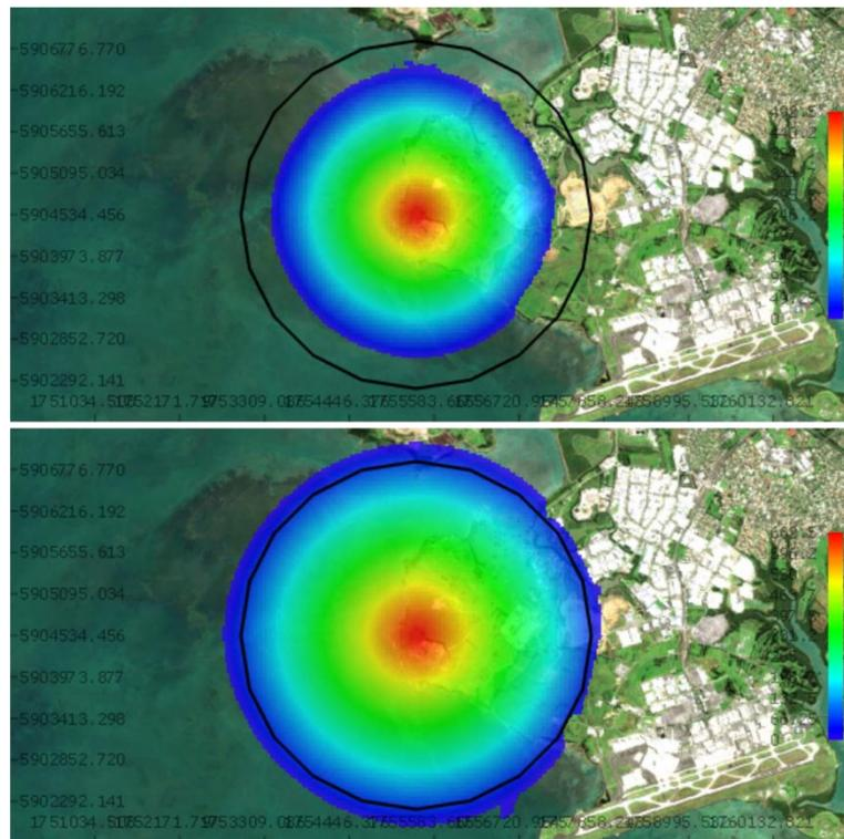
**Figure 9. (top)** Energy grade line surge propagation for Maungataketake case study with  $\alpha = 15^\circ$ , **(bottom)** energy grade line surge propagation for Maungataketake case study with  $\alpha = 15^\circ$  using an energy ( $h_{v0}$ ) similar to the Te Maari case.
