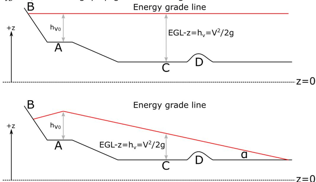
**Figure 6. (top)** Energy grade line approach under frictionless assumptions, **(bottom)** energy grade line under a linear energy dissipation approach.
