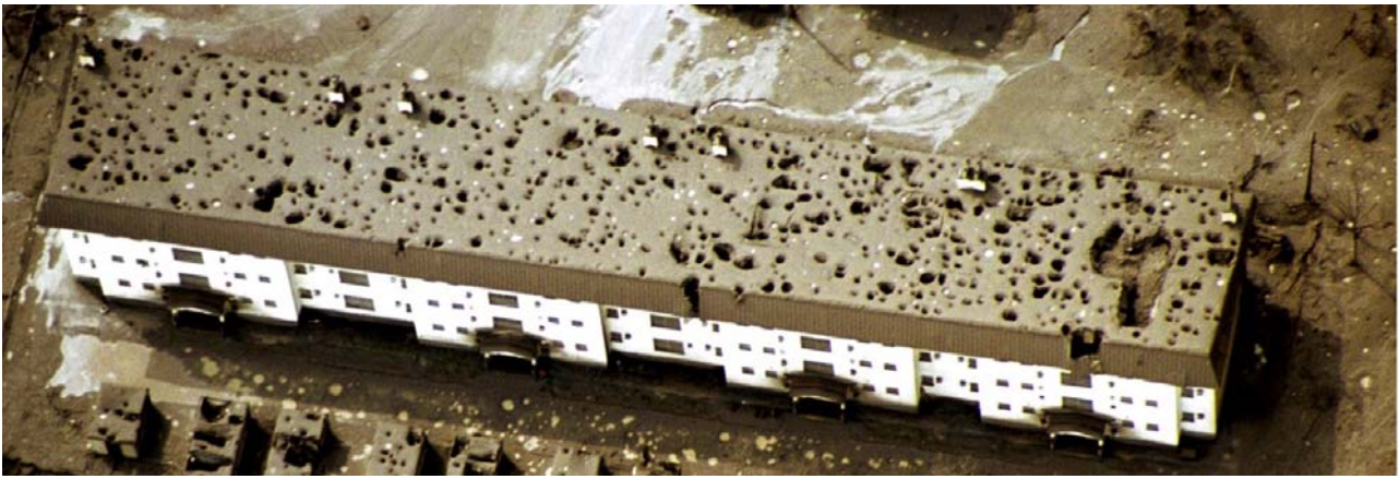
Figure 1. A roof impacted by ballistics during the 2000 eruption of Usu volcano (photo courtesy of Professor Okada).
