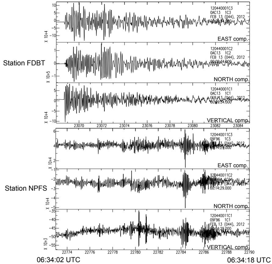
Figure 5: Shot 3 recorded on the two temporary stations FDBT and NPFS. The low SNR of station NPFS can be seen.
