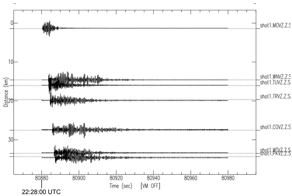
Figure 4: Seismographs showing vertical acceleration caused by shot 1 across GeoNet stations local to the Ruapehu vicinity, plotted relative to their distance to the Lake Moawhango blasts.
