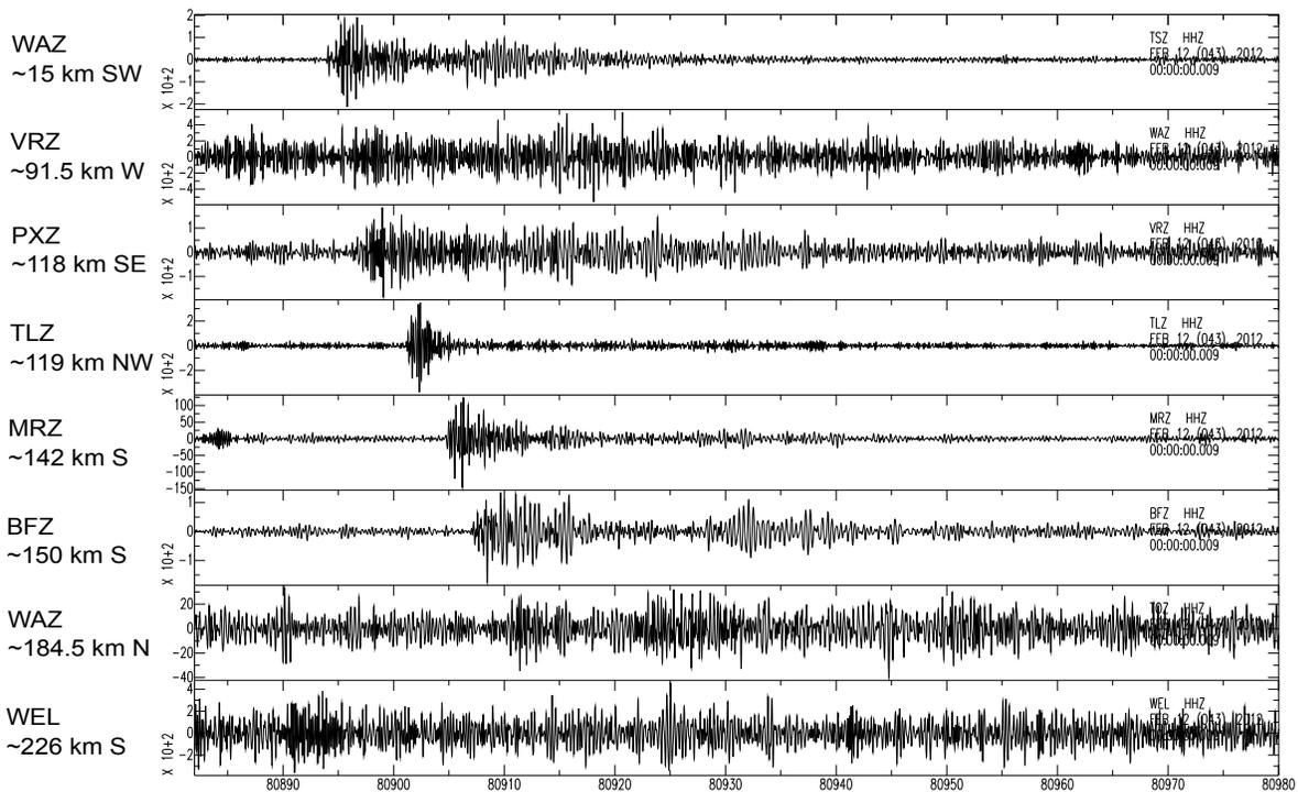
Figure 3: Seismographs showing vertical acceleration caused by shot 1 across GeoNet stations in the North Island (see <http://www.geonet.org.nz/resources/network/netmap.html> for detailed locations) and their approximate distances from Lake Moawhango. The time series have been put through a 2-10 Hz band pass filter. For reference, station WEL is located in Wellington City.
