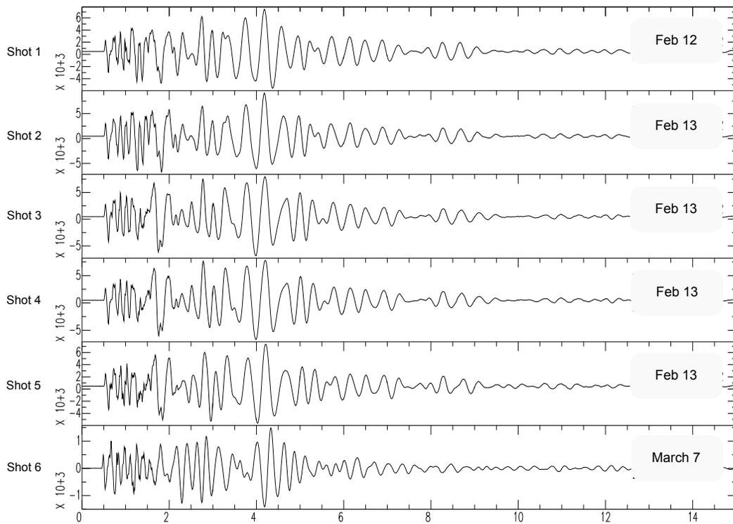
Figure 6: Vertical acceleration component seismograms from GeoNet station MOVZ showing all 6 shots. The first five shots were all taken within 24 hours of one another. Shot 6 was taken almost a month later. Amplitudes for shot 1-5 are consistent with one another, however the amplitudes reached in shot 6 are about 20% of the others. Dates are for shot timings in UTC.
