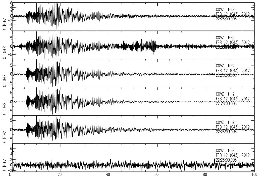
Figure 9: Similarly to the last figure, this shows vertical acceleration component seismograms from borehole station WNVZ showing each of the shots. Note that COVZ is further from the source than WNVZ, and the final shot has attenuated to below the level of noise at the station.
