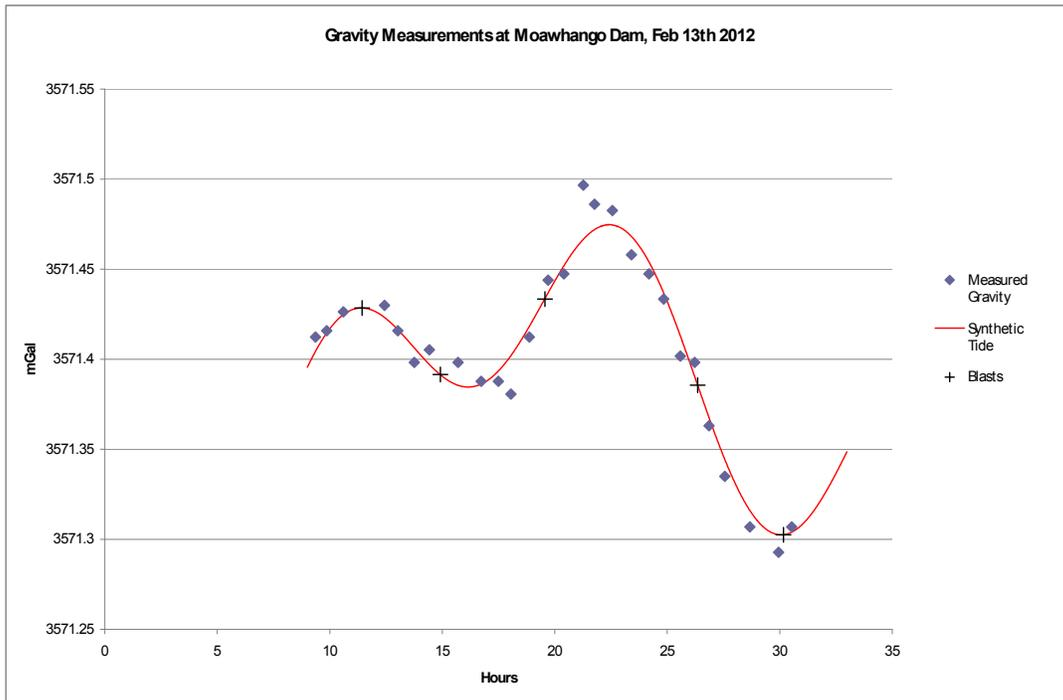
Figure 2: Gravity measurements and synthetic tide calculations over the course of the experiment showing the variation in gravitational acceleration.
