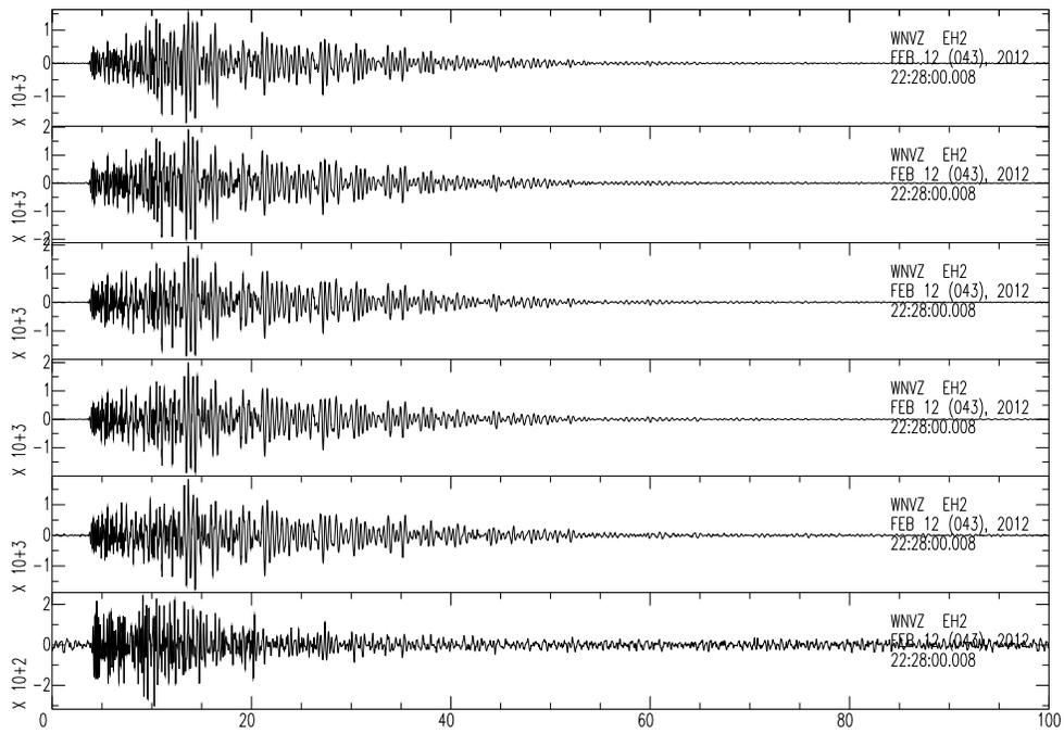
Figure 8: Vertical acceleration component seismograms from borehole station WNVZ showing all 6 shots, filtered with a band pass of 1-10Hz. Shots are ordered 1-6 from top to bottom, similarly to figure 6.
