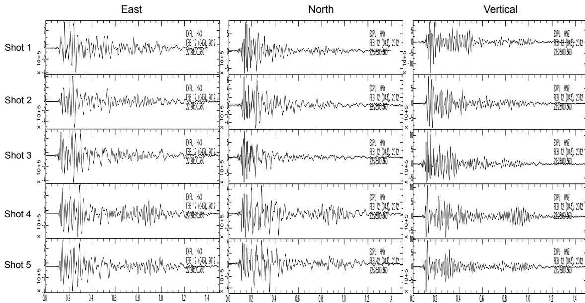
Figure 7: Strong motion acceleration records from the on-site accelerometer for the first 5 shots. The accelerometer was located close to the point at which the explosives were detonated. The waveforms show less correlation than can be seen on more distant seismometers, possibly due to the accelerometer's proximity to the detonation charges.
