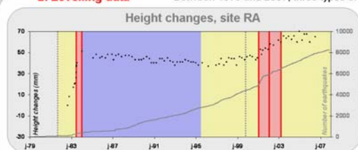
Fig. 3. Comparison between height changes (black points, mm) on site RA relative to the origin (see Figure 4 for the location of sites) and the cumulative number of earthquakes (grey) recorded between 1979 and 2007 at Lake Taupo. The fill colours highlight changes in the global deformation trend.
