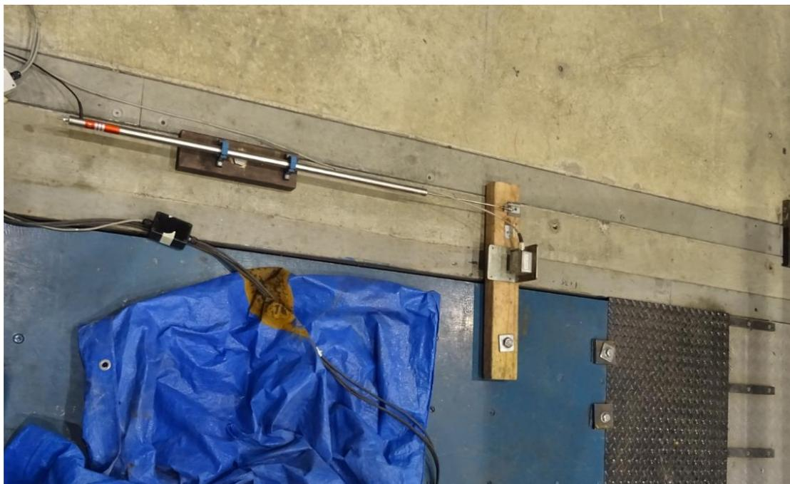
Figure 2.9. LVDT and accelerometer at the table
