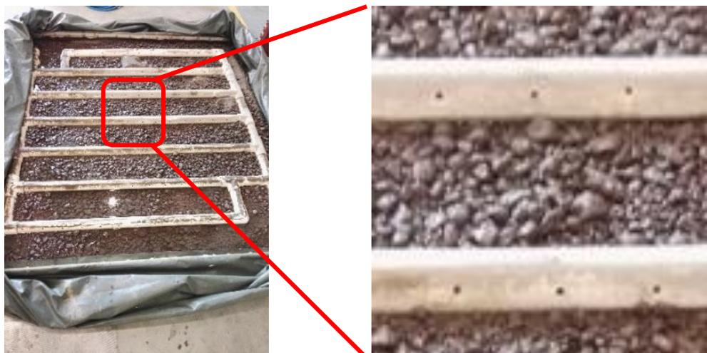
Figure 4.2. Pipe system at the base of the laminar box
