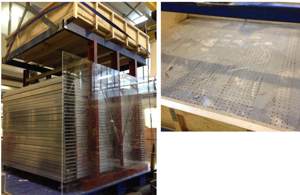
Figure 2.6. Test set-up. Laminar box with the raining box above
