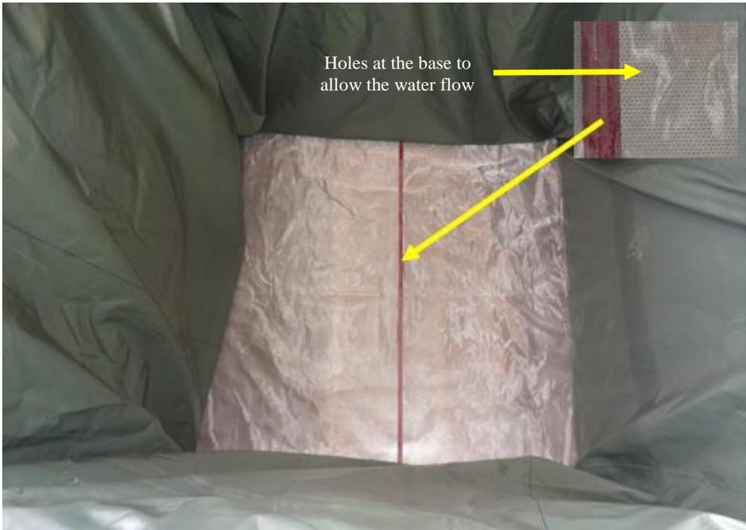
Figure 2.4. Top view of base and lateral membrane
