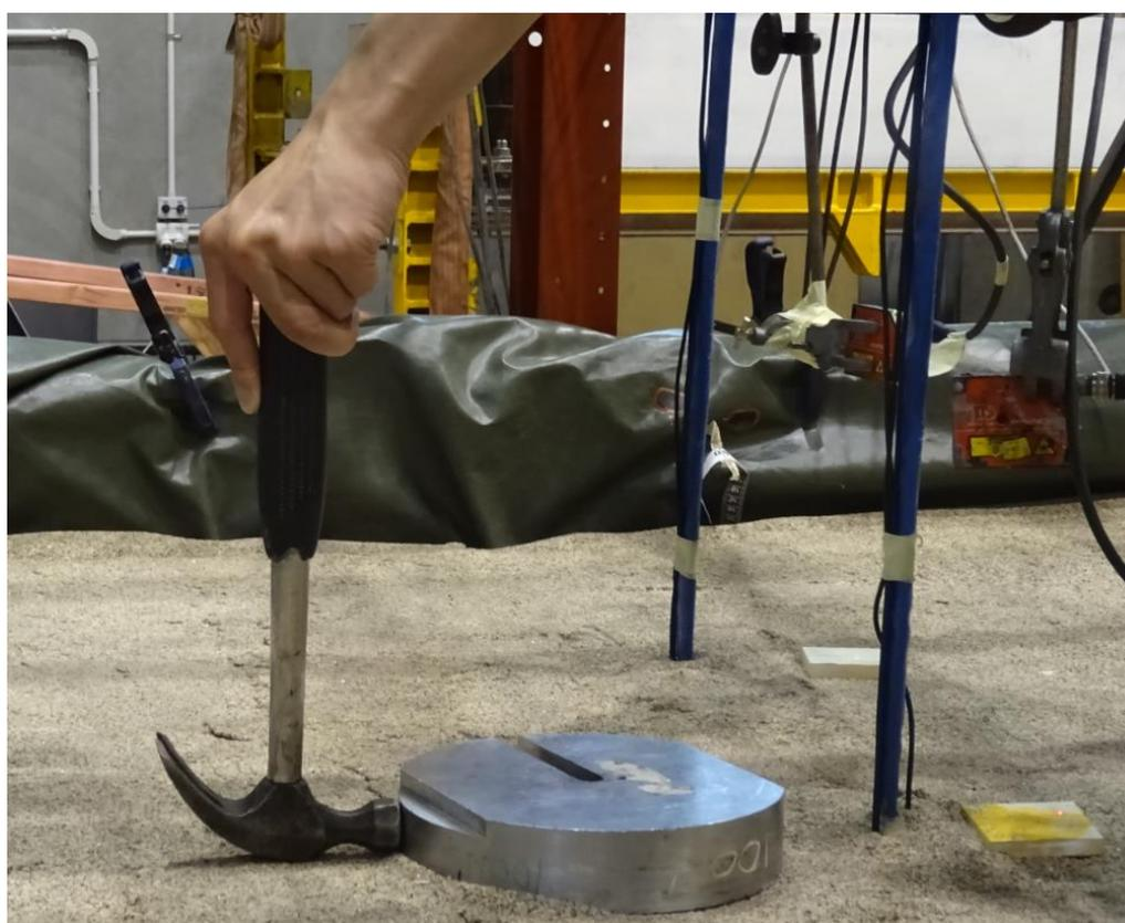
Figure 2.10. Impact tests to obtain the shear wave velocity
