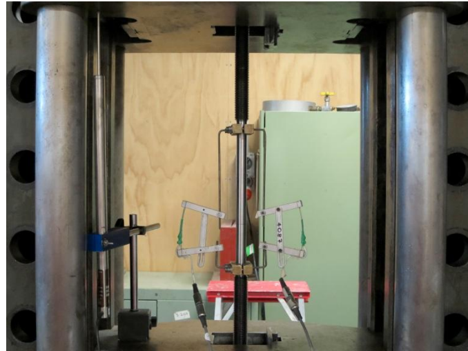
Figure 5: Tensile Testing of a Threaded Rod
