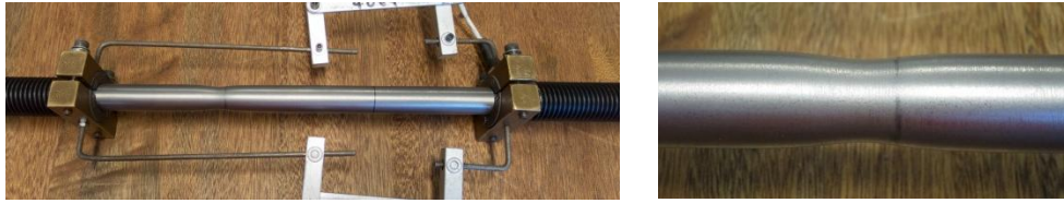
Figure 7: M30 Plain Class 8.8 Threaded Rod with M24 Shank a) Yielded Threaded Rod; b) Yielding Region
