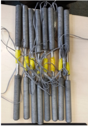
a) Application of strain gauge
