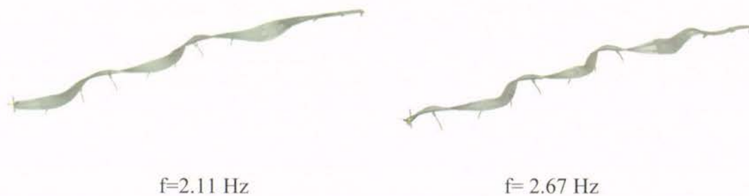
Figure 5.22. Selected horizontal mode shapes of the Southbound Bridge obtained by numerical analysis.
