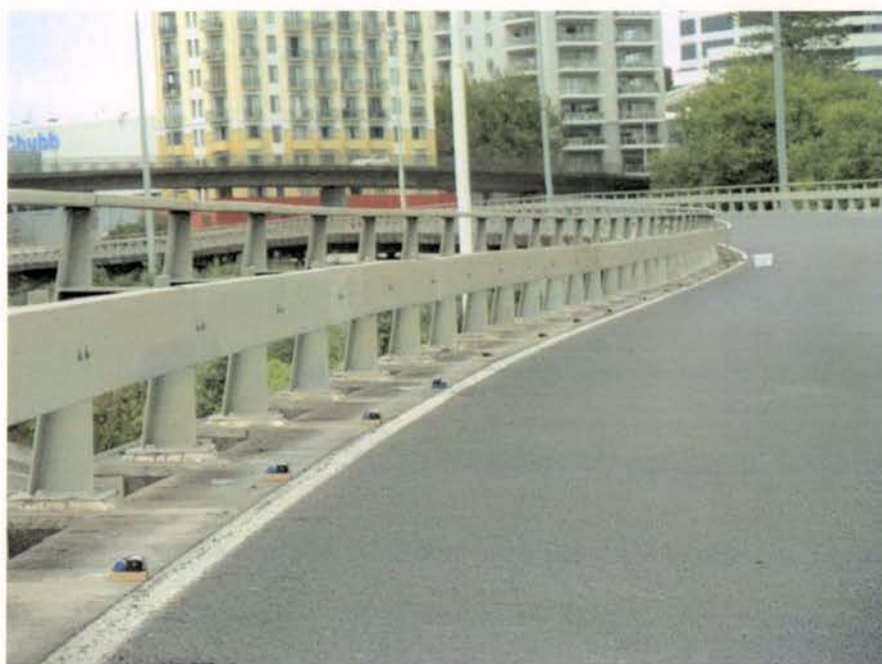
Figure 6.19. USB accelerometers arranged along the bridge curbs.
