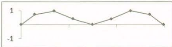
Mode 5 (1 st horizontal): Frequency 5.33 Hz
