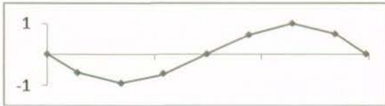
Mode 1 (1 st vertical): Frequency 1.64 Hz
