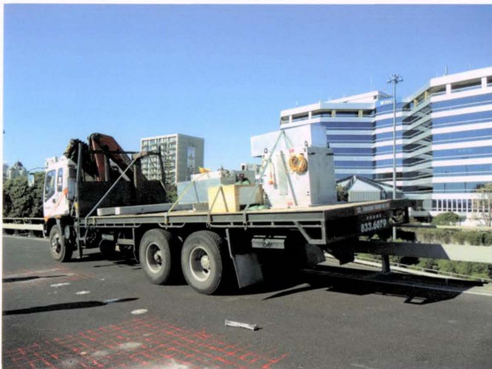
Figure 6.34. Transporting shakers with hiab truck.
