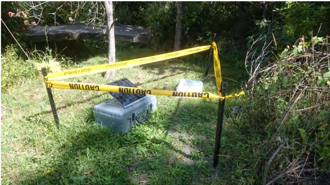
Figure 3: An example of the portable seismometer deployment.
