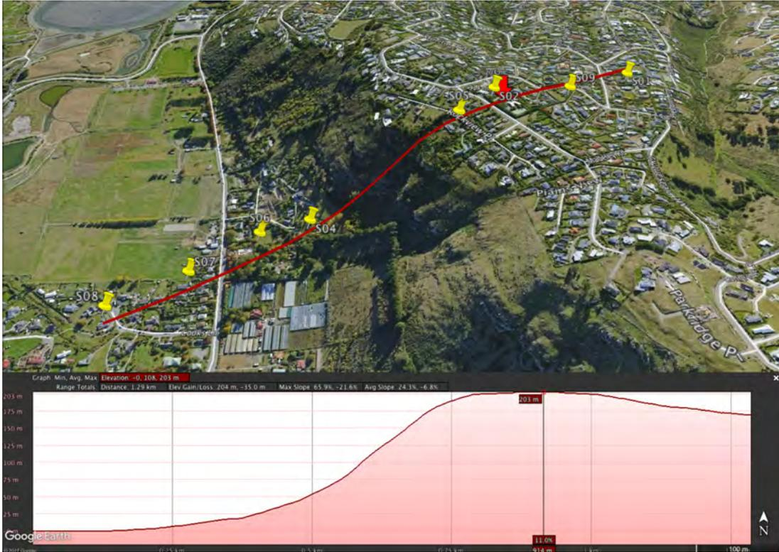
Figure 2: Location of experimental transect in Heathcote Valley / Mt Pleasant, indicating sensor locations and topographic profile.
