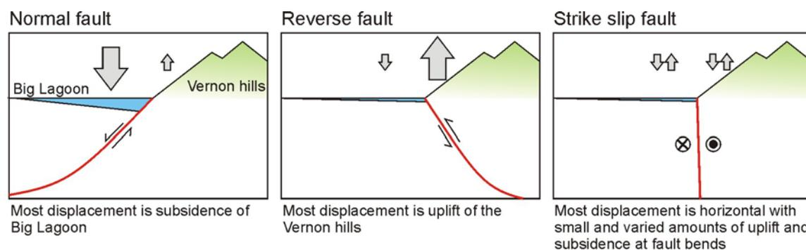
Figure 13 Simple faulting scenarios of the Vernon fault along the Big Lagoon segment. Each scenario illustrates the dominant absolute movements associated with each type of fault: normal fault, reverse fault, strike-slip fault.
