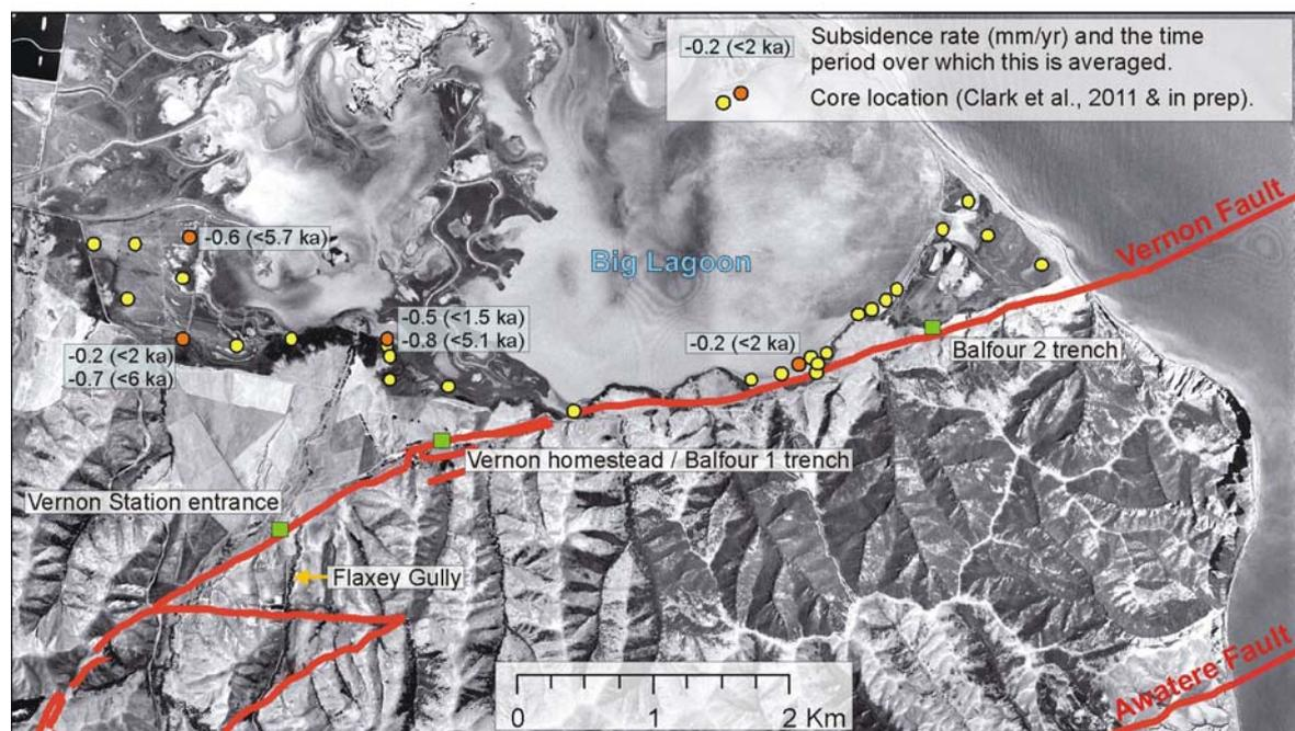
Figure 2 Airphoto of the section of the Vernon fault adjacent to Big Lagoon. The Vernon fault location is from the NZ Active Faults Database. The locations of detailed investigation in this study are shown by the green boxes. The location of cores obtained for paleo-sea level studies by Hayward et al. (2010) and Clark et al. (2011 and in prep) are shown, along with the rates of Holocene subsidence.
