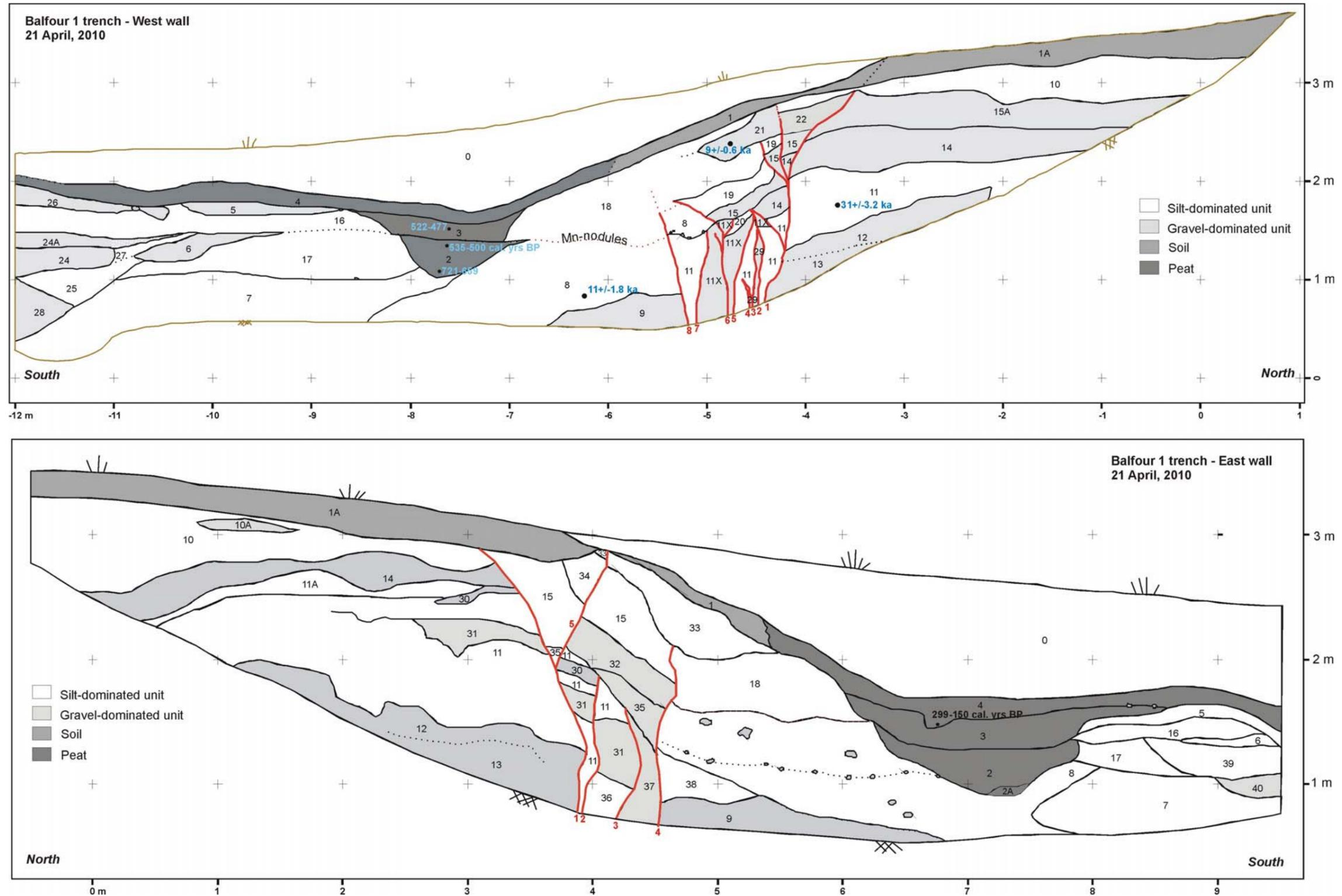
Figure 7 Trench logs of the Balfour 1 trench. All unit descriptions are in Table 2, Unit numbering does not follow stratigraphic order. Faults are numbered in bold red numerals, the fault numbering does not signify correlation between the two walls. Trench location: NZMG 5960096N/2600076E.
