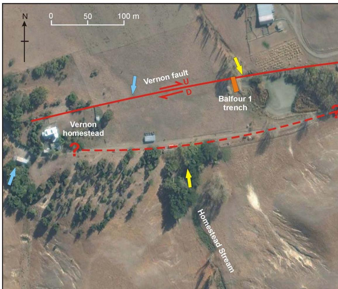
Figure 5 Satellite image of the Balfour 1 trench site. Solid red line shows the well-defined fault scarp, dashed red line shows where an inferred fault is shown in the NZ Active Faults Database. Yellow and blue arrows mark possible offset channels, both of these channels flow from south to north. Image from Google Earth (August, 2011).
