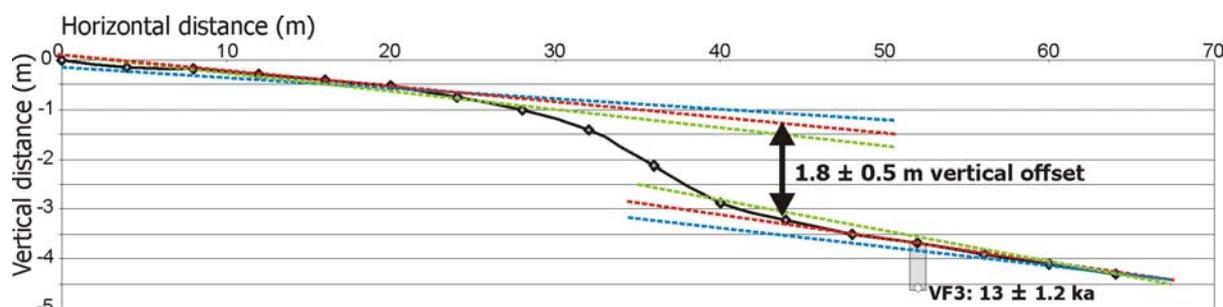
Figure 4 Topographic profile across the Vernon fault scarp at the entrance to Vernon Station. The scarp is approximately 20 m wide. The red line shows the preferred measurement of the vertical offset (1.8 m), the blue and green lines shows the minimum and maximum amounts of vertical offset that could be interpreted from the projections of the offset fan surface across the scarp. The different possible interpretations result in an uncertainty of  $\pm 0.5$  m.
