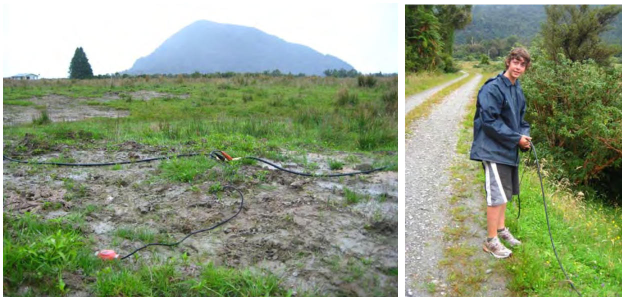
Figure 2. Left: an example of a 40 Hz geophone planted and ready for recording. The geophone is connected to 48 channel line cables by way of alligator clips. Right: field assistant Christopher Pooley laying out the line cable along Turnbull Road.
