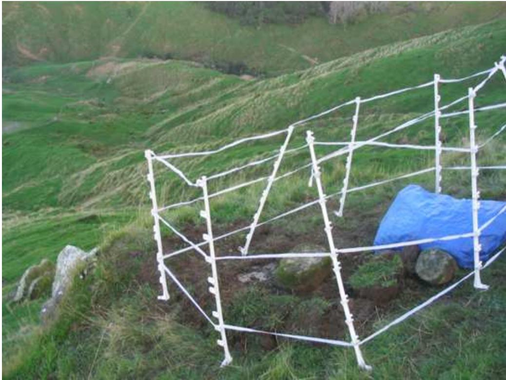
**Figure 3.6: A photograph of the temporary seismic site at Mahia (MHGZ).** A temporary seismic site from the 2006 deployment. The short period sensor is placed in the ground and the seismograph and battery are on top of the ground and covered by a tarpaulin.
