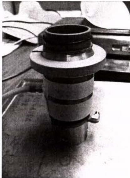
Figure 15 – Mould setup ready for sand placement.
