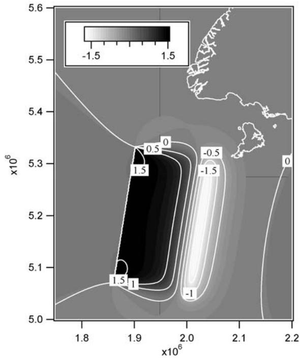
**Figure 25** Vertical displacement (in m) from a  $M_w$  8.6 Puysegur subduction zone earthquake that ruptures the length of the subduction zone to the surface.
