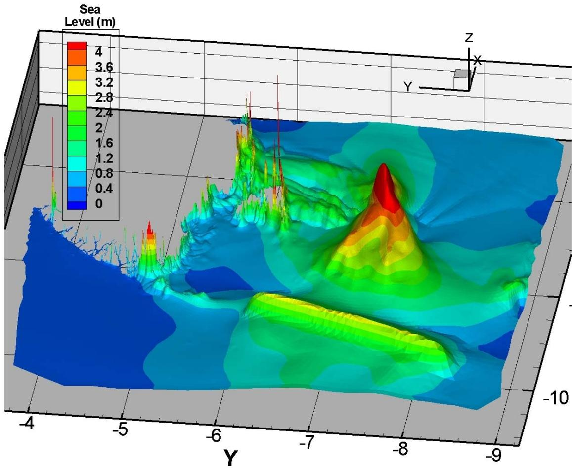
**Figure 36** The envelope of maximum water levels during the Puysegur subduction zone earthquake with no surface rupture scenario.
