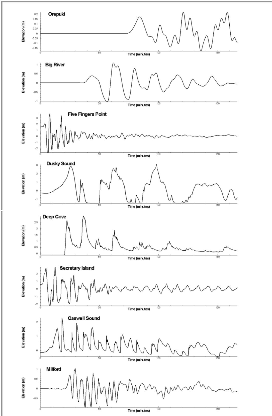
**Figure 31** Time-series of water-surface elevation following the Fiordland subduction zone earthquake with surface rupture scenario. The locations are shown in Figure 27.
