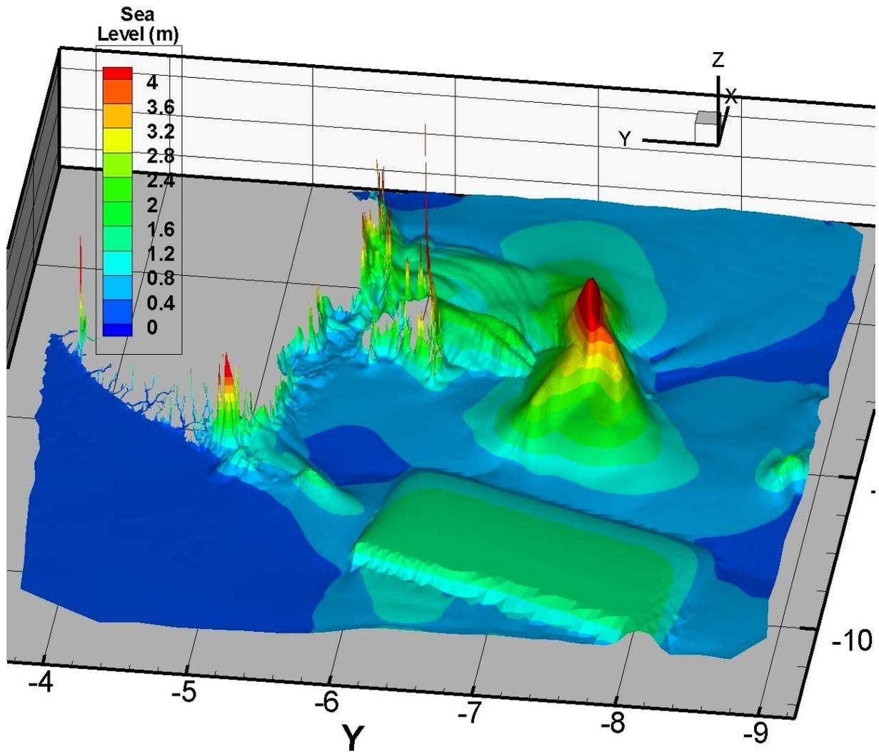
**Figure 34** Envelope of maximum water levels during the Puysegur subduction zone earthquake with surface rupture scenario.
