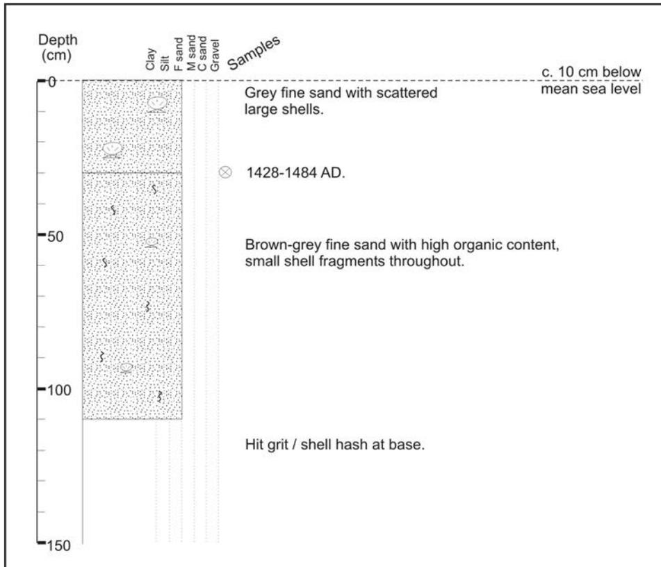
**Figure 21** Stratigraphic log of Auger 3 in Goose Cove tidal inlet.
