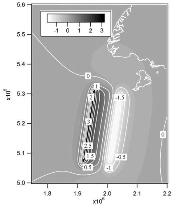
**Figure 26** Vertical displacement (in m) from a  $M_w$  8.5 Puysegur subduction zone earthquake that ruptures the length of the subduction zone without reaching the surface.
