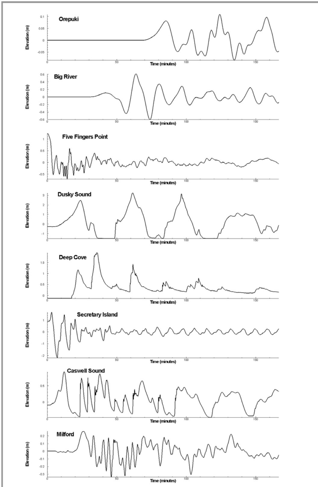
**Figure 33** Time-series of water-surface elevation following the Fiordland subduction zone earthquake with no surface rupture scenario. The locations are shown in Figure 27.
