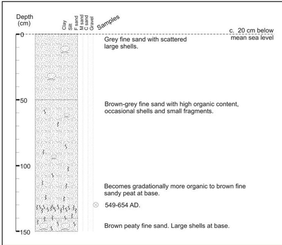
**Figure 20** Stratigraphic log of Auger 2 in Goose Cove tidal inlet.
