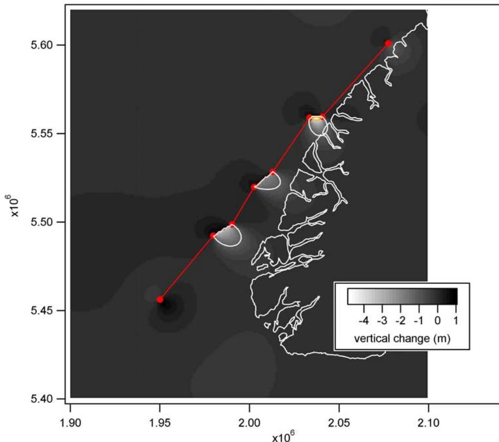
**Figure 22** Vertical displacements (in m) from an  $M_w$  7.8 Alpine Fault earthquake with rupture along several fault segments. Note the contour shown represents 1 m of subsidence, and the subsidence zone encircled by the 1 m contour ranges from 1 – 4.5 m.
