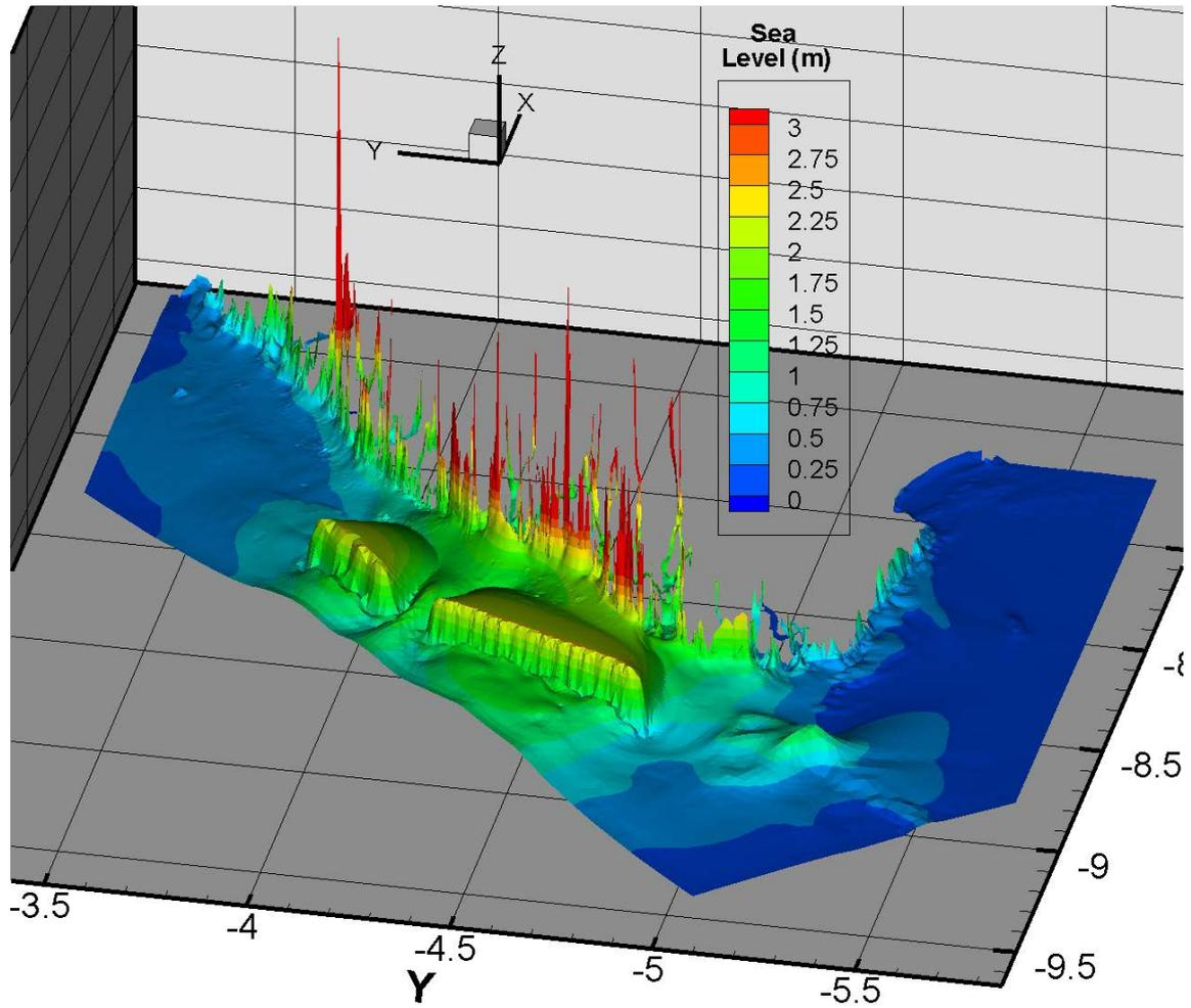
**Figure 30** The envelope of maximum water levels during the Fjordland subduction zone earthquake with surface rupture scenario.
