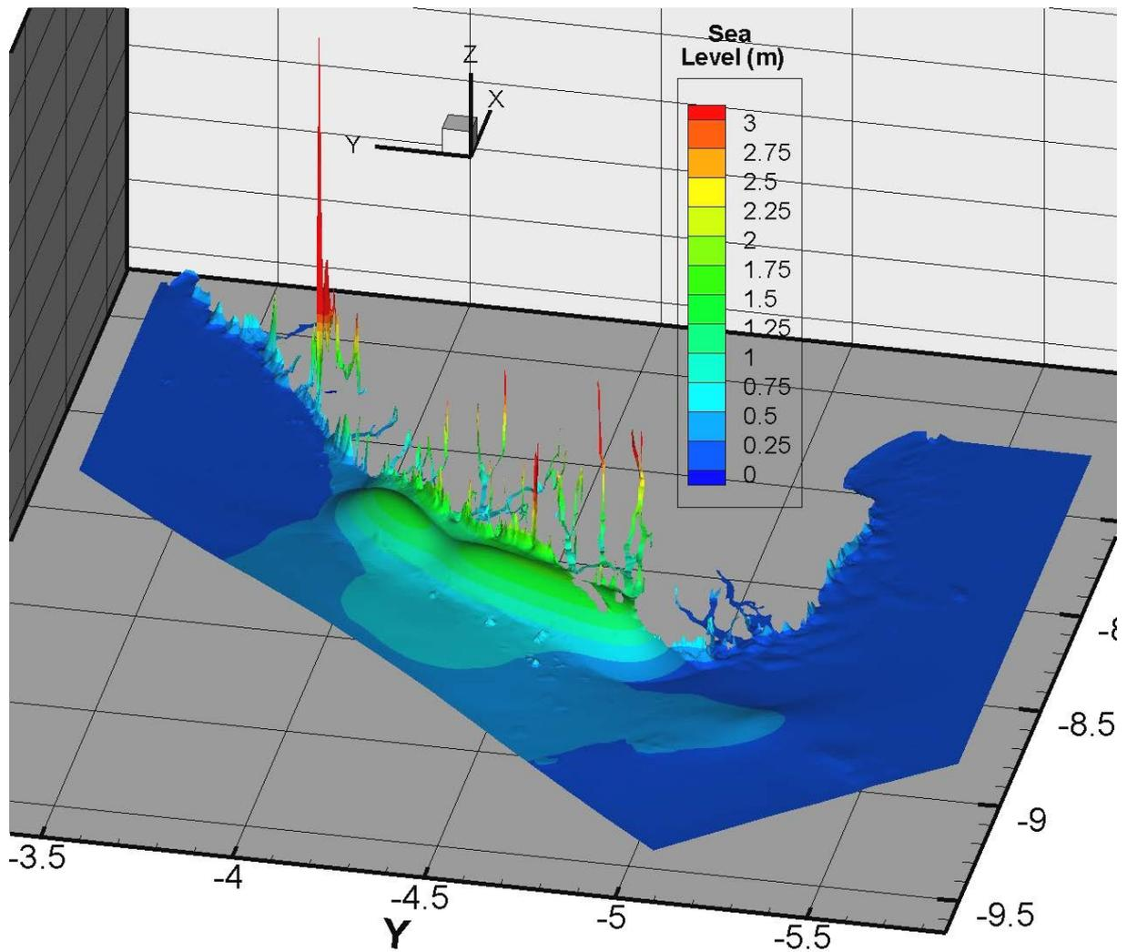
**Figure 32** Envelope of maximum water levels during the Fjordland subduction zone earthquake with no surface rupture scenario.
