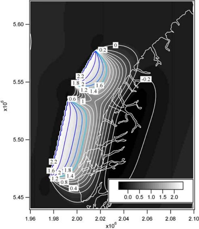
**Figure 23** Vertical displacement (in m) from an  $M_w$  7.9 Fiordland subduction zone earthquake that ruptures a large part of the subduction zone to the surface.
