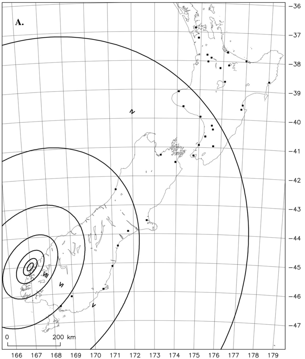
**Figure 38** Expected intensities from A. an  $M_w$  7.8 on the offshore Alpine Fault; B. an  $M_w$  7.9 on the Fjordland subduction zone; C. an  $M_w$  8.6 earthquake on the Puysegur subduction zone.
