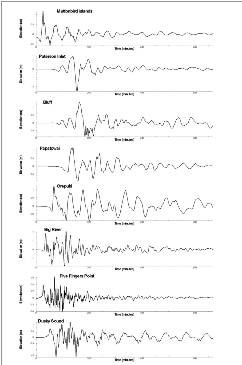
**Figure 37** Time-series of water-surface elevation following the Puysegur subduction zone event with no surface rupture. The locations are shown in Figure 27.
