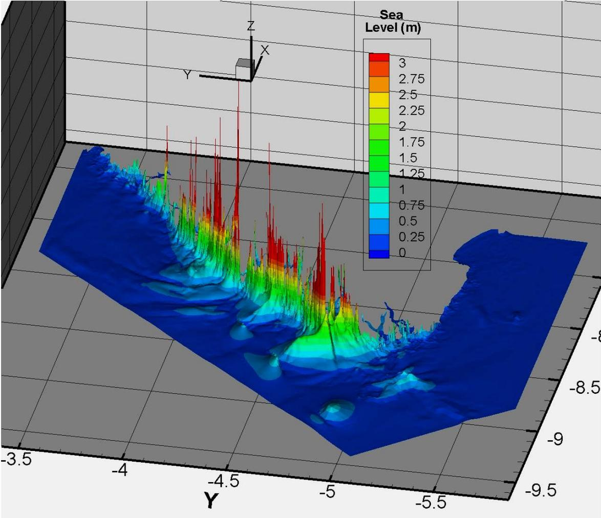
**Figure 28** Envelope of maximum water levels during the Alpine Fault earthquake scenario.
