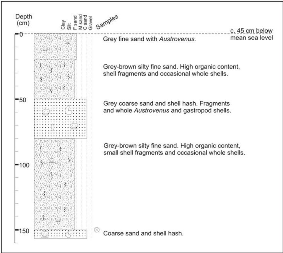
**Figure 19** Stratigraphic log of Auger 1 in Goose Cove tidal inlet.
