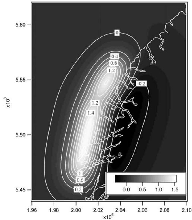
**Figure 24** Vertical displacement (in m) from an  $M_w$ 7.7 Fiordland subduction zone earthquake that ruptures a large part of the subduction zone without reaching the surface.
