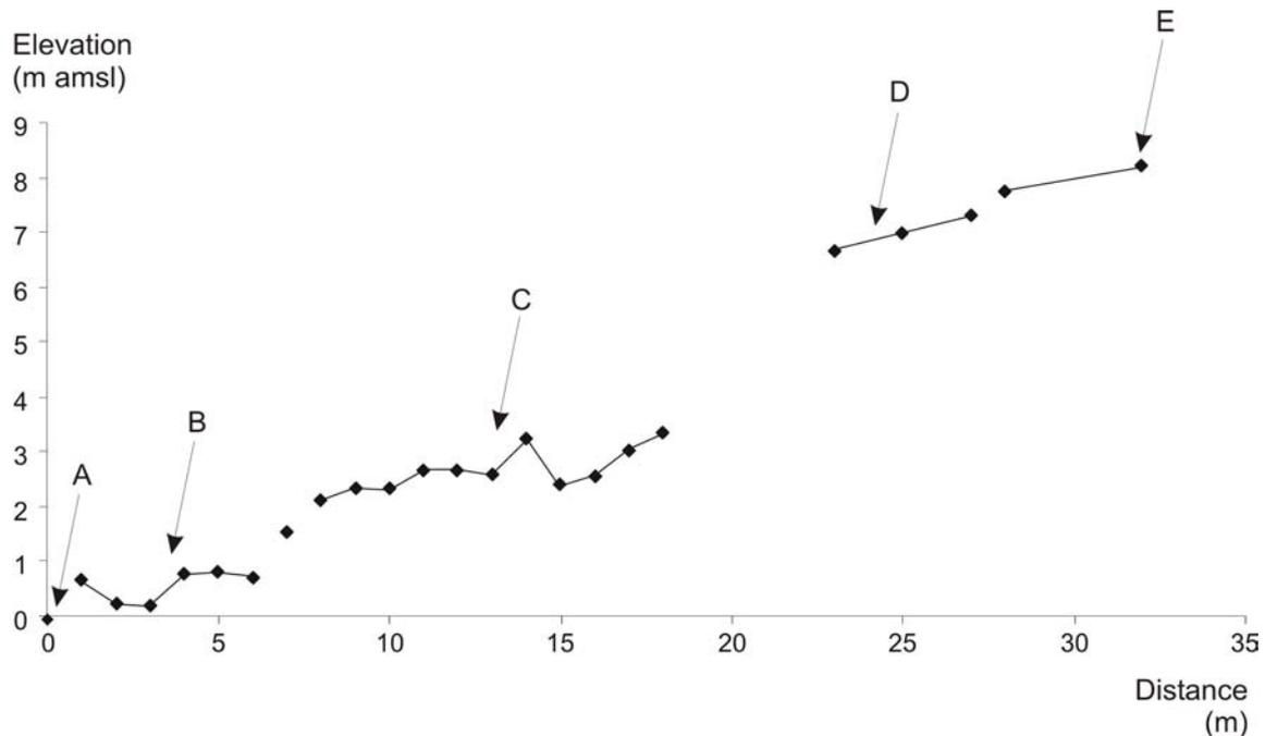
**Figure 14** Profile across the stepped bedrock platforms at the approximate position of the solid lines in Figure 13. This profile was measured from a known tide position using a dumpy level. Platform elevations are reasonably consistent with the topography measured by RTK-GPS as shown in Figure 13.
