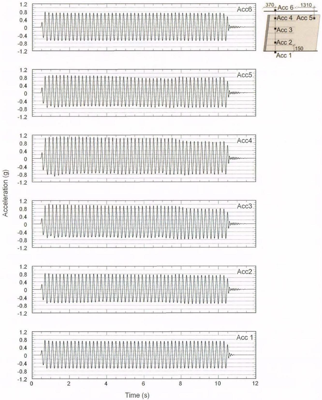
Figure B-73. Test-7 acceleration time histories at 0.7g shaking step.
