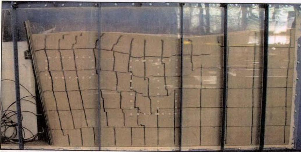
Figure C-18. Test-4 after 0.65g shaking step.
