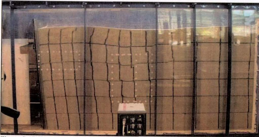
Figure C-17. Test-4 after 0.6g shaking step.
