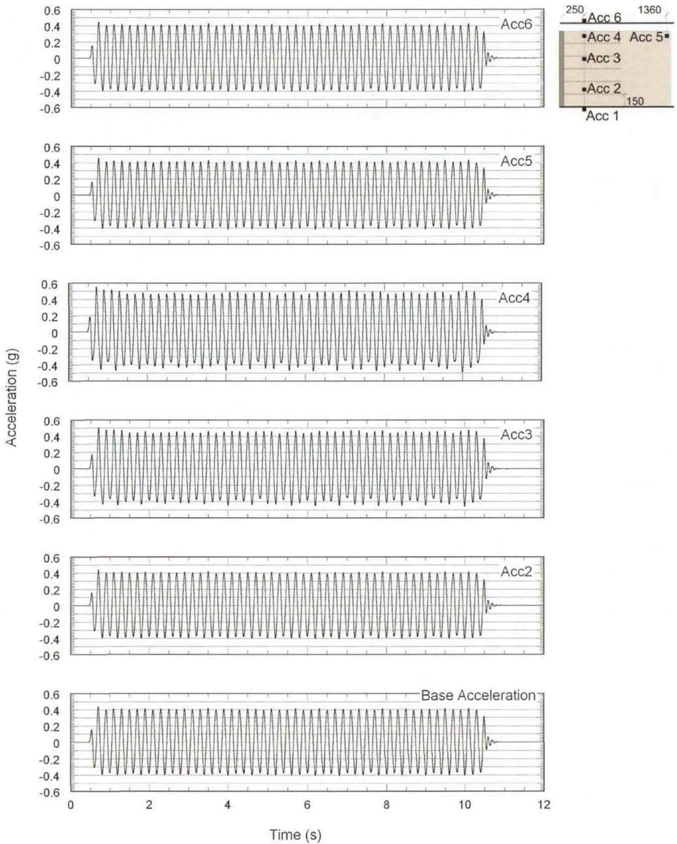
Figure B-46. Test-5 acceleration time histories at 0.4g shaking step.
