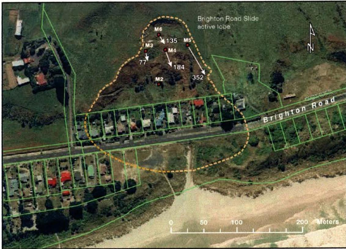
Figure 3.2: The Brighton Road Slide with survey marks and horizontal displacement in mm shown as vectors. The graph below summarises the displacement a Brighton Road Slide 1998 – 2001.
