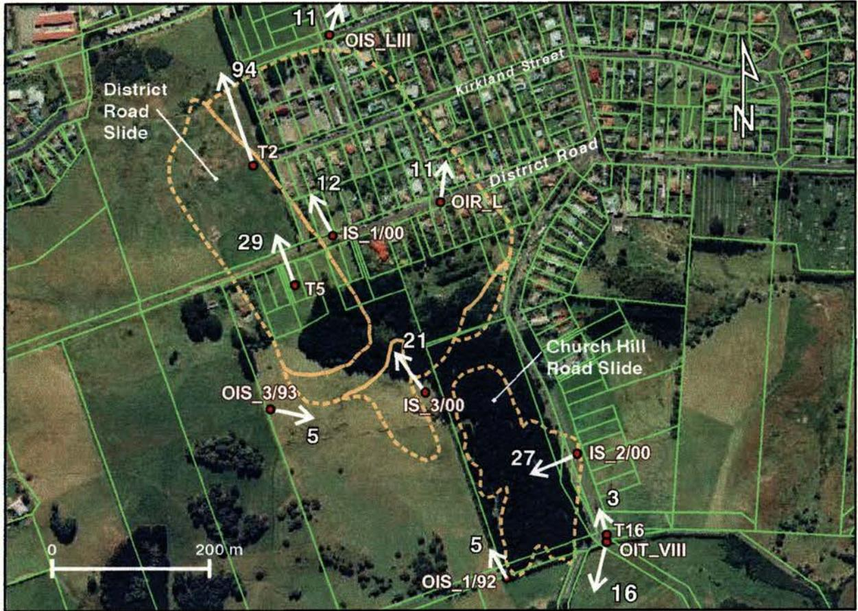
**Figure 3.4:** The Church Hill Rd and District Rd slides, Green Island, with survey marks showing horizontal displacement vectors (mm) for rationalised survey points. The total horizontal and vertical displacements are given in the graphs below (overleaf).
