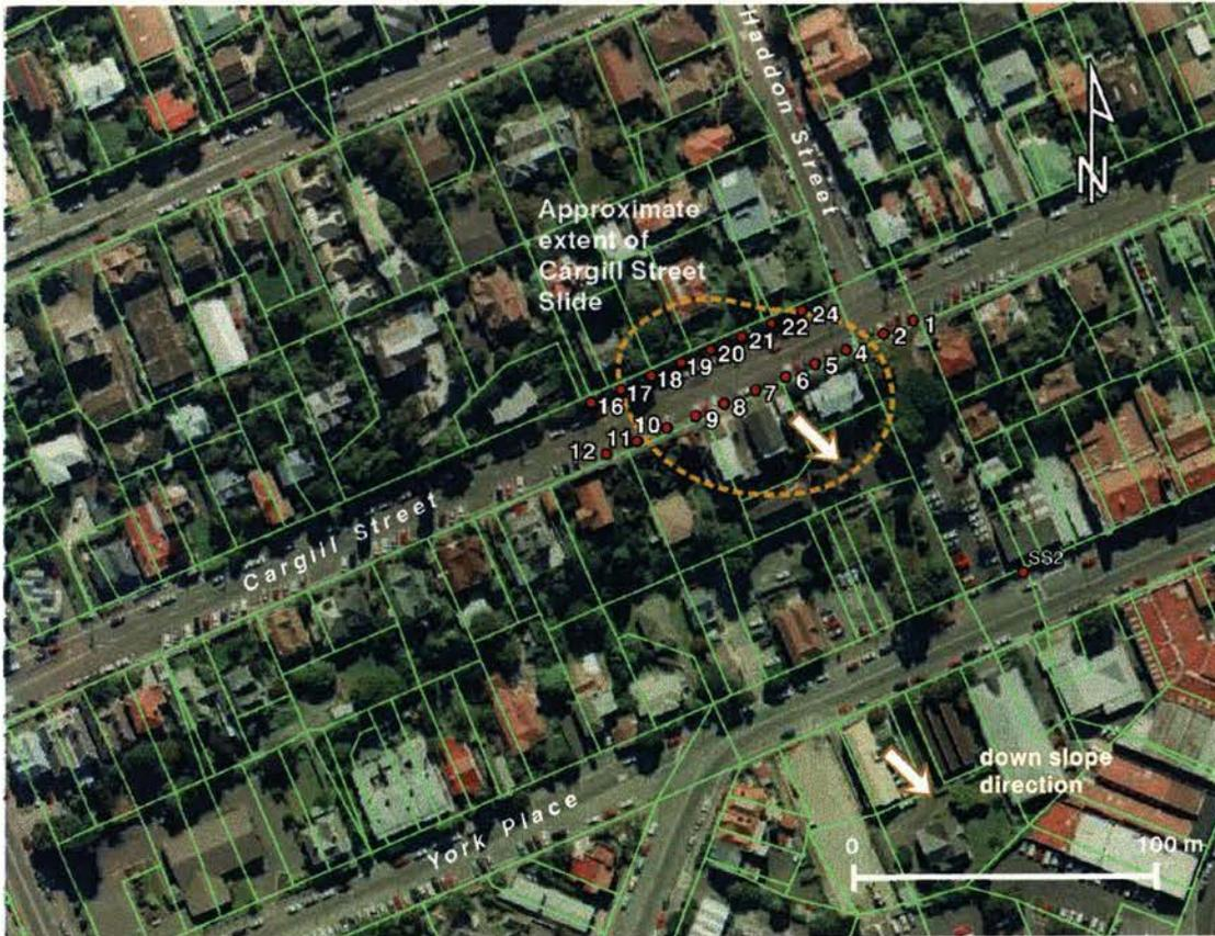
**Figure 3.3:** Approximate extent of the Cargill St Slide, Central Dunedin. The survey marks are shown. Only levels and offset, either downslope (-) or upslope (+), were recorded. The graph below summarises the displacement recorded at survey marks 1987 to 1988
