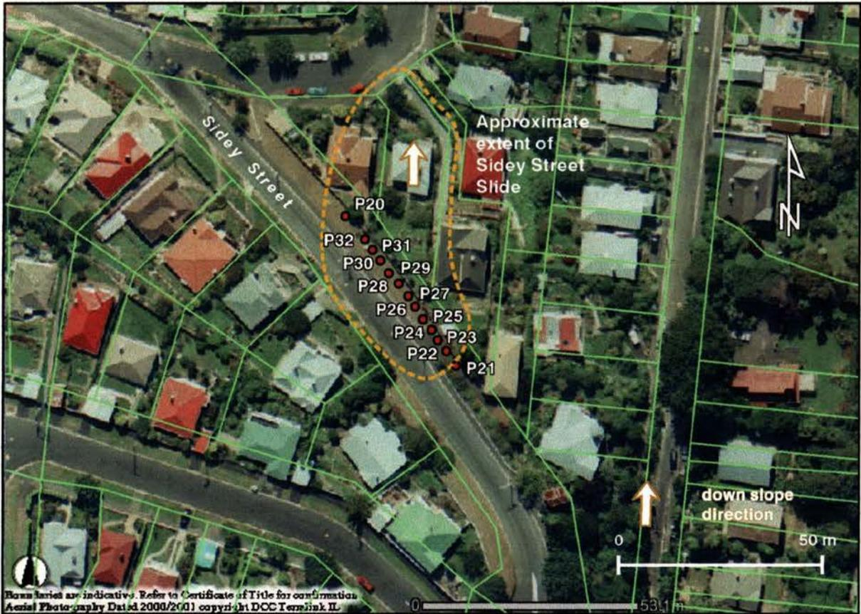
**Figure 3.8:** Approximate extent of the Sidey Street slide with the monitoring pins indicated. The vectors of horizontal movement are not shown as they were measured a downslope (-) or upslope (+) movement from a baseline bearing. Total horizontal and vertical deformation (mm) of survey marks at the Sidey Street slide 1997 – 2000 are given on the graph below.
