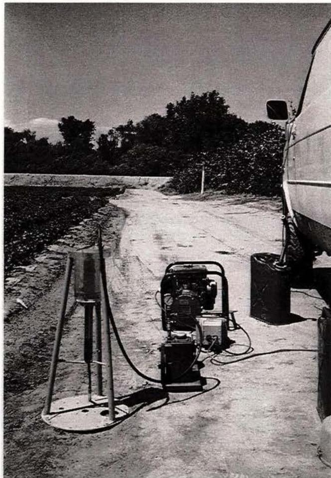
**Figure 3.2** Piezocone de-airing in progress (Miller's Farm, Test 7)
