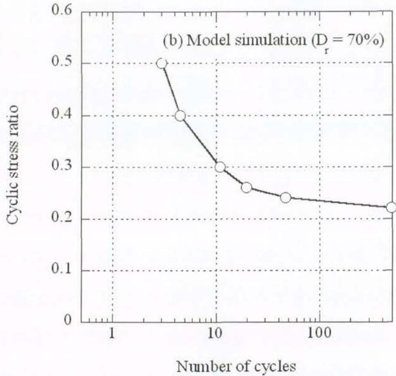
Figure 47. Liquefaction resistance of Albany sand adopted in the simulations (NIED 2006)
