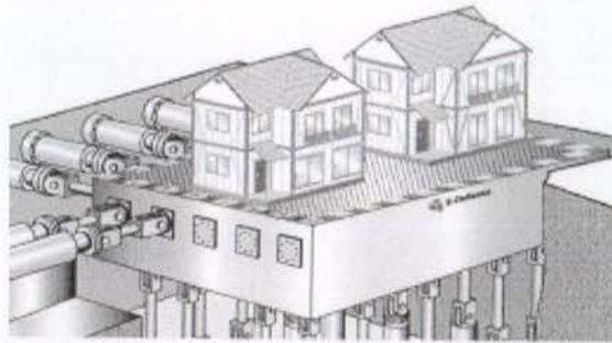
Figure 14. Schematic view of Japanese-style wooden houses on the shake table (Sato and Inoue 2004)
