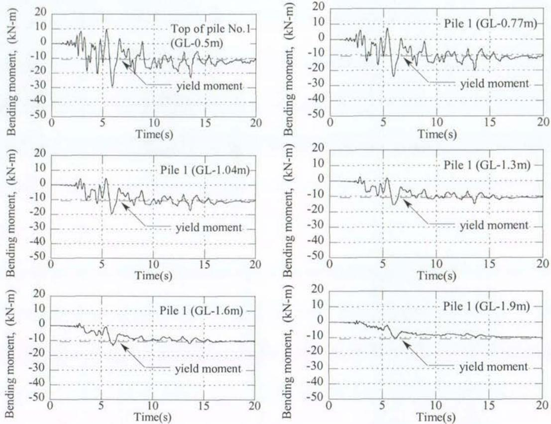
Figure 59. Computed bending moments for pile 1 in the analysis using elastic piles (NIED 2006)
