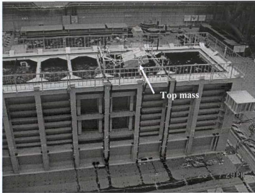
Figure 43. Full-scale experimental model during the shaking
