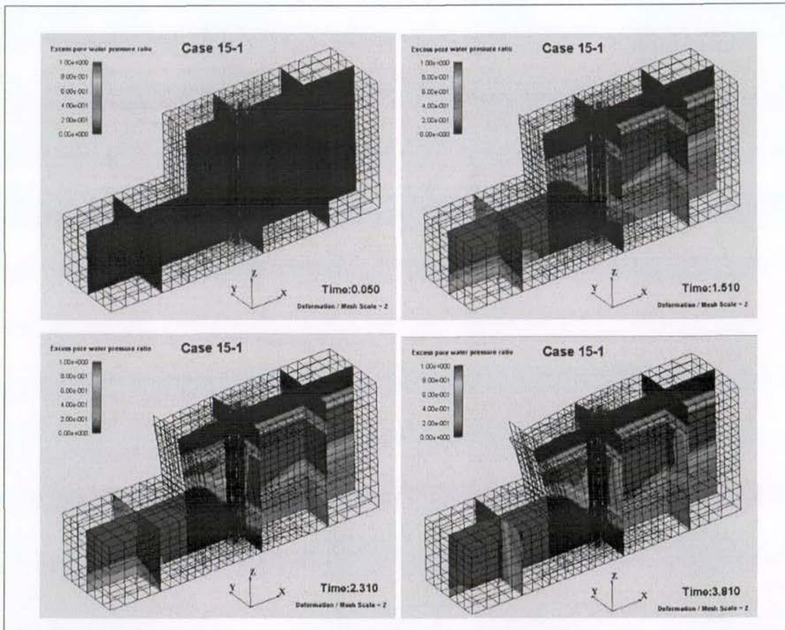
Figure 22. Development of excess pore water pressure (NIED 2004)
