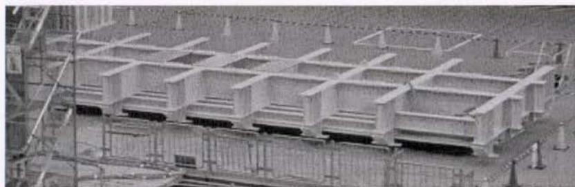
Figure 41. Steel frame on rollers used to transport experimental model
