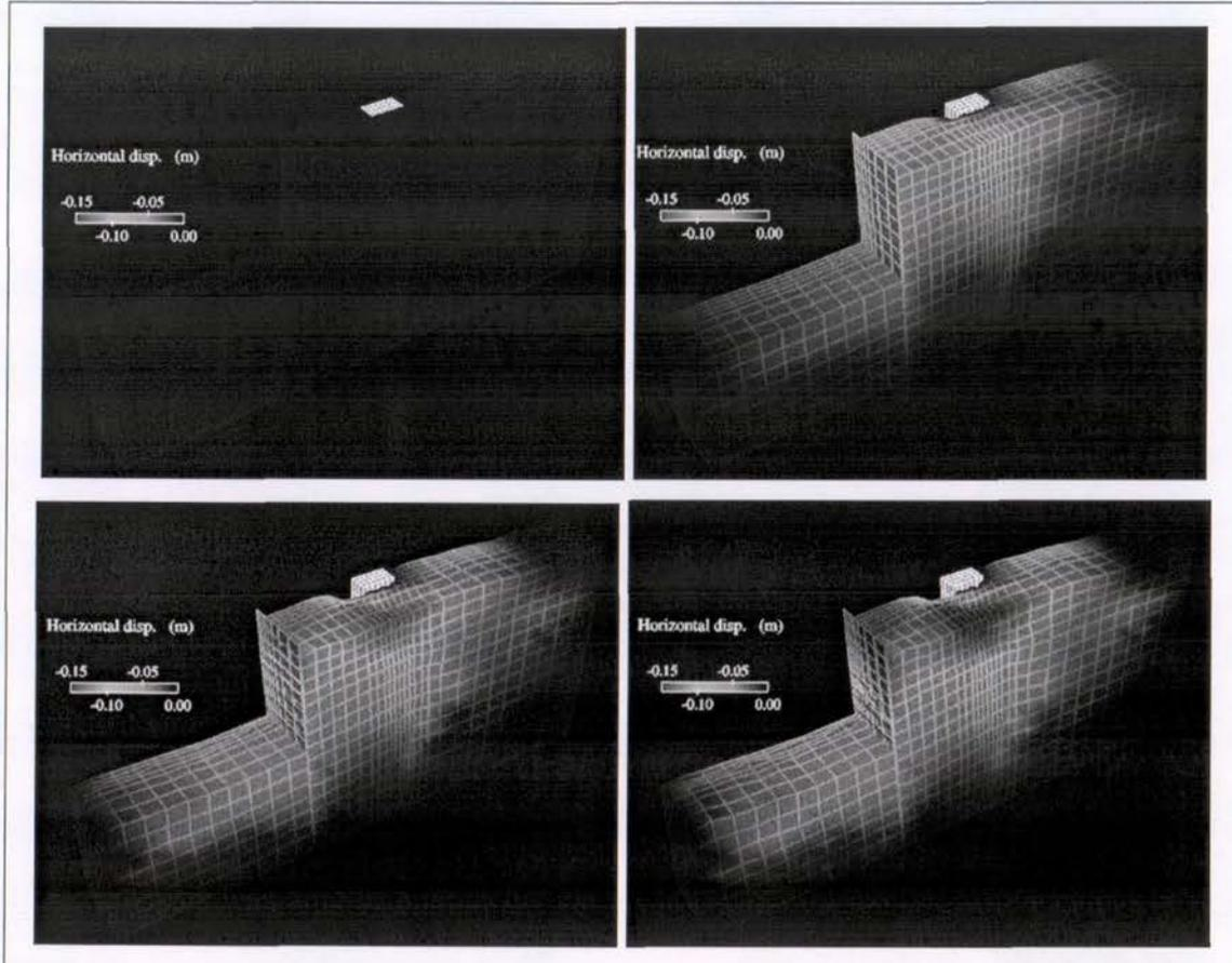
Figure 21. Computed horizontal ground displacement (NIED 2004)
