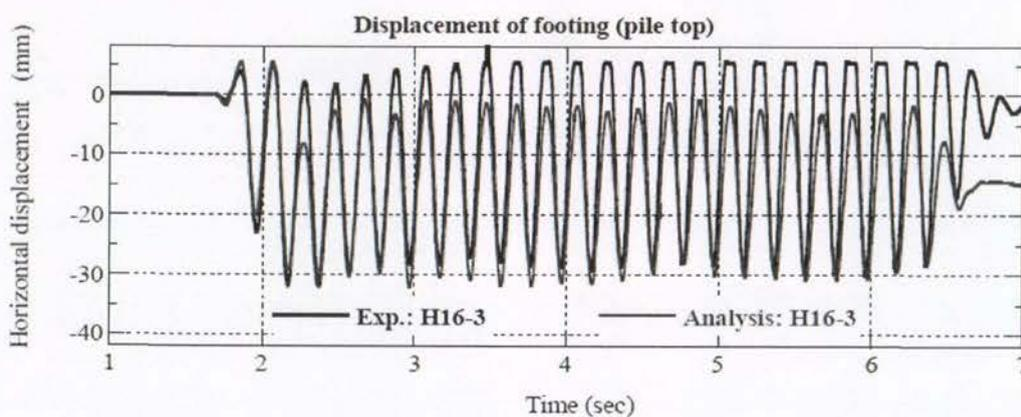
Figure 25. Comparison of computed and recorded displacement of the footing in Experiment 16-3 (NIED 2004)
