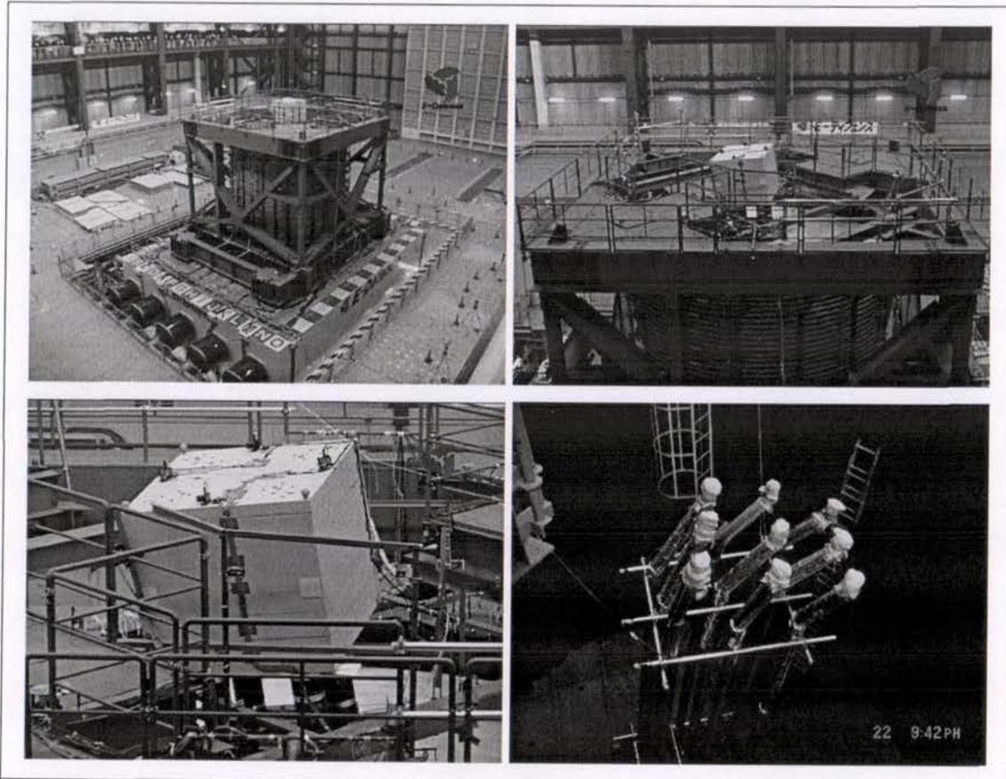
Figure 34. Model of piles undergoing cyclic shaking, (a) before shaking, (b) during shaking, (c) after shaking, (d) after soil has been removed (NIED (website) 2006)
