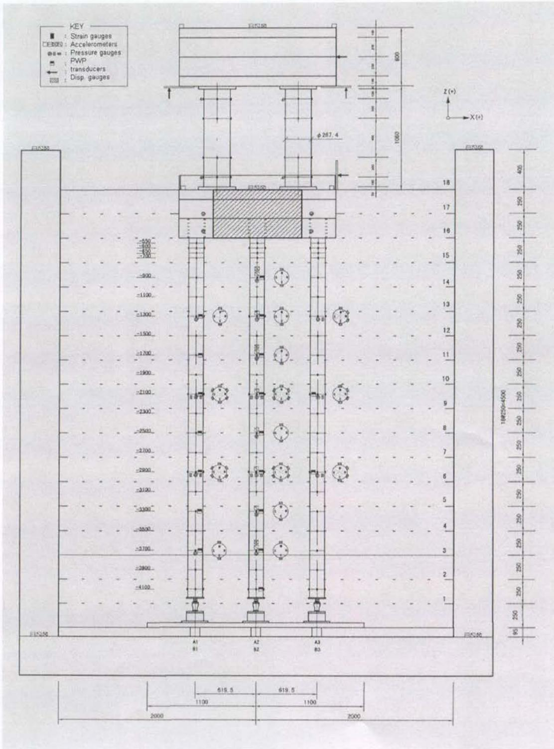
Figure 38. Instrumentation layout on the piles
