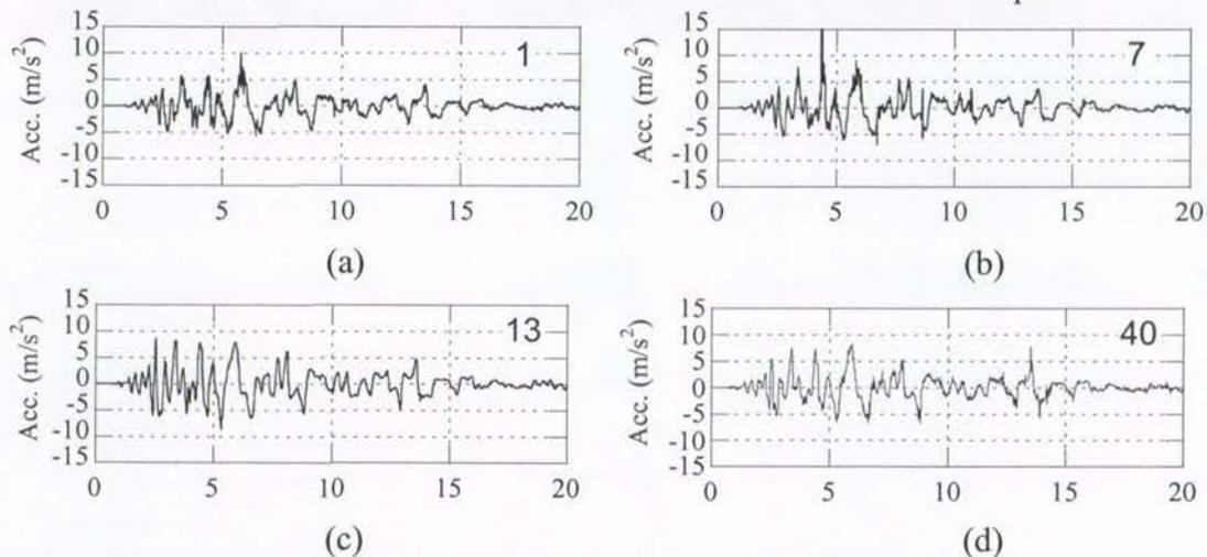
Figure 56. Computed horizontal accelerations at the top of the ground model; (a,b) submerged soil; (c) near the sheet pile wall, and (d) free field response (NIED 2006)
