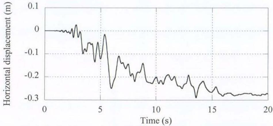
Figure 57. Computed horizontal displacement of the sheet-pile wall in the analysis with elastic piles (NIED 2006)
