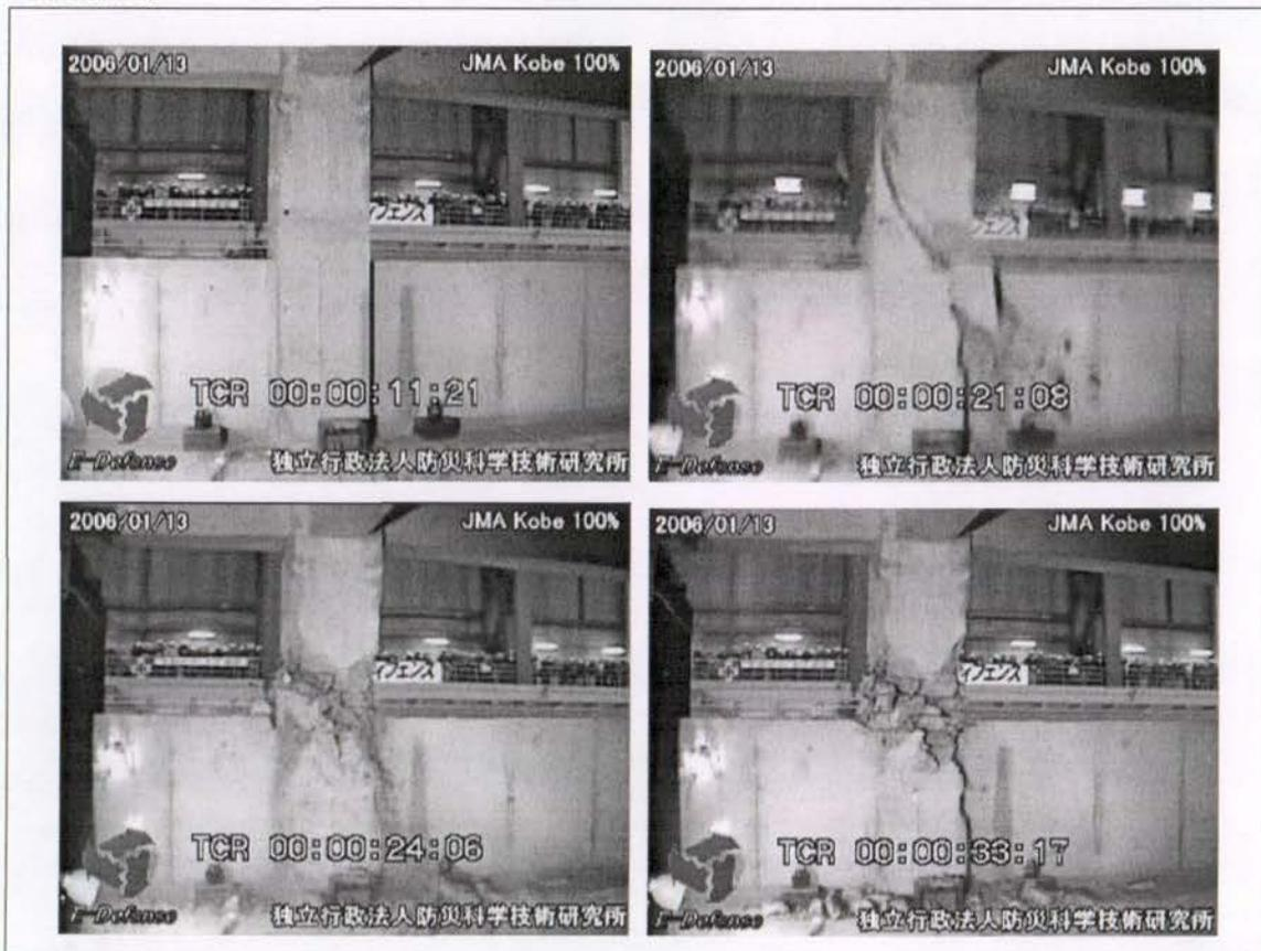
Figure 30. Failure of ground floor columns of RC building (NIED (website) 2006)
