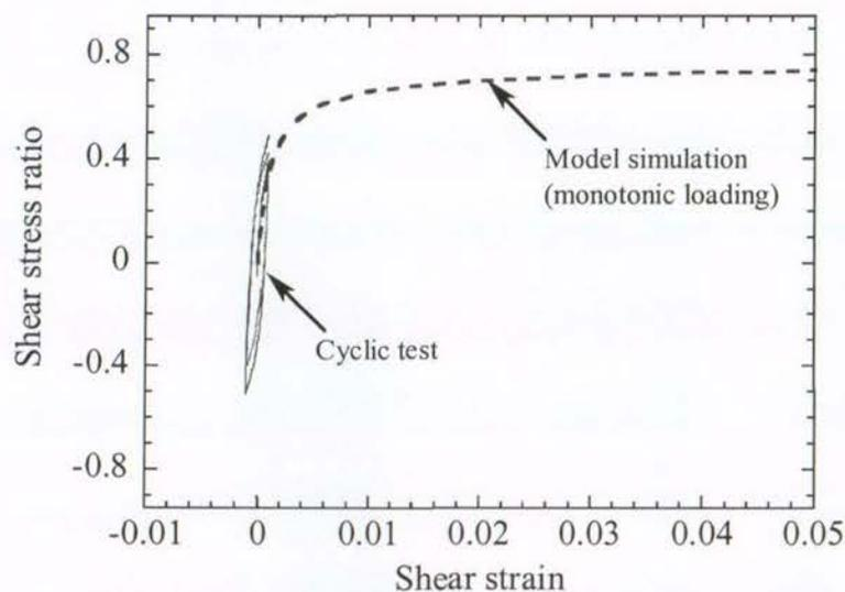
Figure 49. Drained cyclic tests on Albany sand (Uzuoka et al., 2006) and model simulation of monotonic loading behaviour (NIED 2006)
