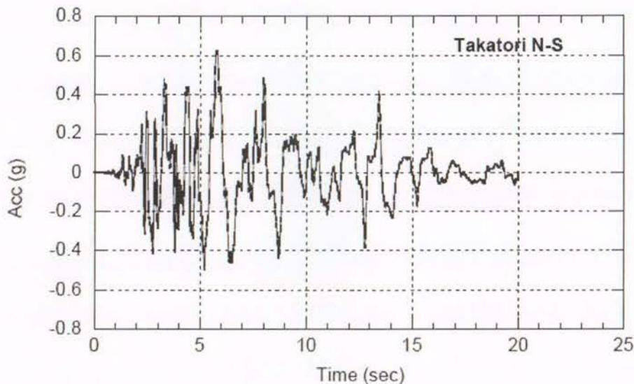
Figure 42. Takatori N-S accelerogram used a input motion in the analysis (NIED 2006)
