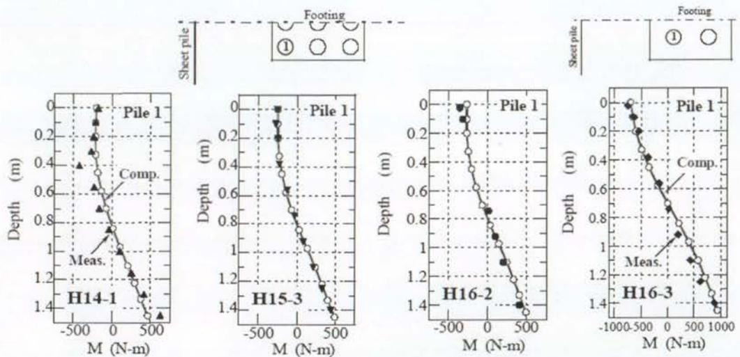
Figure 26. Comparison of computed and recorded bending moments along Pile 1 (NIED 2004)
