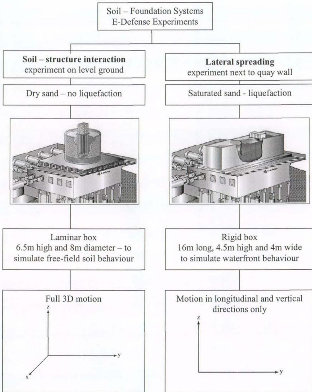
Figure 32. E-Defense experiments on soils and foundations
