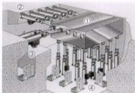
Figure 11. Schematic of shake table and actuators (NIED (website) 2006)
