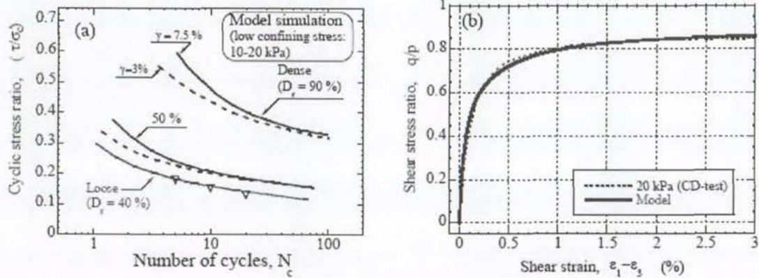
Figure 19. Model simulation of test soils: (a) Liquefaction resistance of Toyoura sand at  $D_r = 40\%$ ,  $50\%$  and  $90\%$ ; (b) Monotonic stress-strain curve of coarse sand crust layer (NIED 2004)
