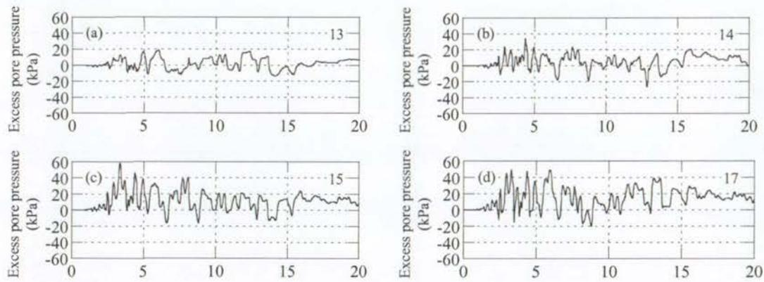
Figure 55. Computed excess pore water pressures in the soil behind the sheet-pile wall (NIED 2006)
