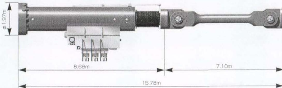
Figure 10. Actuator schematic and dimensions (NIED (website) 2006)
