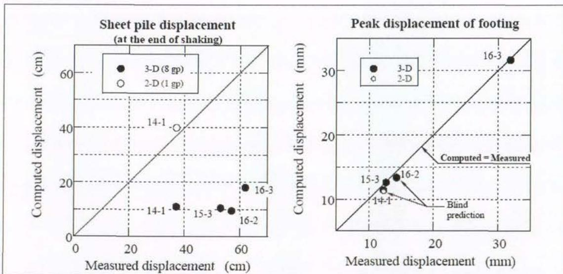
Figure 24. Comparison of computed and measured: (a) final sheet pile displacements; (b) peak footing displacements (NIED 2004)
