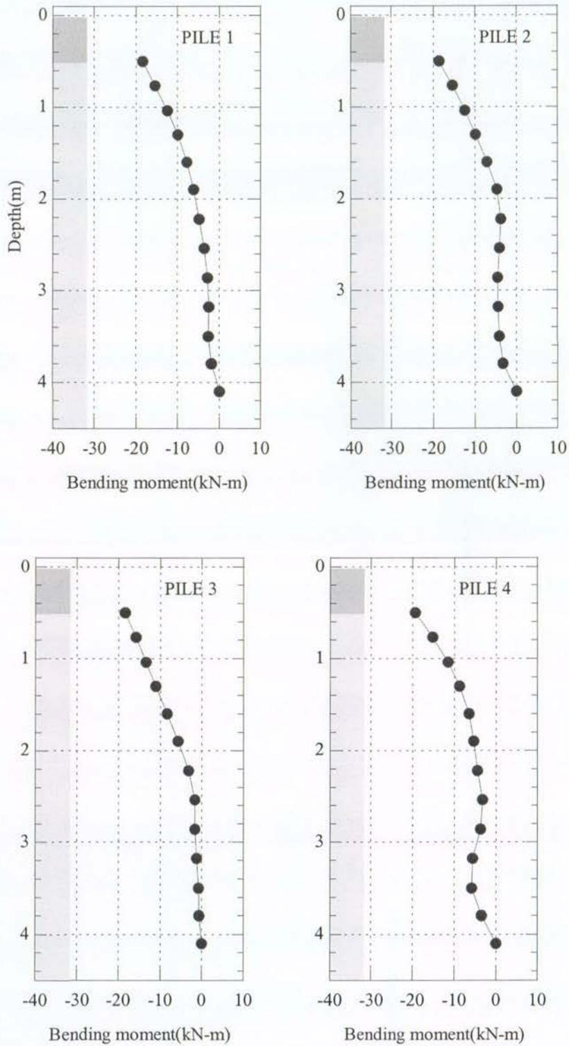
Figure 60. Computed distribution of bending moments for piles 1-4 in the analysis using elastic piles ( $t = 5.76$  sec) (NIED 2006)
