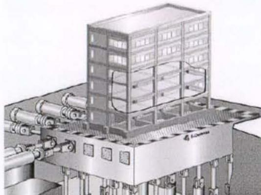
Figure 15. Schematic view of the reinforced concrete building on the shake table (Sato and Inoue 2004)
