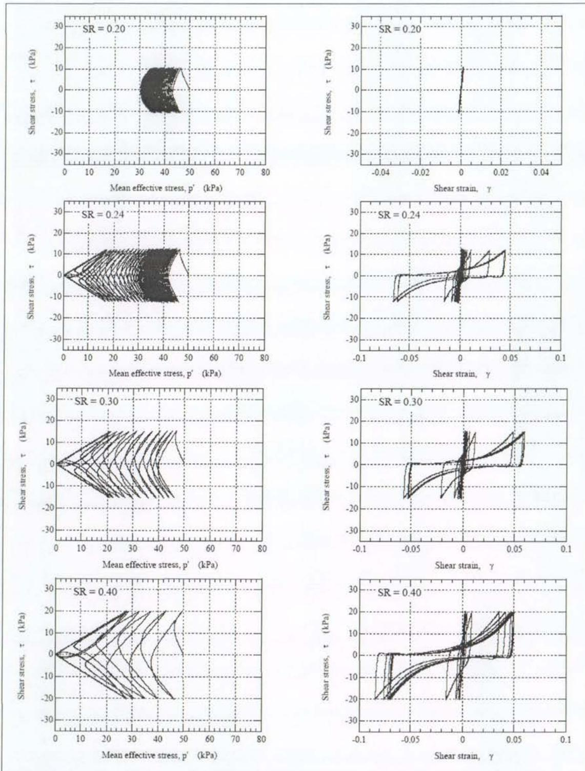
Figure 48. Cyclic behaviour of Albany sand simulated with the model (NIED 2006)
