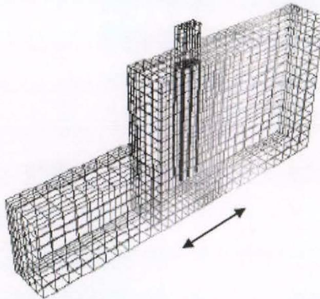
Figure 20. Numerical model used in the 3D analyses (NIED 2004)
