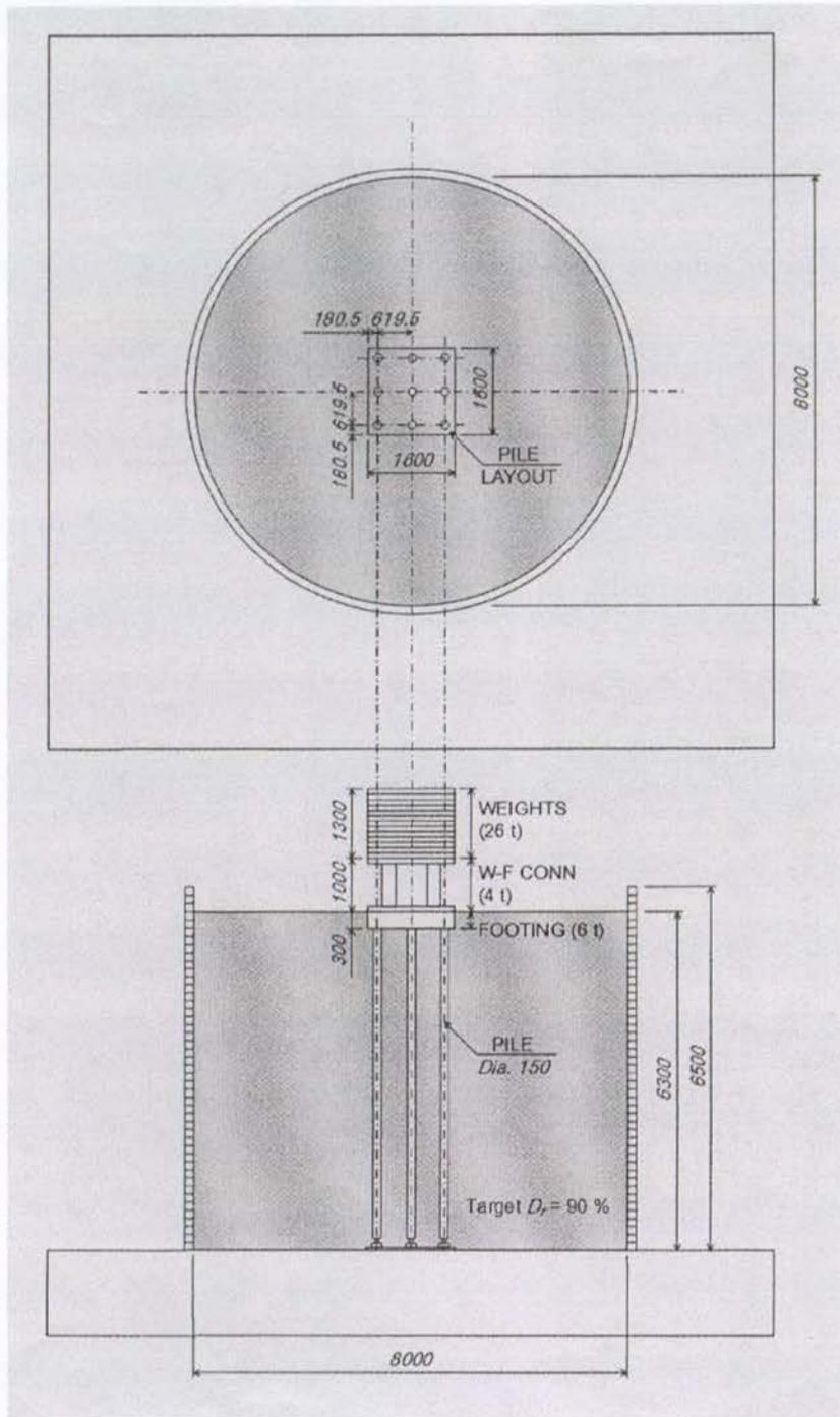
Figure 33. Experimental set-up of E-Defense soil-structure interaction model
