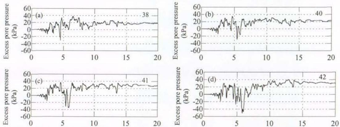
Figure 53. Computed excess pore water pressures in the backfill at a distance approximately 4m from the pile foundation (NIED 2006)
