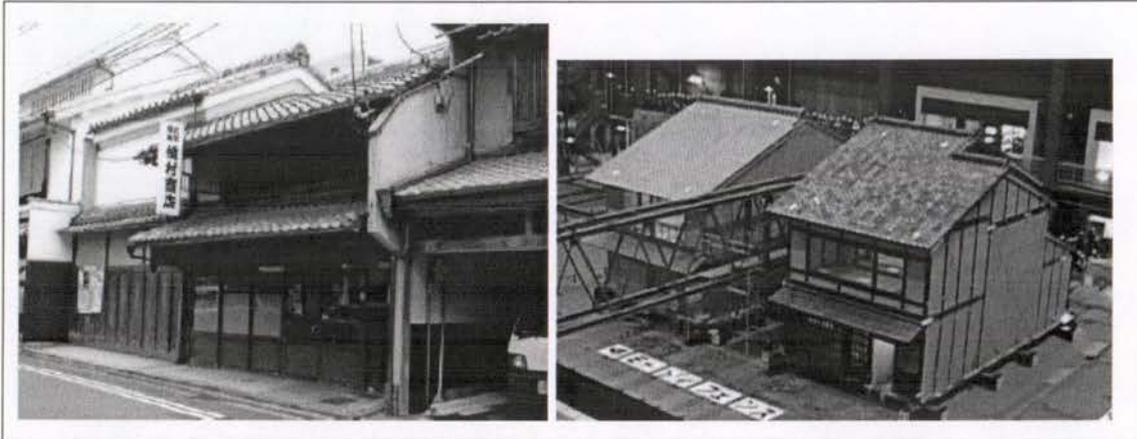
Figure 27. Conventional wooden residential buildings; (a) photo of actual building, (b) photo of building on the shake table (NIED (website) 2006)
