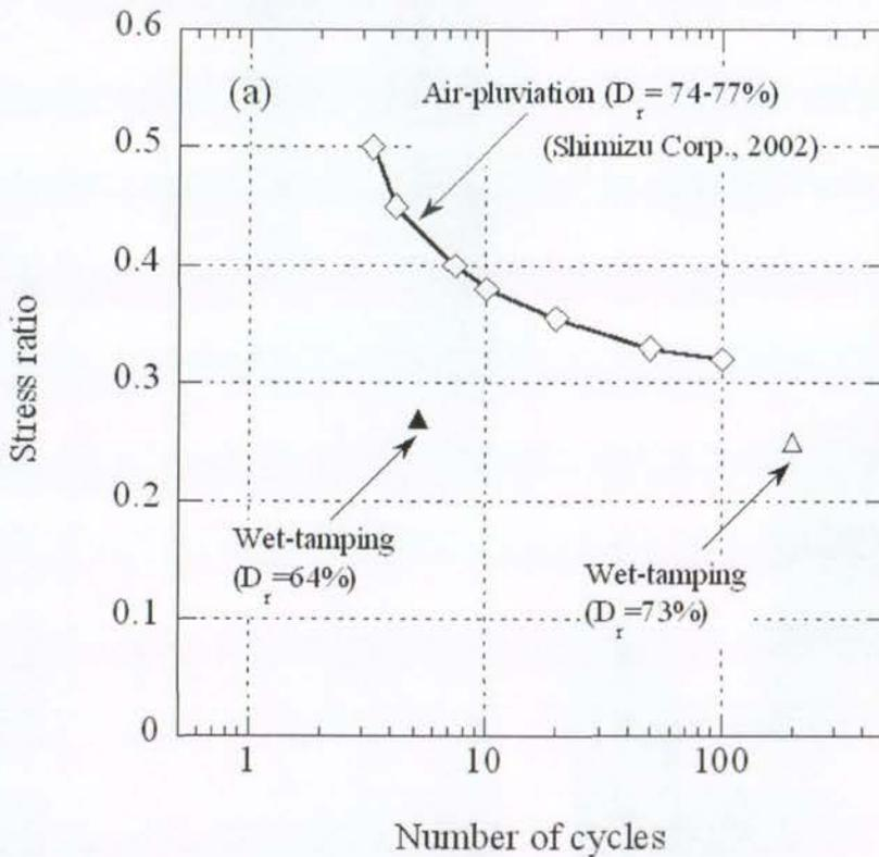
Figure 46. Liquefaction resistance of Albany sand from results of cyclic triaxial tests (NIED 2006)
