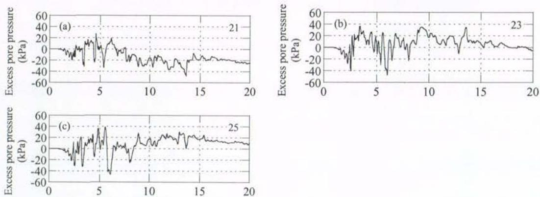
Figure 54. Computed excess pore water pressures in the soil in the vicinity of the piles (NIED 2006)
