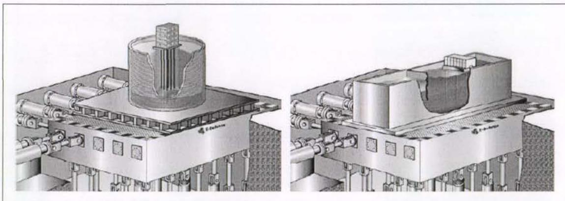
Figure 16. Schematic showing experiments of piles in soil undergoing (a) cyclic shaking and (b) lateral spreading (Sato and Inoue 2004)
