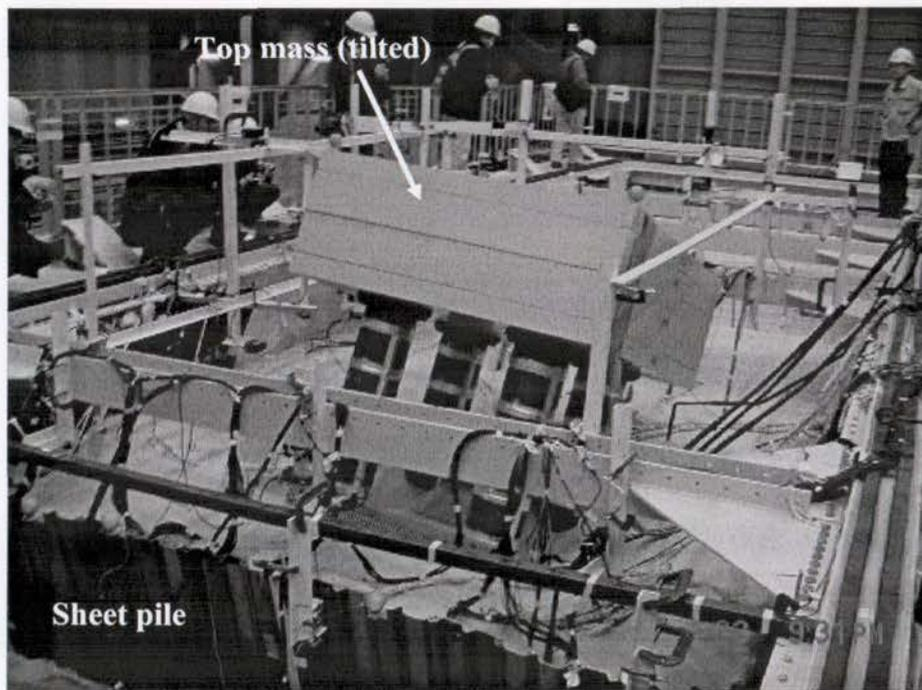
Figure 44. Full-scale experimental model after the shaking
