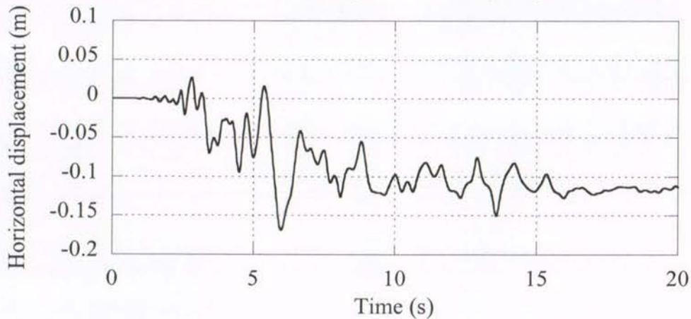
Figure 58. Computed horizontal displacement of the footing (pile cap) in the analysis with elastic piles (NIED 2006)
