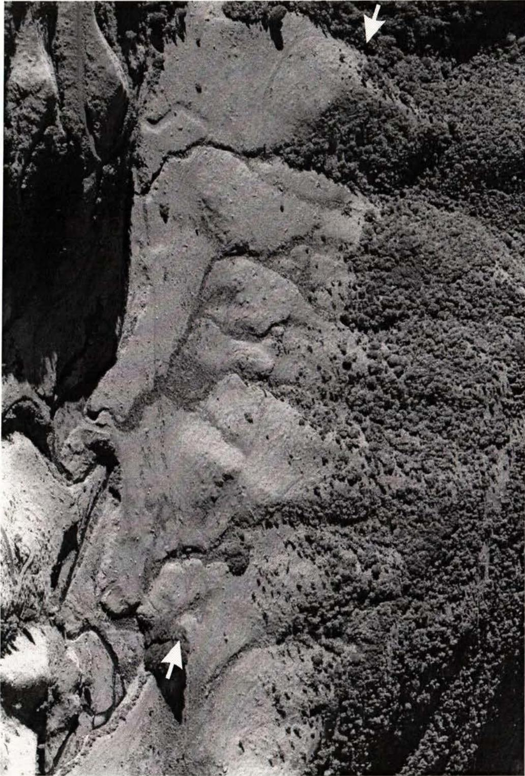
**Fig. 15.** Aerial photograph looking east-southeast across uphill-facing, bedrock scarp of the Northern Ohariu fault, Makahika Stream area (grid ref. S25 135 614). Bold arrows show the fault's location. Makahika Stream winds its way left to right across the bottom of the photo. *Photo: D.L. Homer, Institute of Geological & Nuclear Sciences (photo ref. CN 39624 13).*
