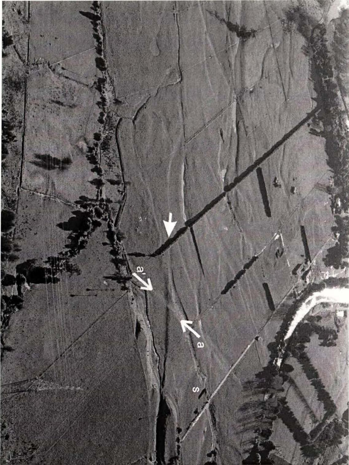
**Fig. 10.** Aerial photograph looking north-northwest across northeast-trending Northern Ohariu fault, Florida Road/Ohau River area. Bold arrows show fault's location. The 3.0-3.5 m net displacement of the young terrace riser is denoted by the arrows labelled a-a', and is interpreted to represent the amount of surface rupture displacement that occurred at this site during the most recent earthquake. "s" is location of silage pit discussed in text.
