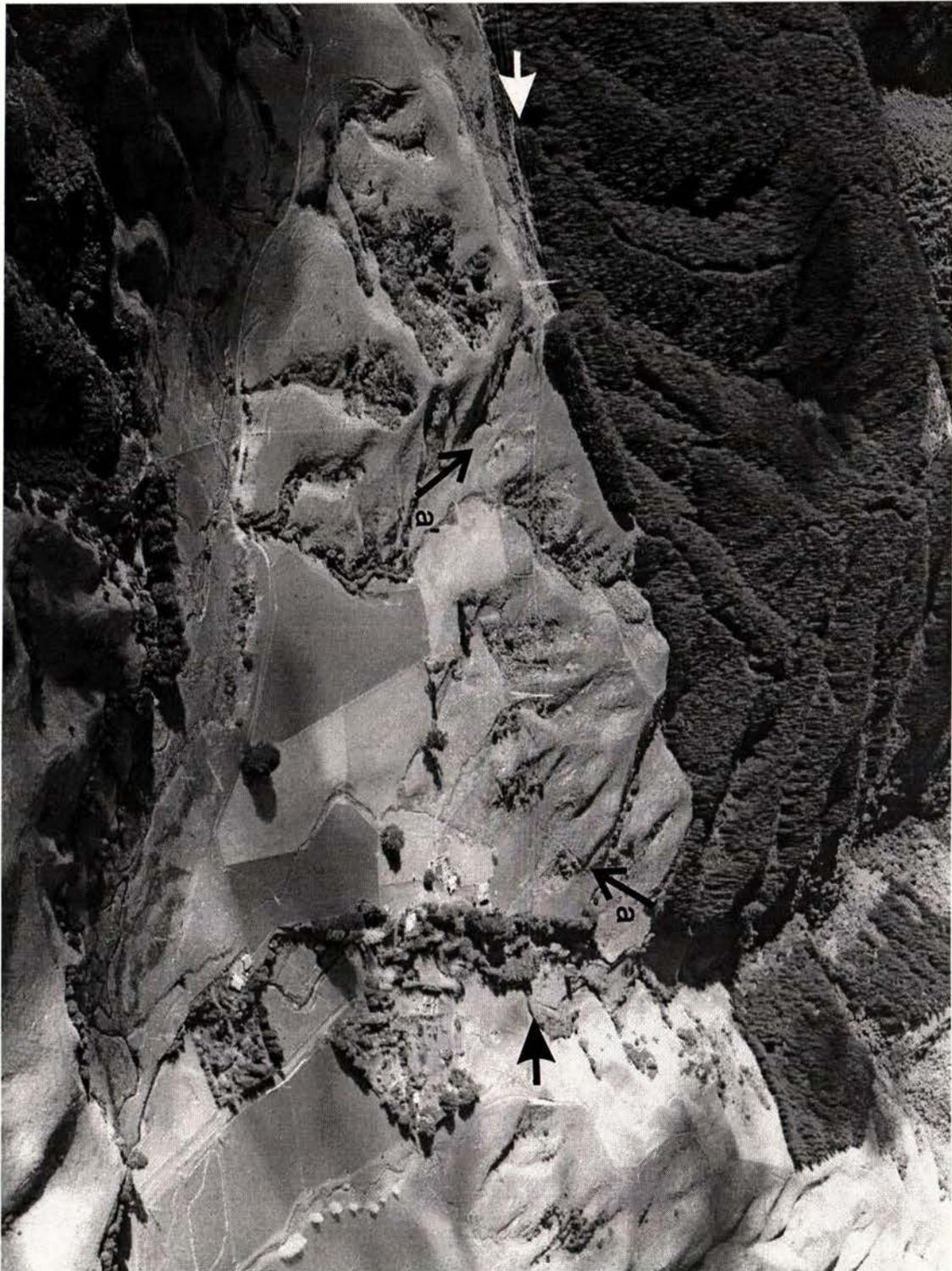
**Fig. 6.** Aerial photograph looking southeast across the northeast-trending Northern Ohariu fault, Corbetts Road area. Bold arrows show the fault's location. The maximum right-lateral offset of ca 450 m is denoted by the arrows labelled a & a', and the prominent loess covered alluvial terrace to the right of a' is probably Marton in age (ca 140 000 years), yielding a maximum right-lateral slip rate at this site of about 3 mm/yr.
