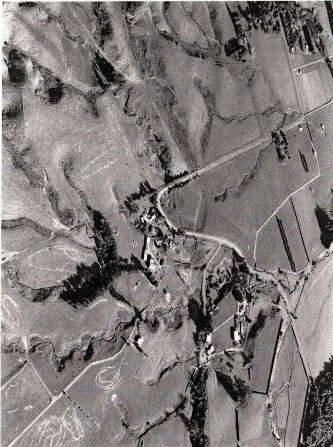
**Fig. 9.** Aerial photograph looking north-northwest across the northeast-trending Northern Ohariu fault (grid ref. S25 050564). Bold arrows show the fault's location. The main road in the photo is Florida Road. The displaced terraces in the photograph are Marton in age and younger (less than ca 140 000 years).
