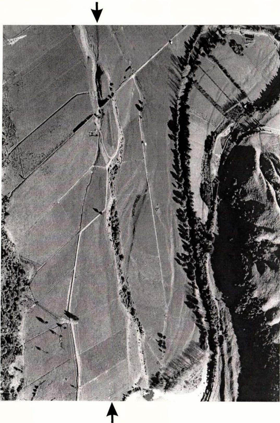
**Fig. 11.** Aerial photograph looking north-northwest across the ENE-trending Northern Ohariu fault (grid ref. S25 073 574). The bold arrows show the location of the fault. The river and road in the upper part of the photo are the Ohau River and Gladstone Road, respectively. The displaced alluvial terraces in the photograph are Ohakean age (10 000-15 000 years old) and younger. The photograph shown in Fig. 10 was taken just to the left (southwest) of this photo.
