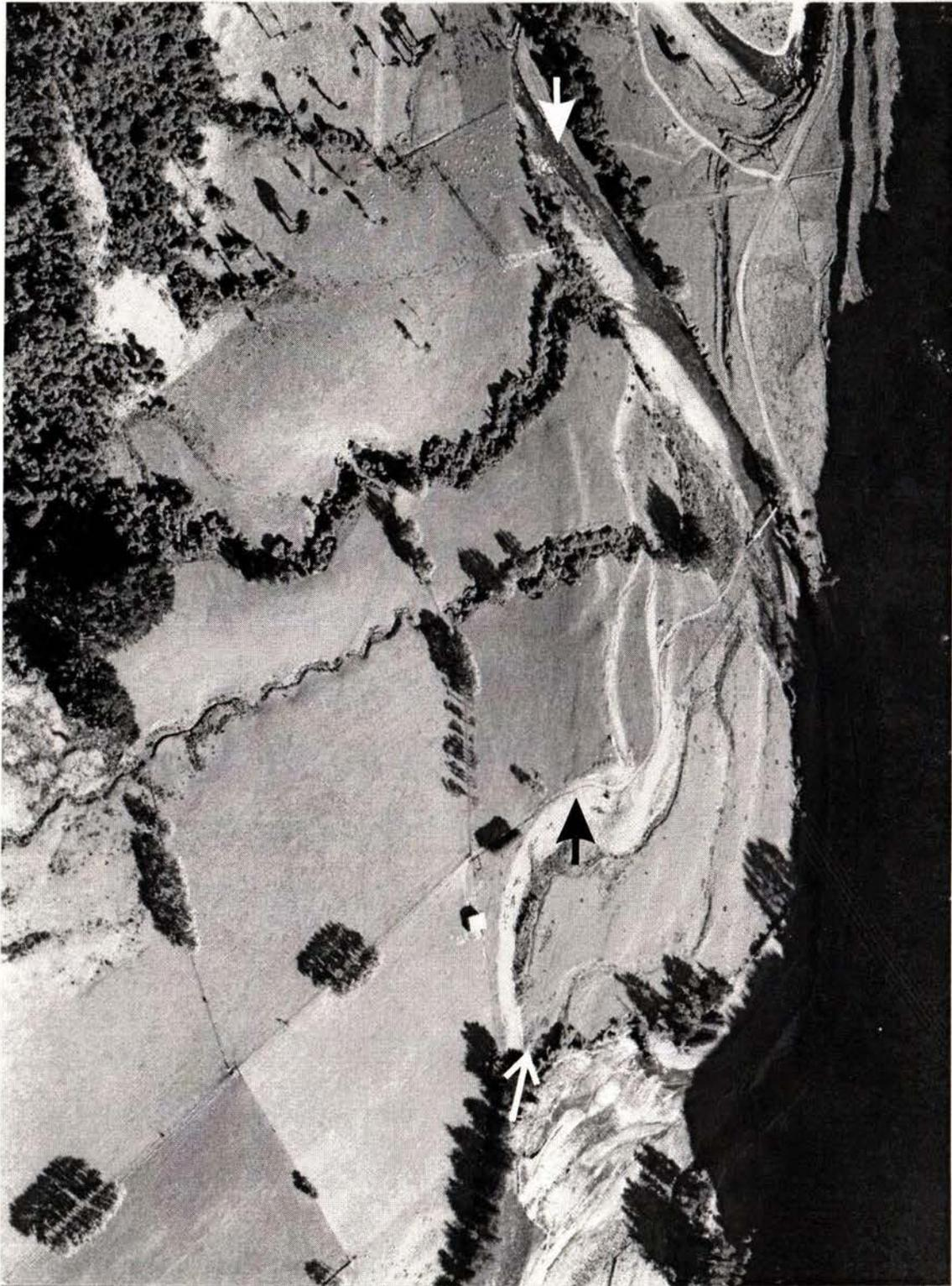
**Fig. 12.** Aerial photograph looking northwest across the scarp of the Northern Ohariu fault, Poads Road, Ohau River area (grid ref. S25 081 579). Bold arrows show the fault's location across Ohakean age terrace, and finer arrow shows location of possible scarp on Holocene degradational terrace. The photograph shown in Fig. 11 was taken just to the left (southwest) of this photo.
