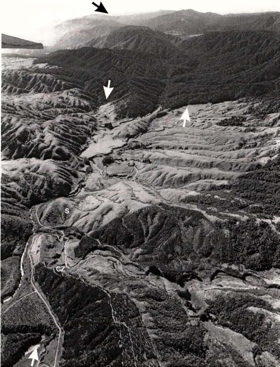
**Fig. 13.** Aerial photograph looking east-northeast along the Northern Ohariu fault, Makahika Stream area. Bold arrows show the locations of the fault traces. Makahika Stream flows top to bottom along left side of photo, and Makahika Station is located near the center. "cz" and "s" are locations discussed in text. The area shown in this photograph encompasses that shown in Figs. 14-16.
