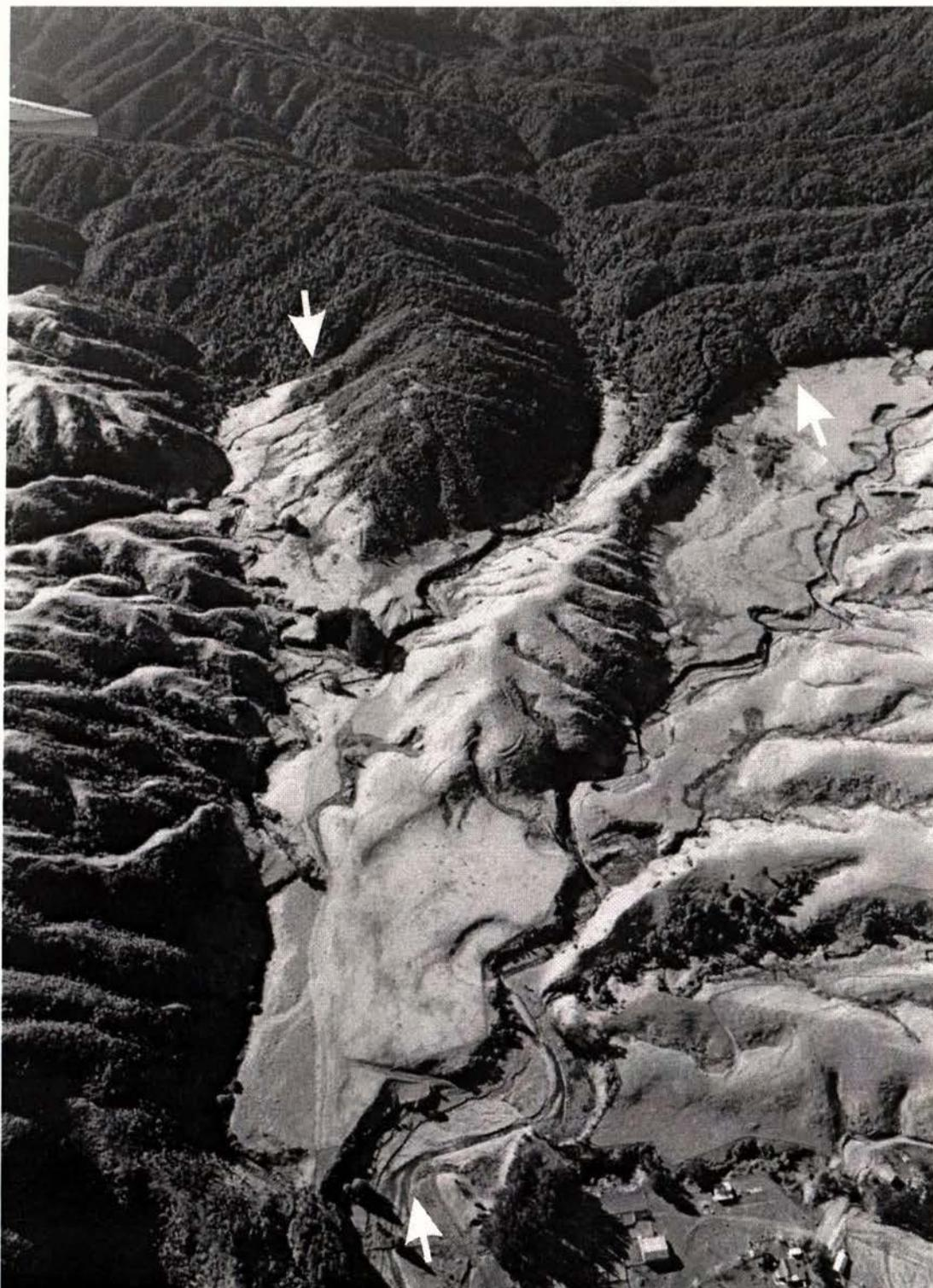
**Fig. 16.** Aerial photograph looking east-northeast along traces of the Northern Ohariu fault, Makahika Stream area. The bold arrows show the locations of fault traces. The prominent displaced alluvial terrace in the foreground is Ohakean in age, and is the same as that shown in Fig. 14. The forested ridges and valleys that are displaced by the arrowed fault trace in the upper centre-right of the photo comprise a dissected alluvial fan of Marton age (ca 140 000 years) or greater.
