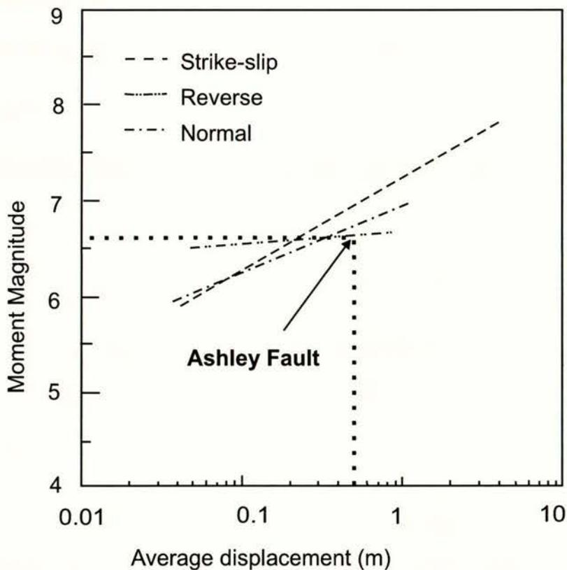
**Fig. 15.** Regression lines for strike-slip, reverse and normal slip relationships. Displacement of 0.5 m per event on the Ashley Fault resulting in a minimum Moment Magnitude of 6.6.
