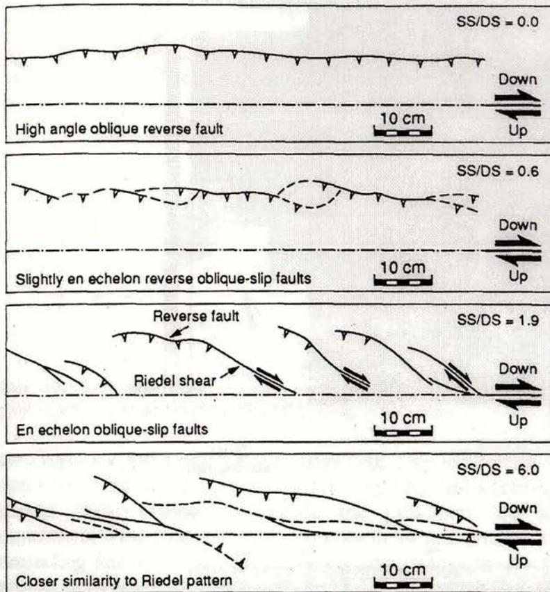
Fig. 7. Reverse oblique-slip faulting: fault patterns formed above a reverse basement fault (Richard et al, 1995)
