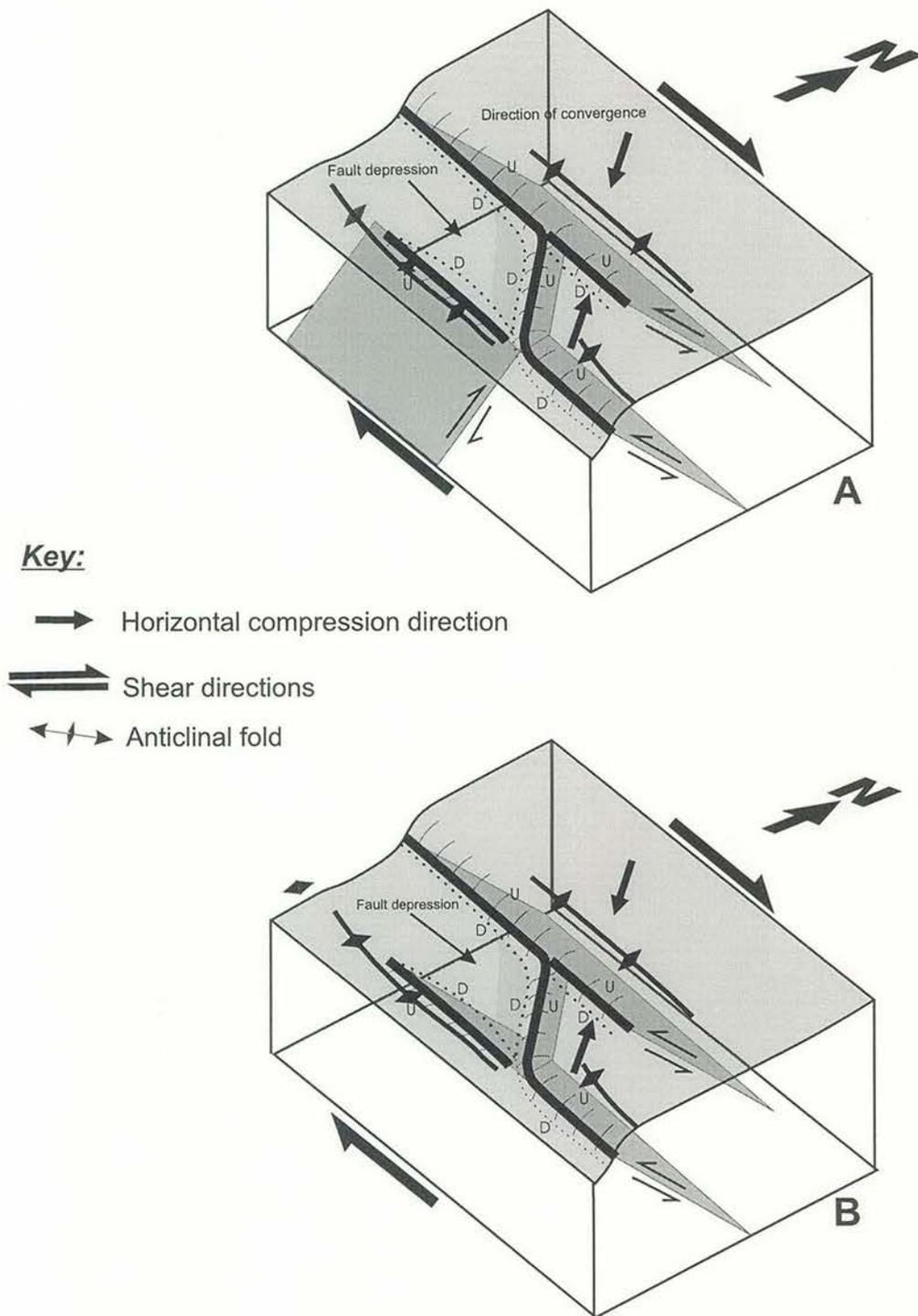
**Fig. 5. A)** Model of the fault depression formed by a southward dipping fault plane on the southern side of the depression. **B)** Model of the fault depression formed normal fault on a north dipping fault plane on the southern side of the depression. Normal faulting occurring as a result of post-event settlement.
