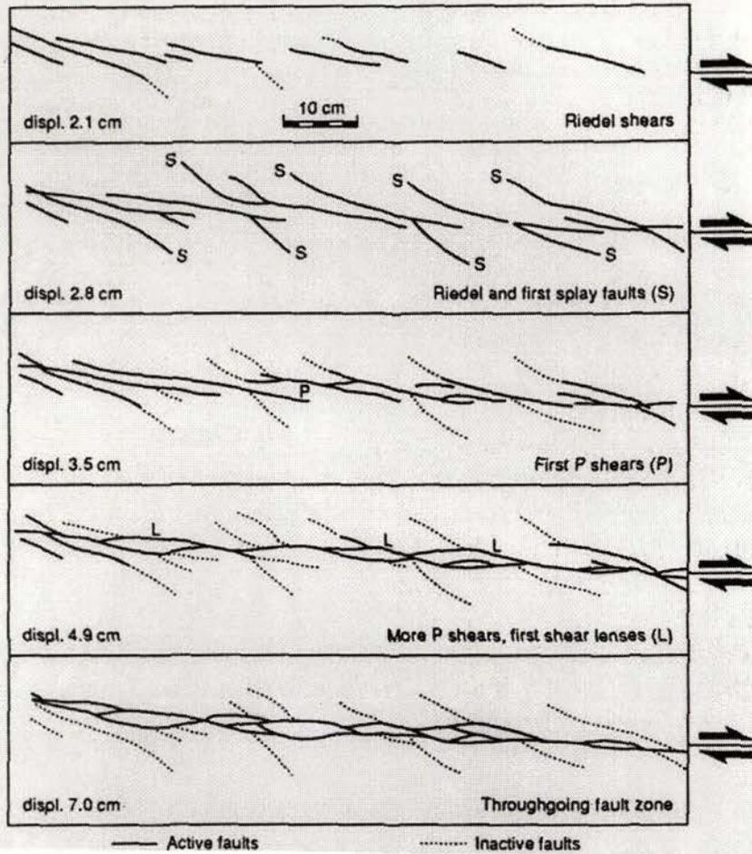
Fig. 6. Sequential development of a dextral thoroughgoing strike-slip fault zone (from Naylor et al, 1986).
