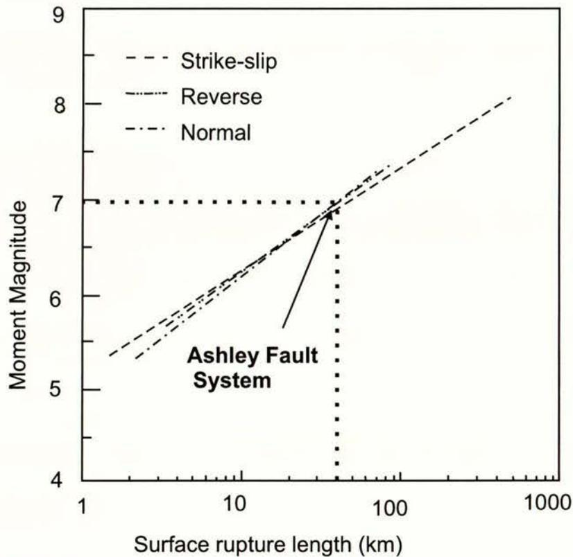
**Fig. 14.** Regression lines for strike-slip, reverse and normal slip relationships. Relationships of the Ashley Fault System indicate a maximum possible Moment Magnitude of 6.9 for the Ashley Fault.
