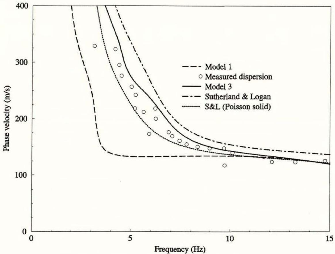
**Figure 4:** Calculated and observed dispersion values for the Parkway site. Model 1 is clearly inadequate to explain the measured dispersion, while model 3 is acceptable, being comparable to the Sutherland and Logan (1998) result if a Poisson solid is assumed. The Sutherland and Logan (1998) s-wave profile, when combined with measured p-wave velocities, gives less credible dispersions.
