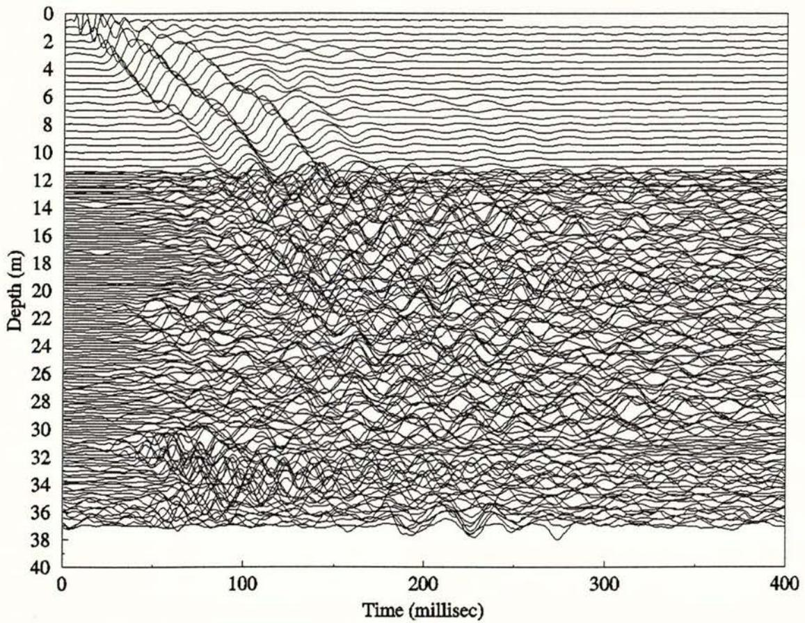
**Figure 1:** Seismograms of horizontal motion plotted as a function of depth, for the Parkway SCPT probe.
