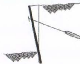
(c) Pullout failure of tendon/grout bond
