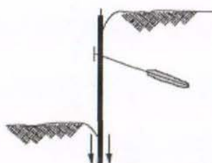
(g) Failure due to insufficient axial capacity
