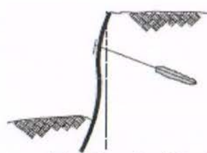
(e) Failure of wall due to insufficient passive capacity
