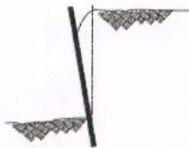
(f) Failure by forward rotation (cantilever before first anchor installed)
