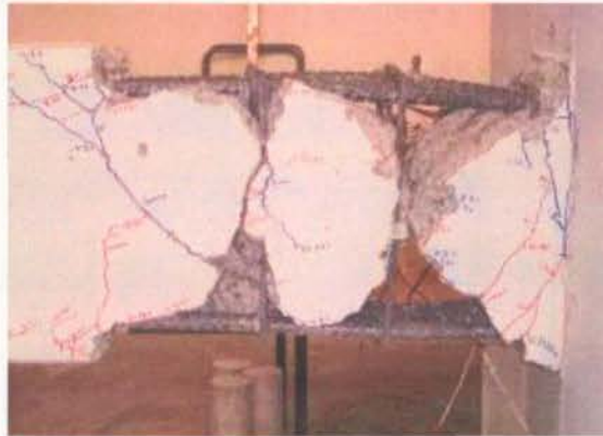
Figure 4.8-End of test after removing spalled concrete showing deformation of reinforcement (A1)
