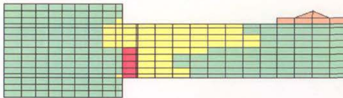
Figure 5.40-Failure and damage regions (Shear failure) (C2)
