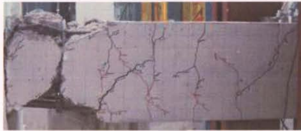
Figure 4.66-Condition of beam at the end of test (D1)
