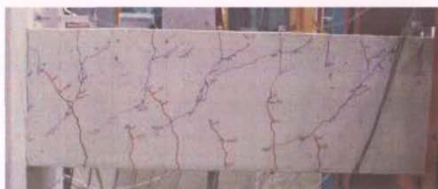
Figure 4.24-Inclination of cracks at 1.0% displacement (B1)
