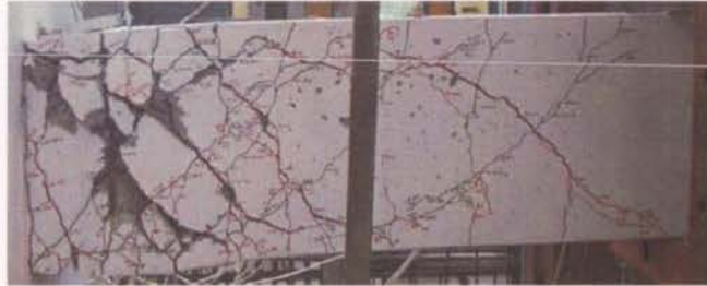
Figure 5.16-Experimental crack pattern (A2)
