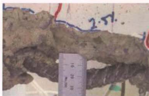
Figure 4.46-Pronounced buckling at 3.0% drift (C1)
