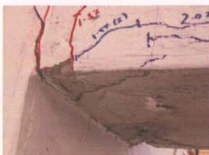
Figure 4.25-Spalling of concrete at 2.0% drift (B1)
