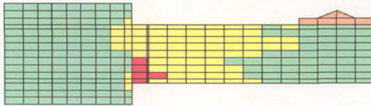
Figure 5.34-Failure and damage regions (Tension failure) (C1)
