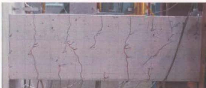
Figure 4.23-Flexural cracks after one complete cycle to 0.5% drift (B1)
