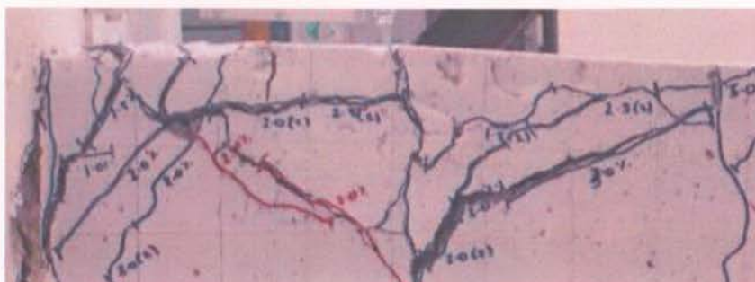
Figure 4.63-Displacement of concrete at top of beam indicating buckling at 3.0% drift (D1)
