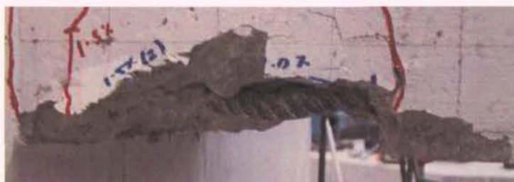
Figure 4.26-Buckled bars exposed by spalling after 2.0% drift (B1)
