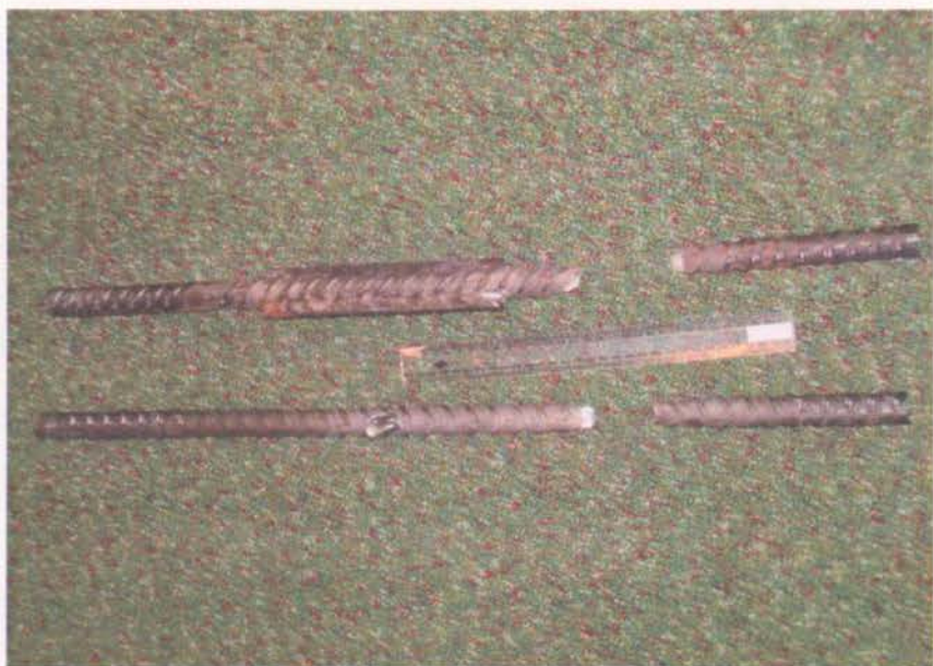
Figure A.7-Fractured steel sample of 25mm bar with stud and round bar welded to it
