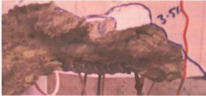
Figure 4.54-Buckling of bottom bars at 5.0% drift (C2)
