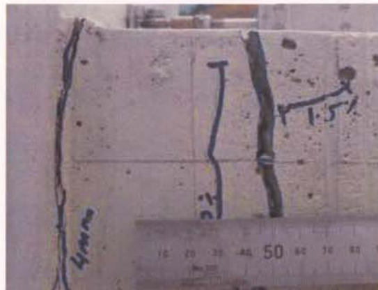
Figure 4.73-Open cracks at 2.5% drift (D2)
