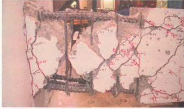
Figure 4.17-End of test after removing spalled concrete showing deformation of reinforcement (A2)
