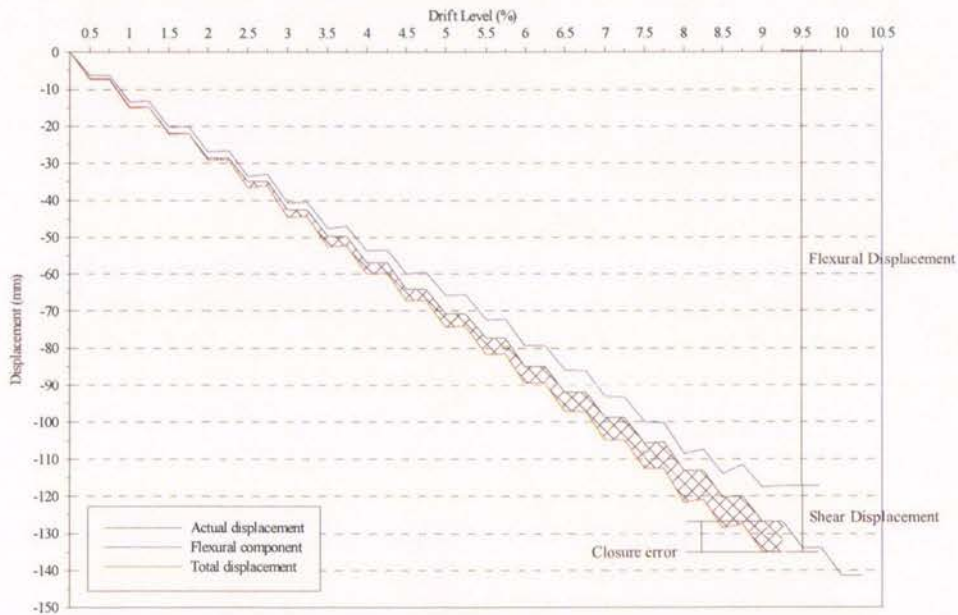
Figure 4.79-Contribution of shear and flexure to the total displacement at the peaks of the loading cycles for beam D2
