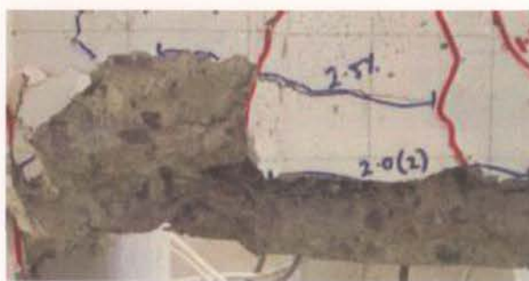
Figure 4.45-First evidence of buckling at 2.5% drift (C1)
