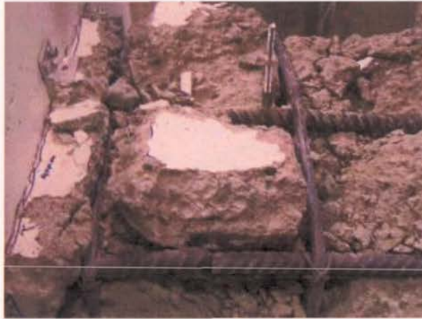
Figure 4.65-Ruptured bar and deformed stirrup at the end of test (D1)
