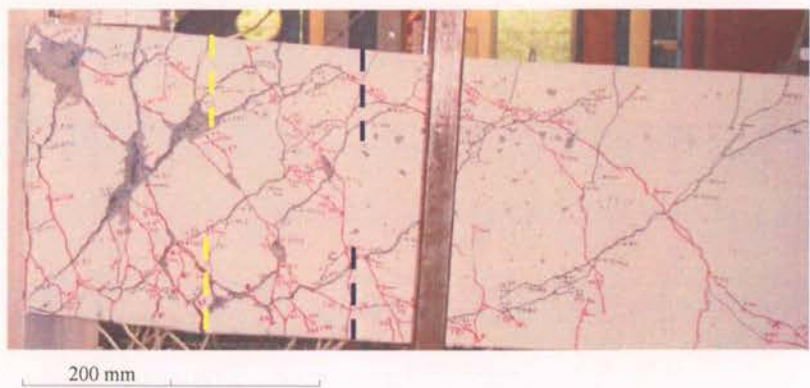
Figure 6.5-Crack widths and estimation of yielding length (A2)
