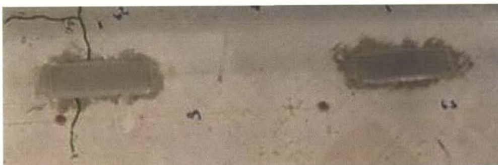
Figure 3.13: Steel strips epoxied to concrete floor.
