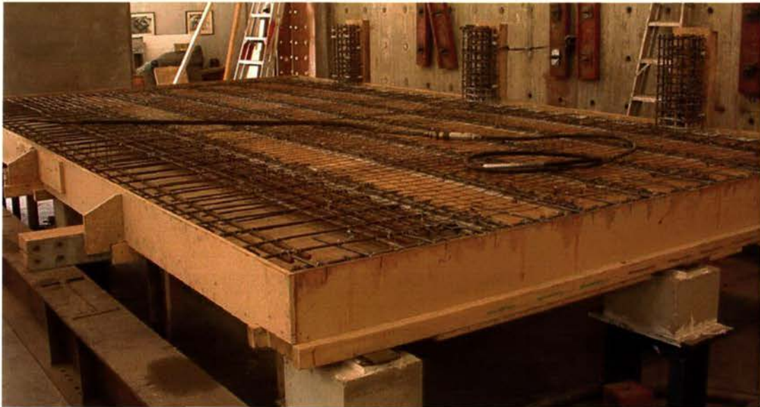
Figure 3.8: Stage III of construction of Unit 2, immediately before concreting.
