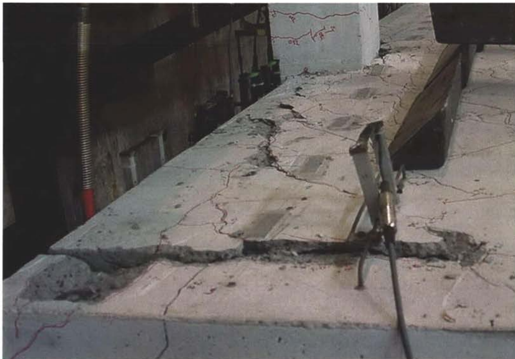
Figure 5.10: Shearing and uplift of floor at north cantilever, at 3.5% drift.
