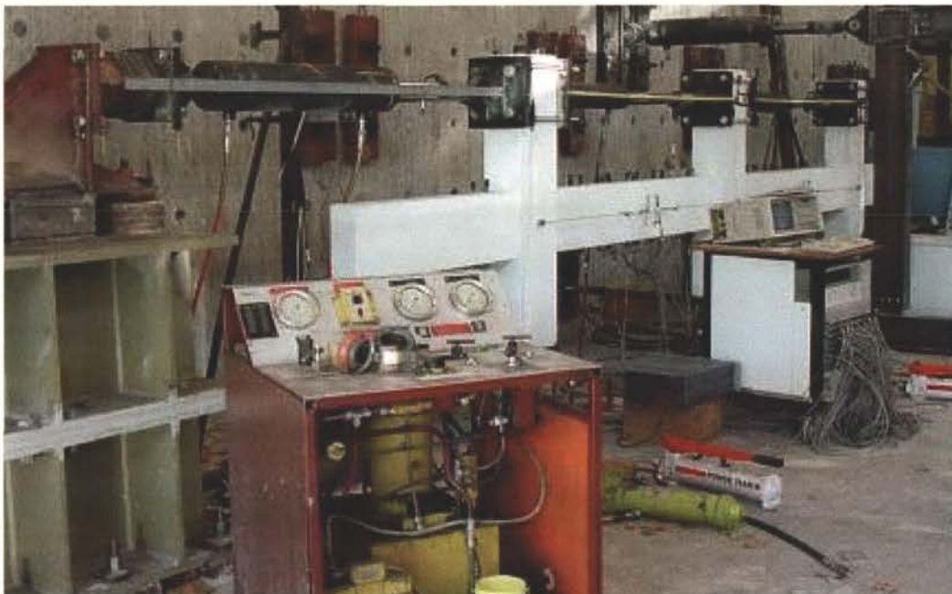
Figure 3.9: Test Arrangement of Unit 1 - motorised hydraulics control (foreground), datalogger (right), loading hydraulic actuators (top of columns), hand-pumps (on floor).
