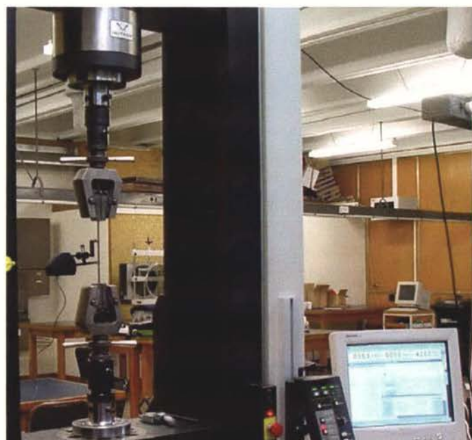
Figure 3.6: Testing of wire reinforcement on Instron Test Machine.
