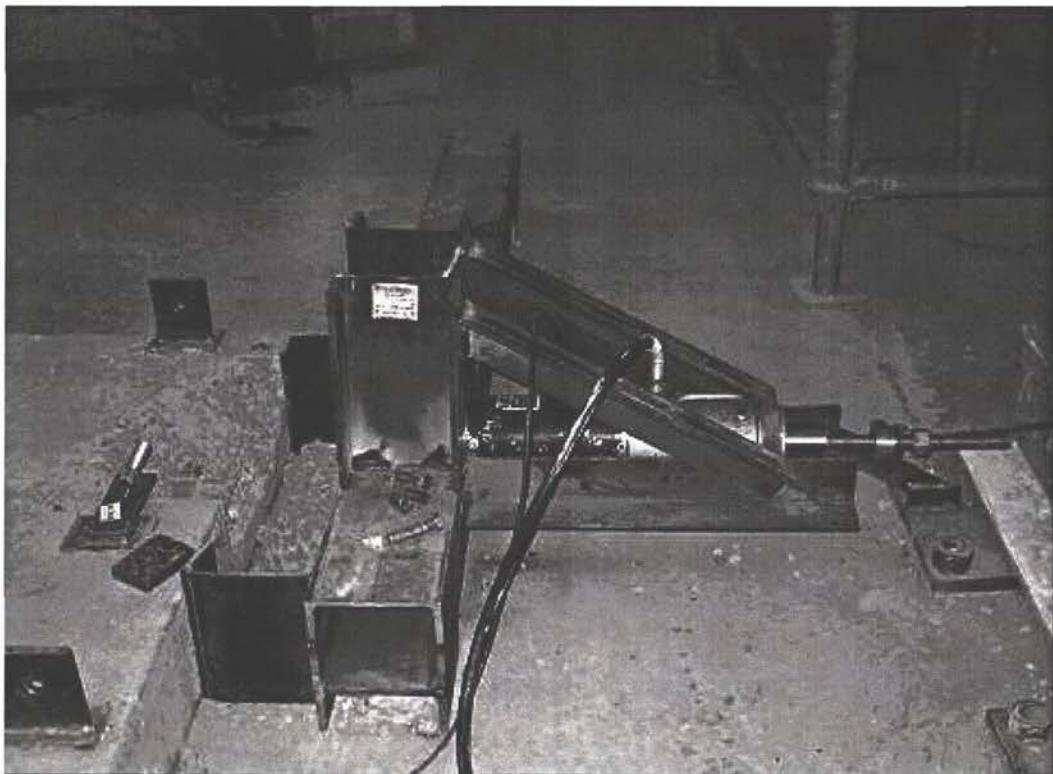
Figure 7      *Shear loading reaction frame*
