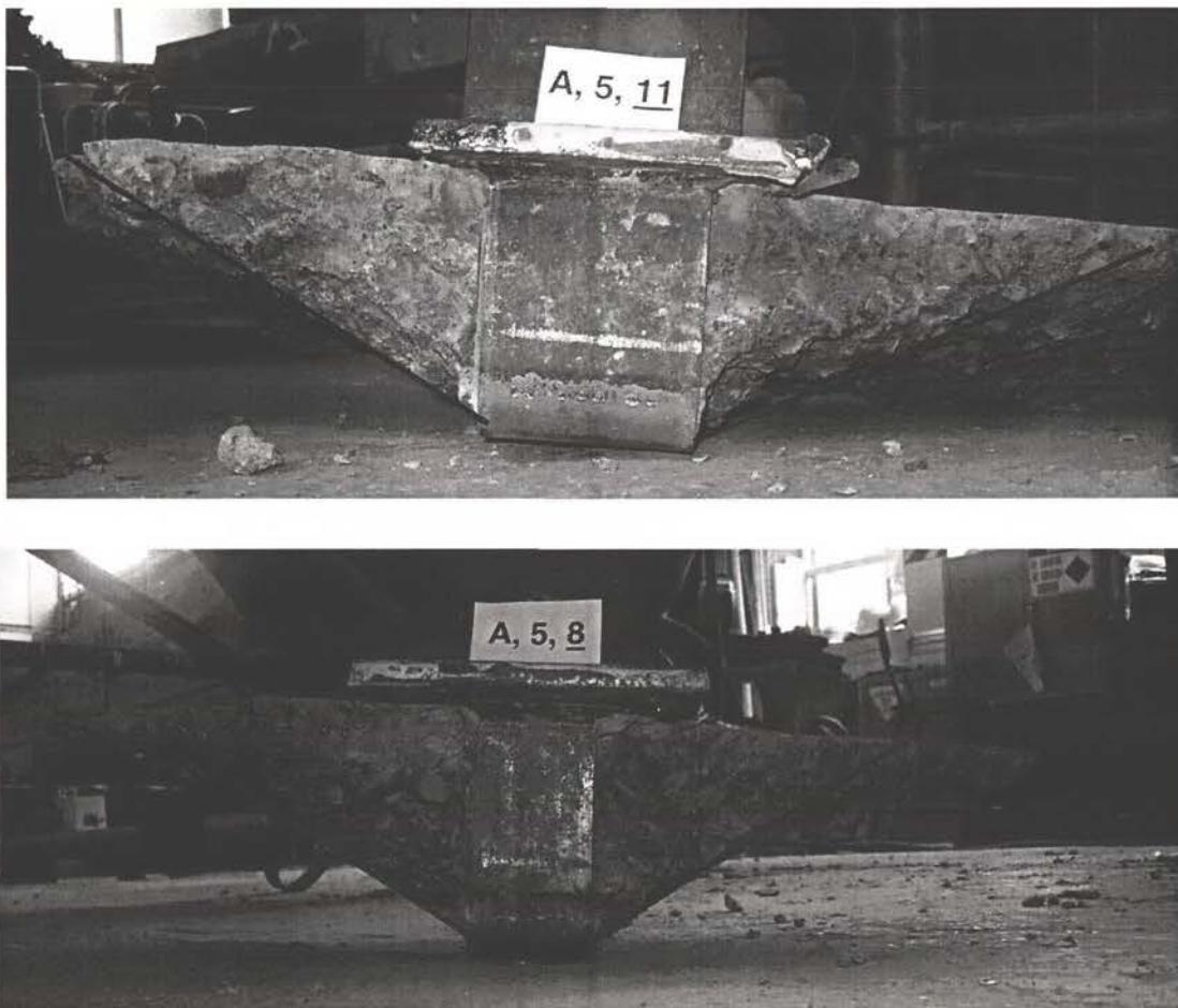
Figure 11      *General shape of the side concrete pullout cones observed during direct tension tests*
