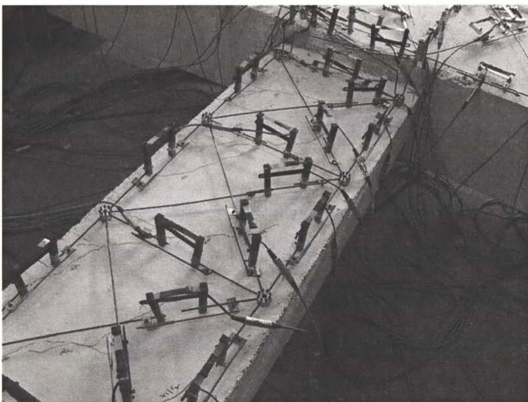
Figure 5-1 Cracking of right hand beam during first cycle to 3/4 M_n
