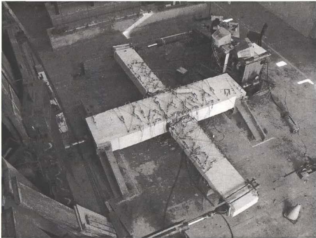
Figure 5-29 Unit 2B at 5% drift showing torsional distortion of both beams
