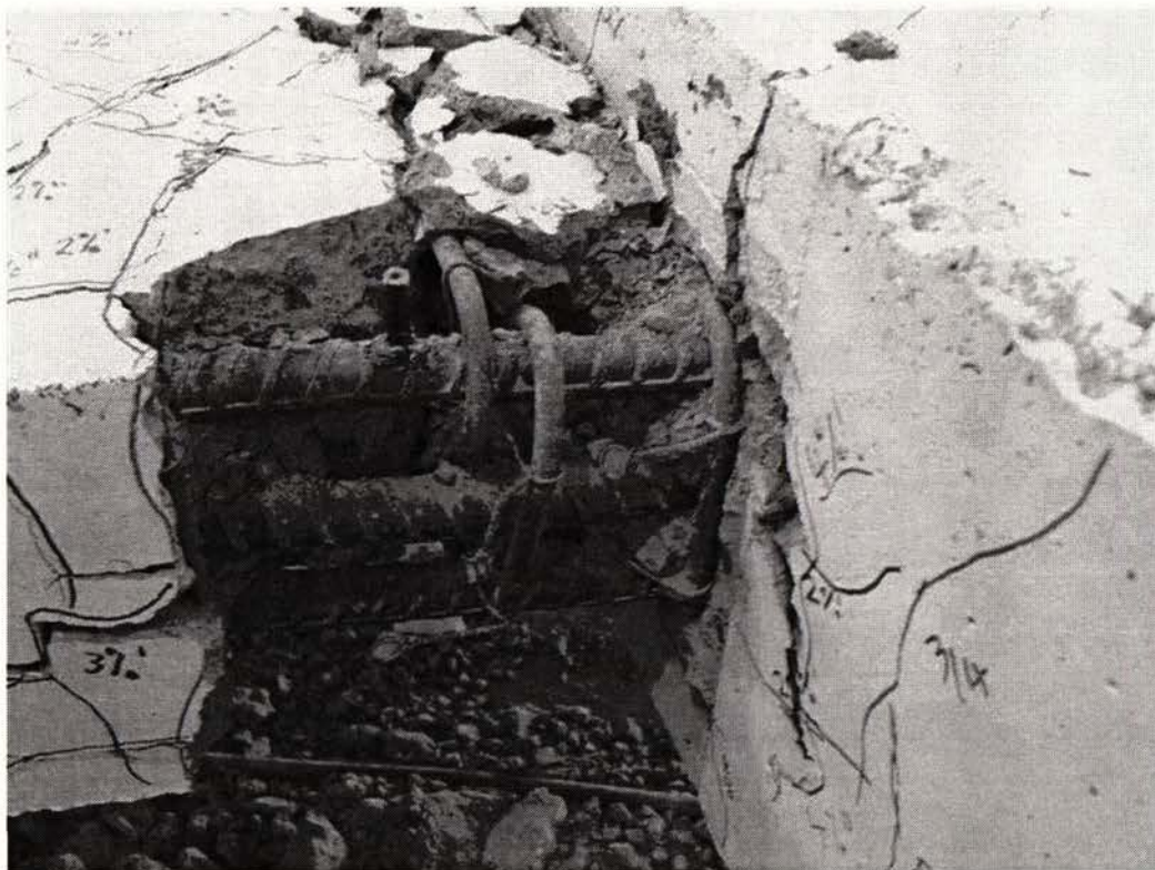
Figure 5-18 End condition of right hand plastic hinge zone showing loss of concrete
