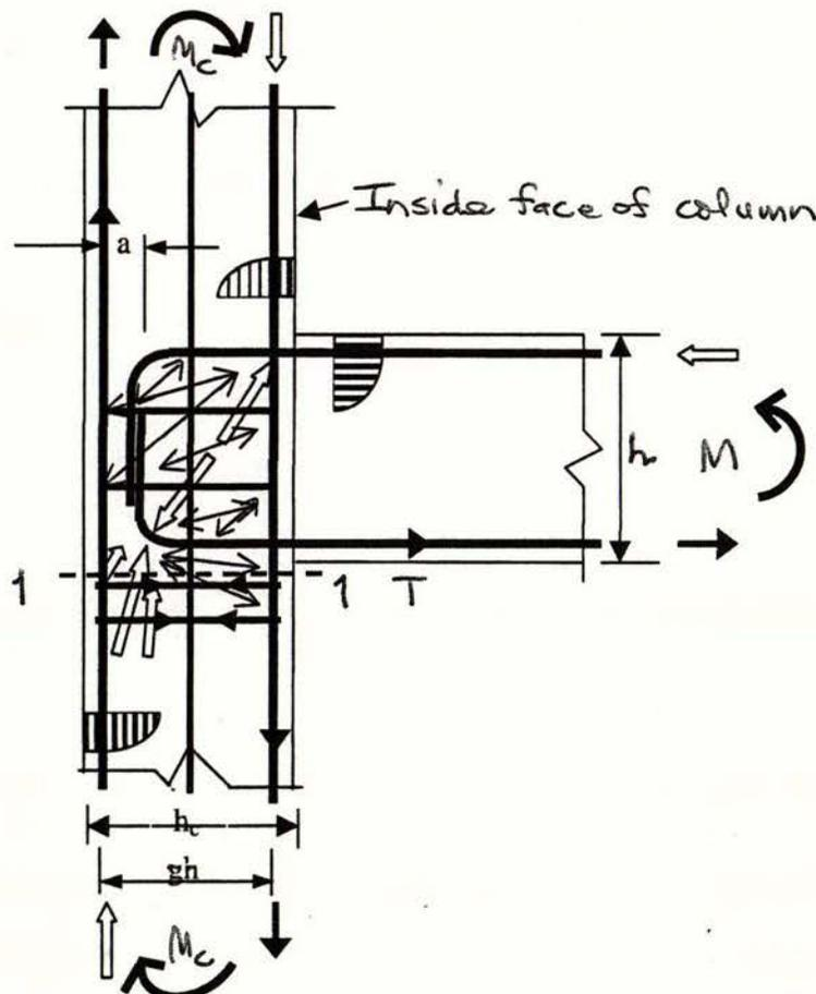
Figure 10. Actions in an external beam-column joint.
