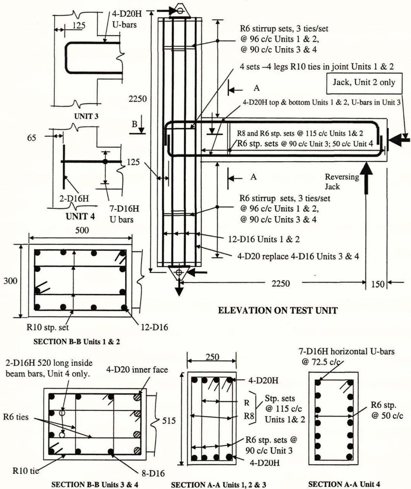
Figure 1. Dimensional and reinforcing details of test beam-column units 1-4.
