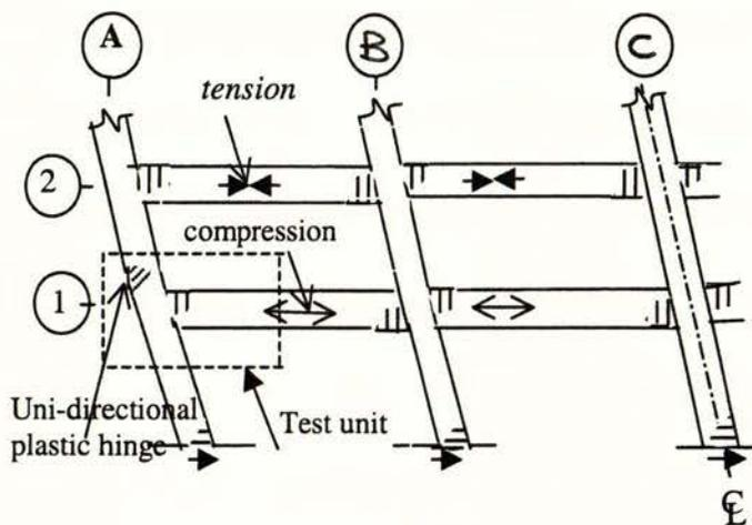
Figure 6. Deformation of column due to elongation.
