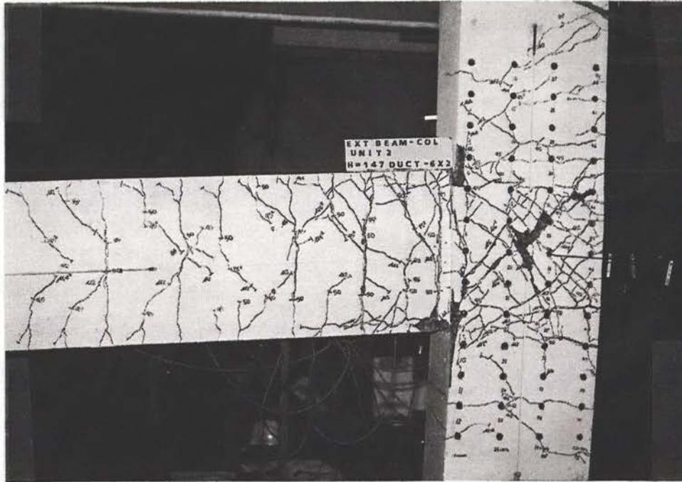
Figure 12. Unit 2 at Ductility 6, second cycle.
