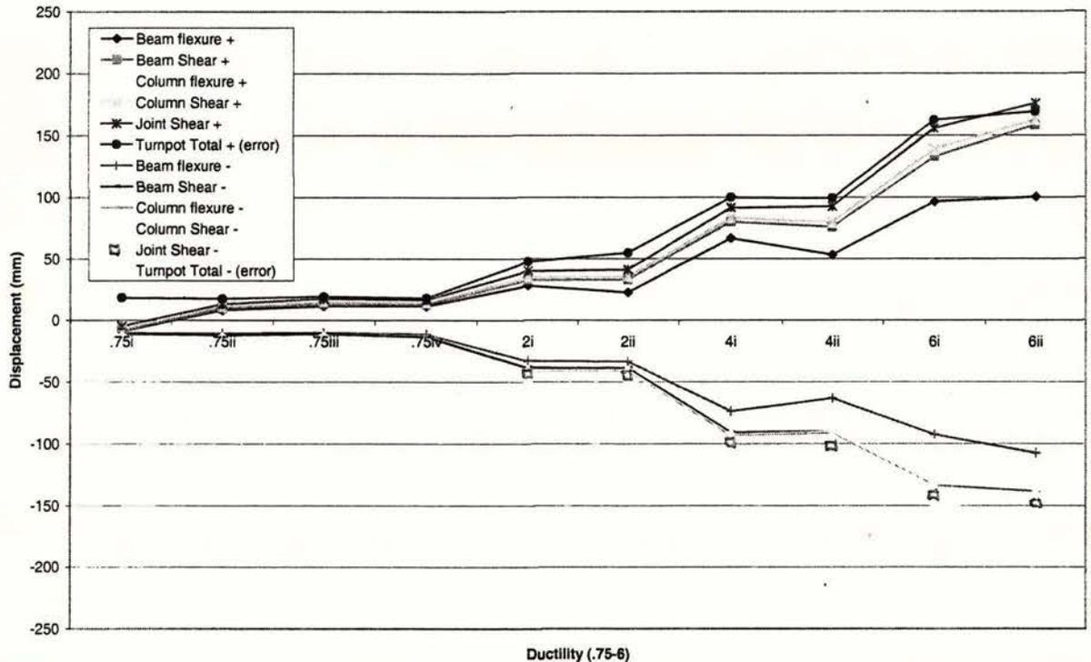
Figure 20. Unit 5: Components of flexure and shear deflection at cycle peaks.
