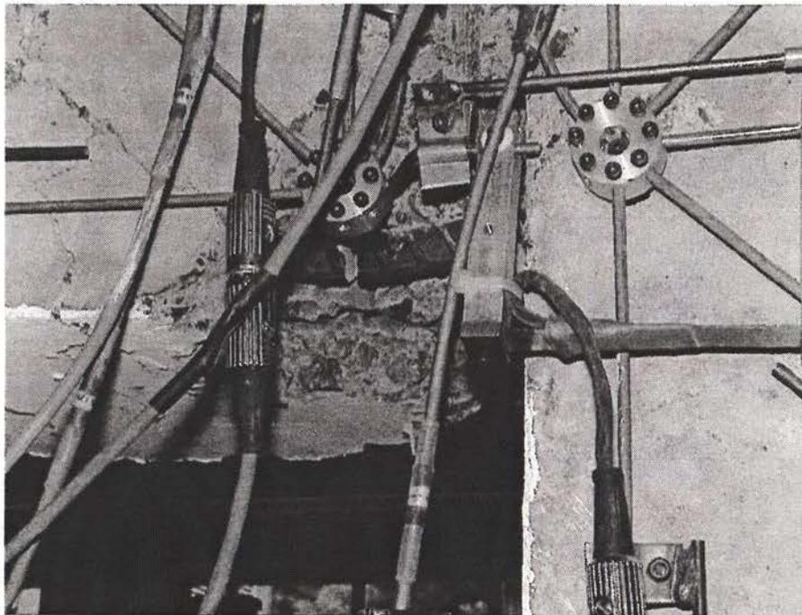
Figure 24. Unit 6 showing the beam bar fracture at stud weld location. Note fracture is at location of bar buckle.
