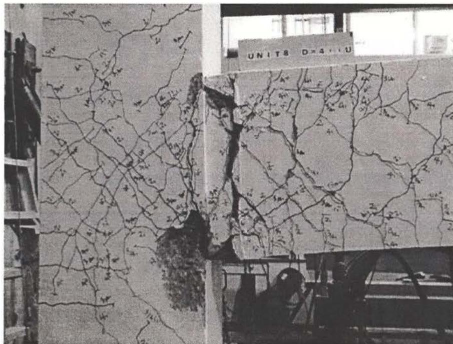
Figure 32. Unit 8 at the completion of the second ductility 4 cycle.
