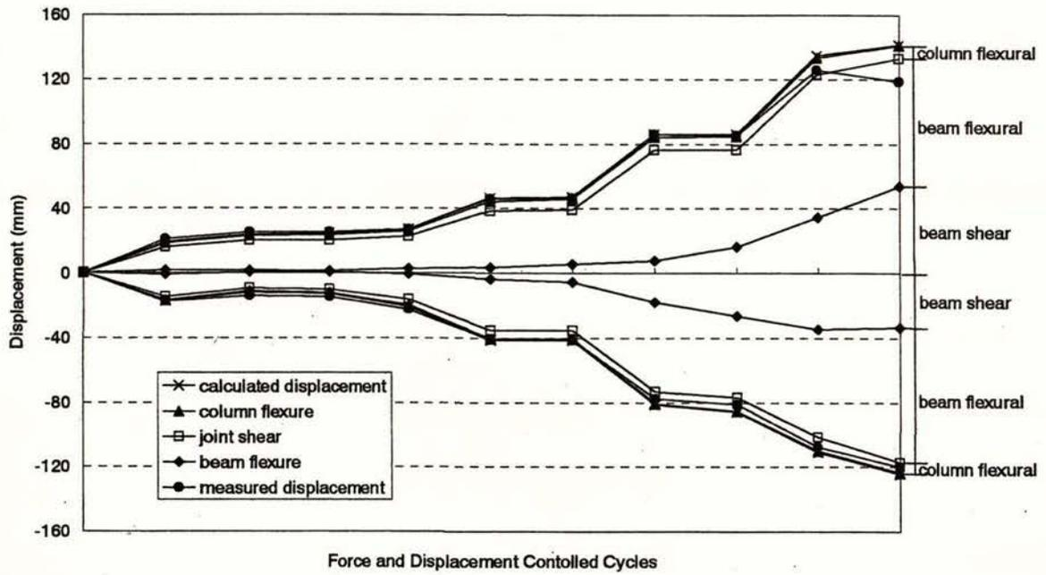
Figure 16. Shear & Flexural Displacements for Unit 3 (Kohno [4]).
