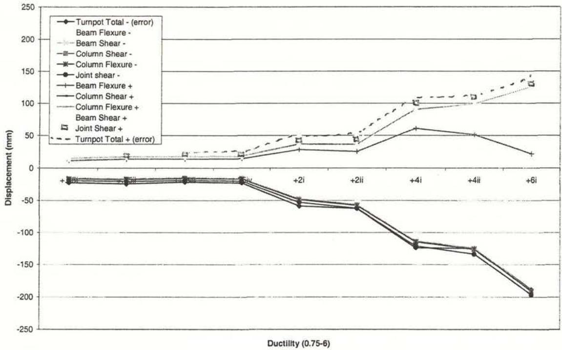
Figure 31. Flexural and shear deflection components for Unit 8 at cycle peaks.
