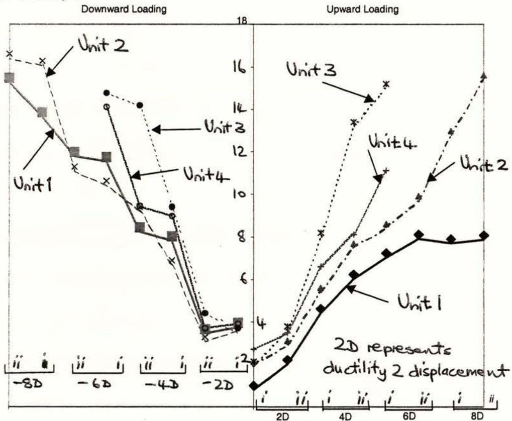
Figure 11. Beam Elongation for Beam-Column units 1-4.
