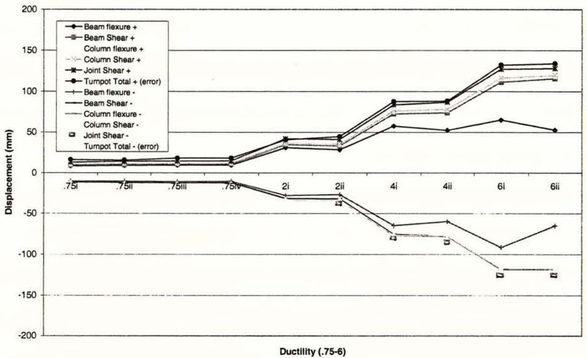
Figure 28. Flexural and shear components of deflection for Unit 7.
