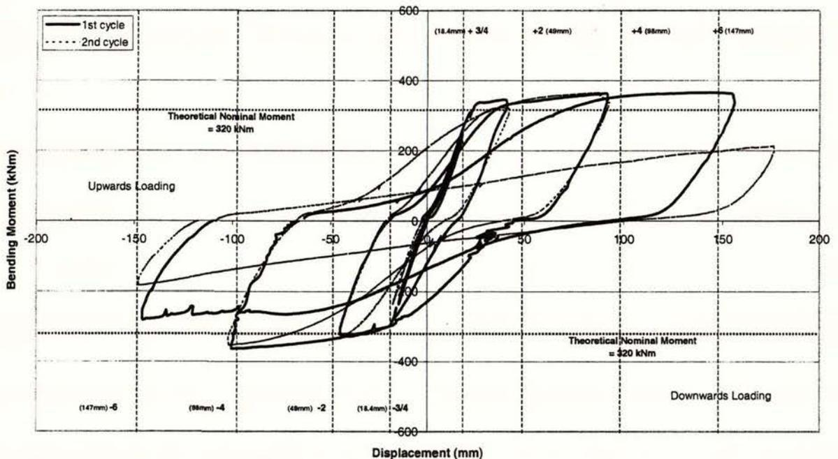
**Figure 19. Unit 5: Beam moment (applied force x 2 metres) at column face versus beam deflection at the position of loading.**
