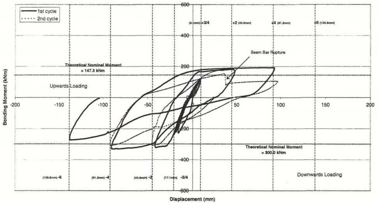
Figure 23. Unit 6 Beam bending moment at column face – Beam tip deflection hysteresis loops. Shows sudden drop in applied force when beam bar fractured.
