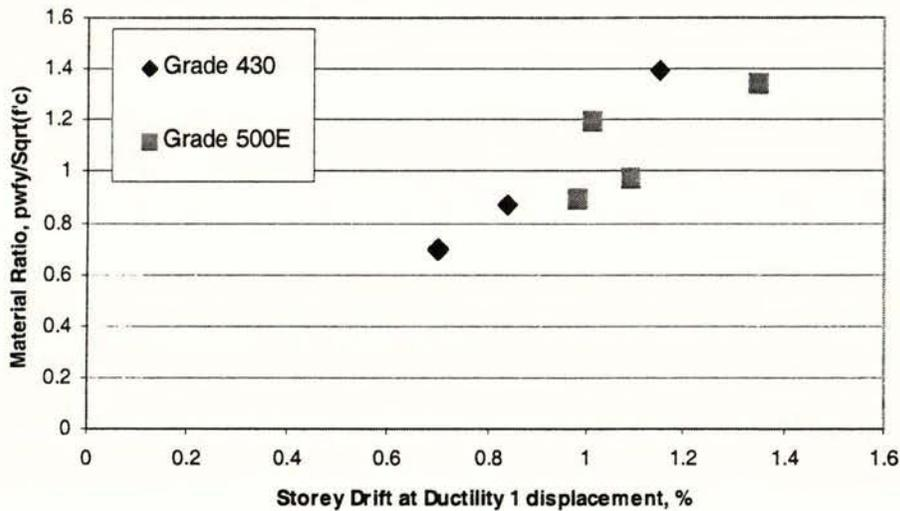
Figure 35. Ductility 1 storey drift verses Material Ratio,  $p_w(f_y/\sqrt{f'_c})$ .
