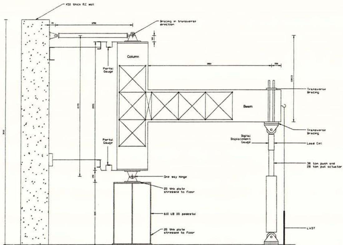
Figure 5. Test unit set up for units 5-8. Units 1-4 identical except for horizontal jack at beam free end in unit 2.
