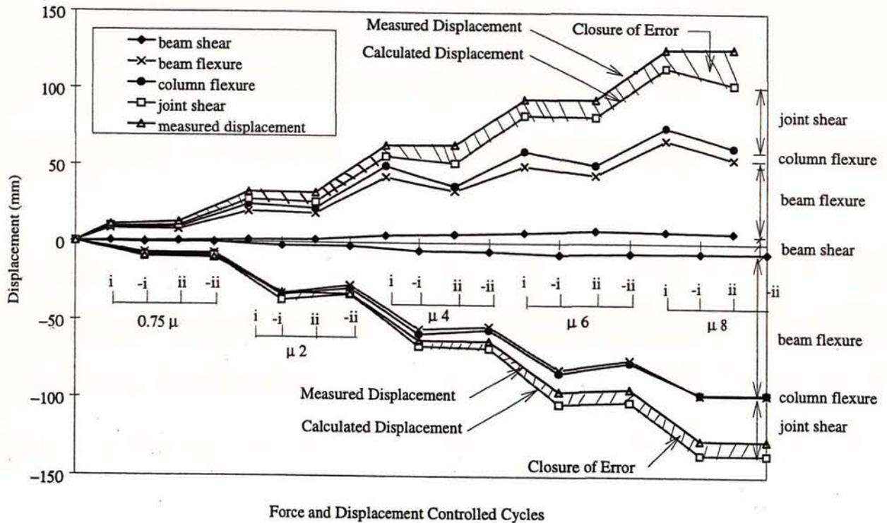
Figure 14: Unit 2 components of flexure and shear deformations (Henao [3]).
