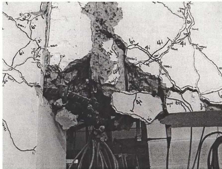
Figure 22. Unit 5 showing buckled beam bar detail, at the end of the second downward ductility 6 cycle.
