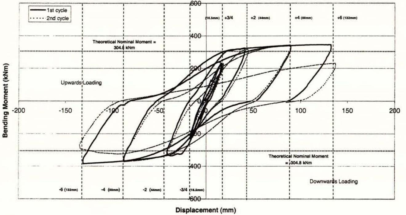
Figure 27. Unit 7 Beam bending moment at column face – Beam tip deflection.
