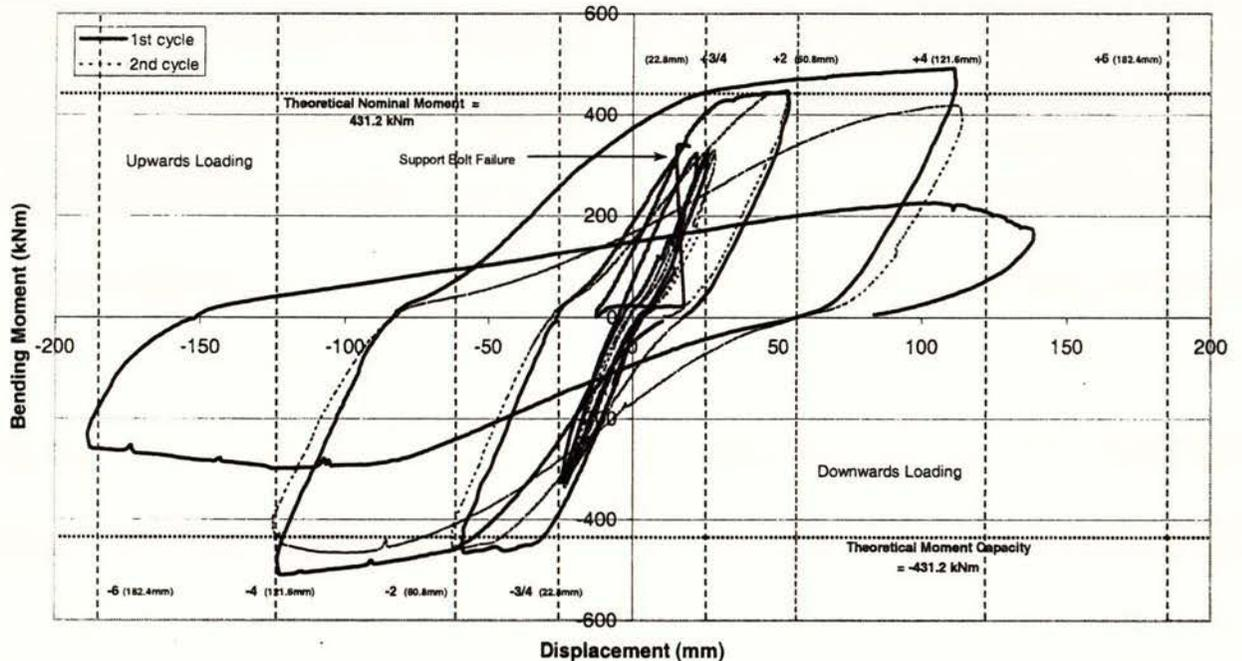
Figure 30. Unit 8 Beam bending moment at column face – Beam deflection hysteresis loops.
