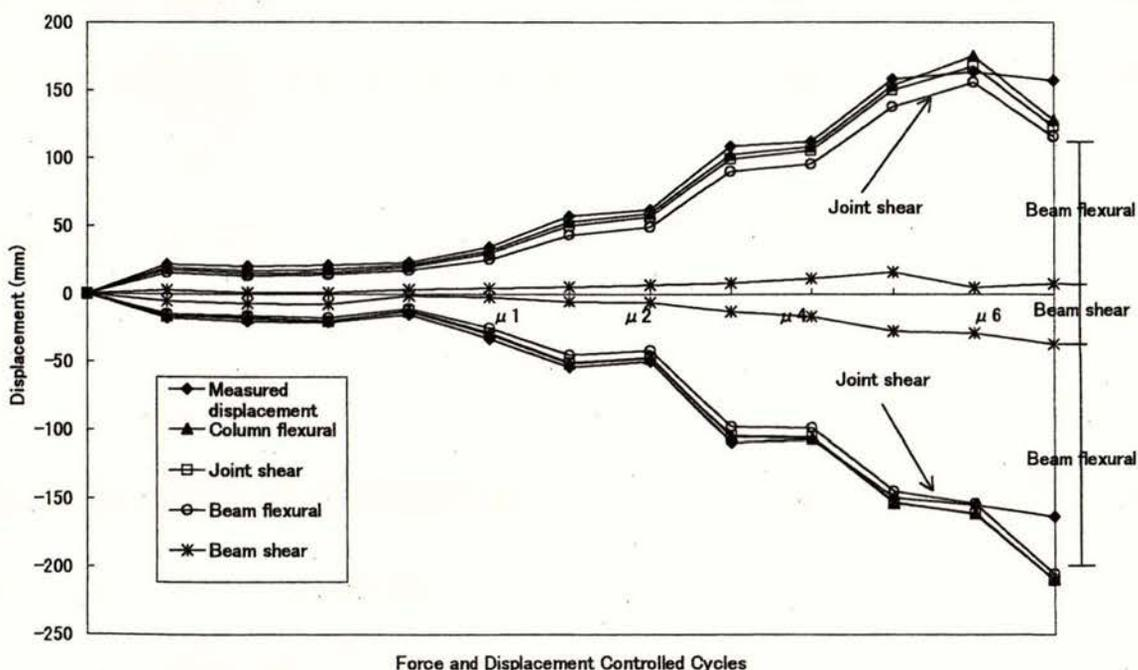
Figure 18. Flexure and shear components of deflection for Unit 4 (Kohno [4]).
