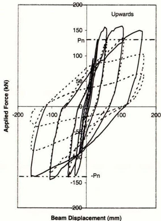
Figure 17. Unit 4 Applied Force- Beam Displacement loops.
