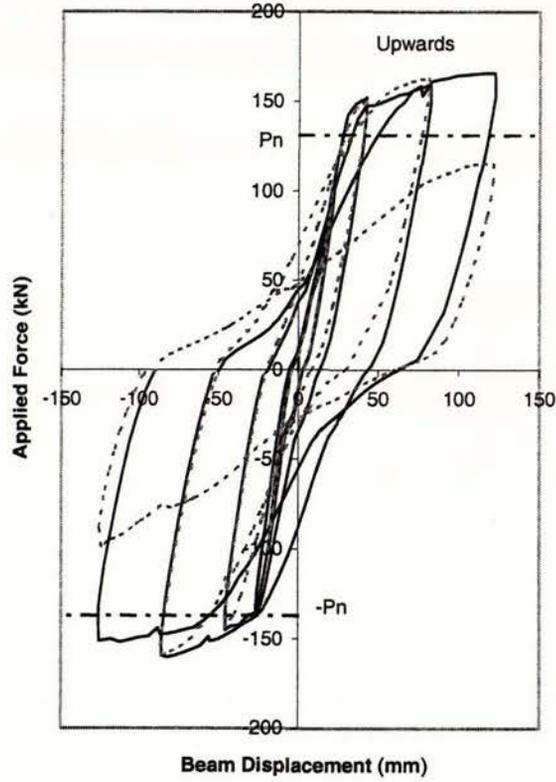
Figure 15. Unit 3 Applied Force- Beam Displacement loops.
