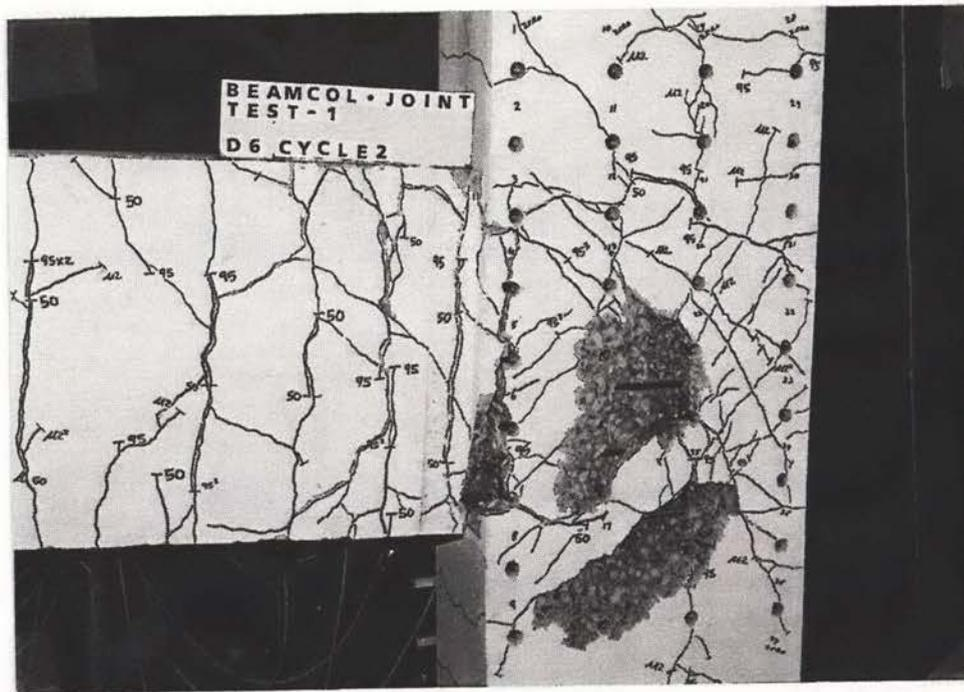
Figure 9. Unit 1 at Ductility 6, second cycle.
