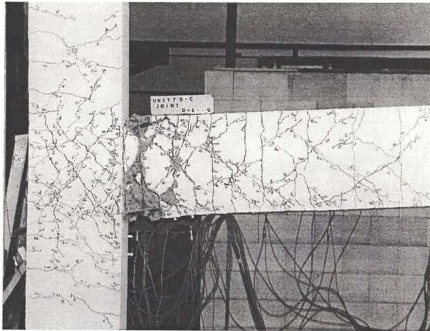
**Figure 29. Unit 7 after completion of the second cycle to ductility 6.**
