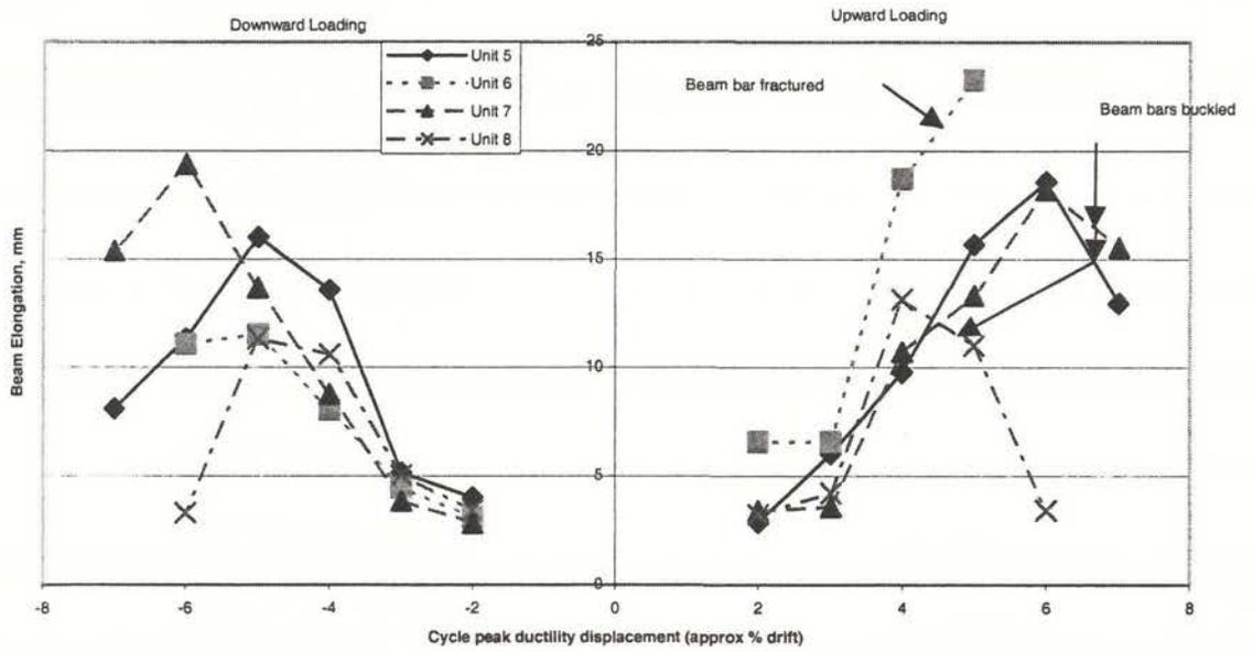
Figure 34. Measured beam elongation in Units 5-8.
