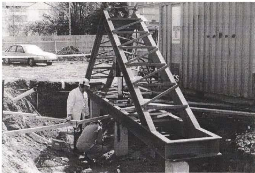
Figure 17. Full-scale cyclic load test frame and actuator.
