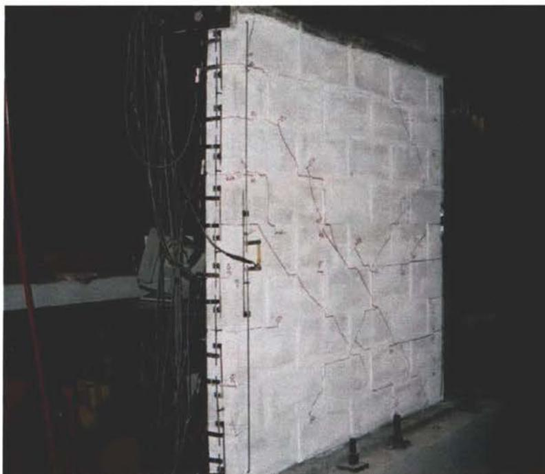
Photo 9 Diagonal cracking after first cycle of  $\pm 4$  mm displacement.
