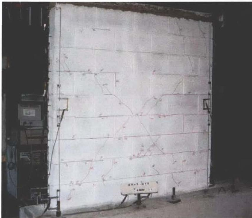
Photo 18 Formation of x-shaped diagonal crack after first cycle to  $\pm 4$  mm displacement.
