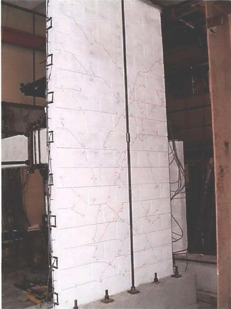
Photo 39 Condition of test wall after first cycle to  $\pm 12$  mm displacement.
