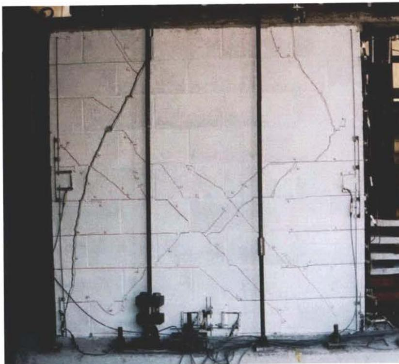
Photo 37 Condition of test wall after first cycle to  $-6$  mm displacement.
