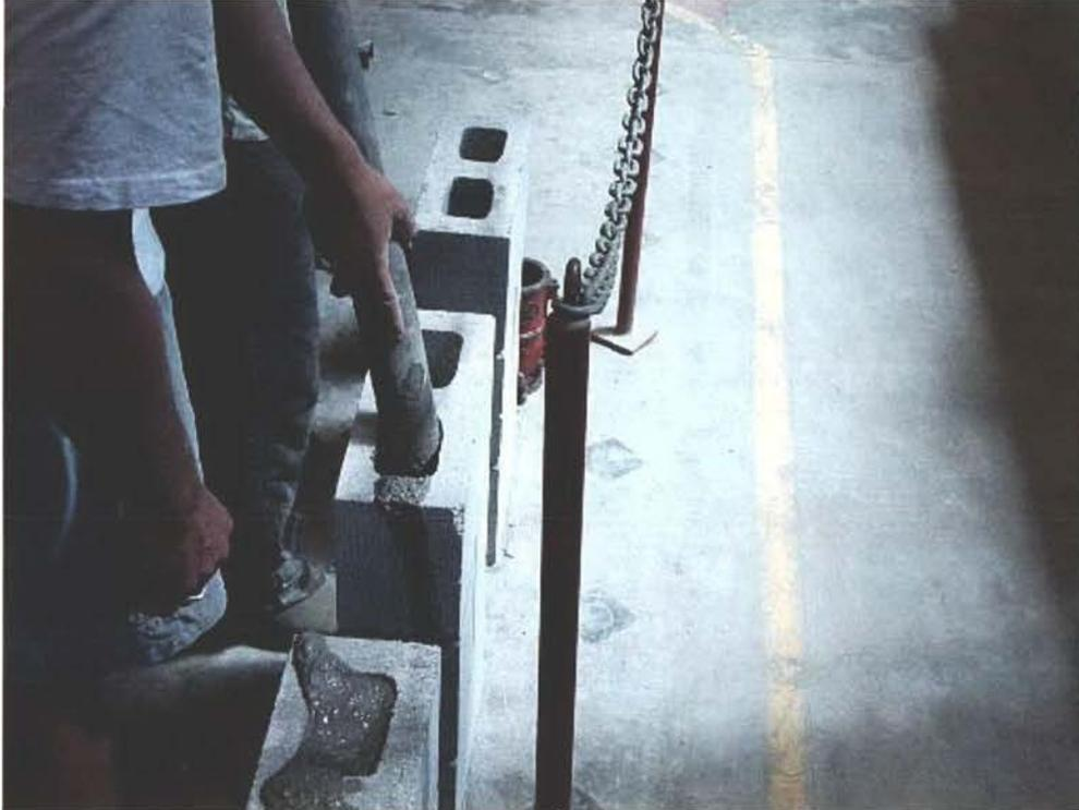
Photo 7 Masonry prisms grouting.
