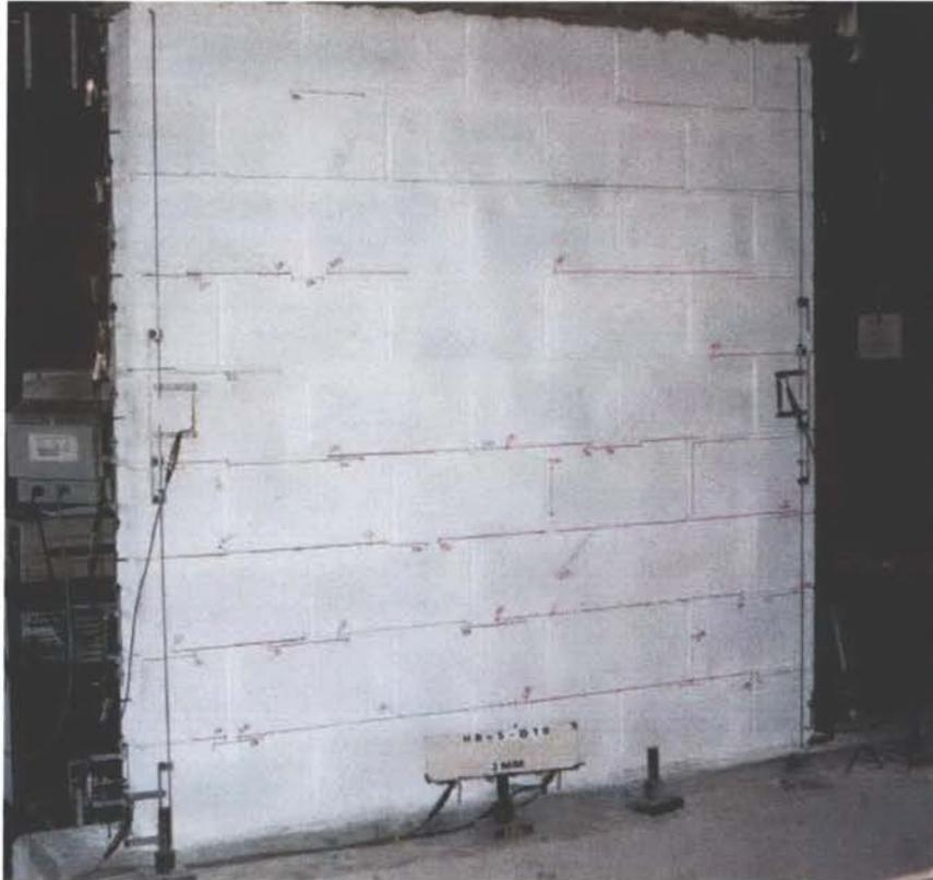
Photo 17 Condition of test wall after first cycle to  $\pm 2$  mm displacement.
