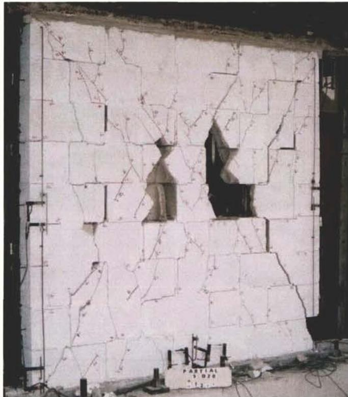
Photo 28 Wall condition after second cycle to  $\pm 12$  mm displacement.
