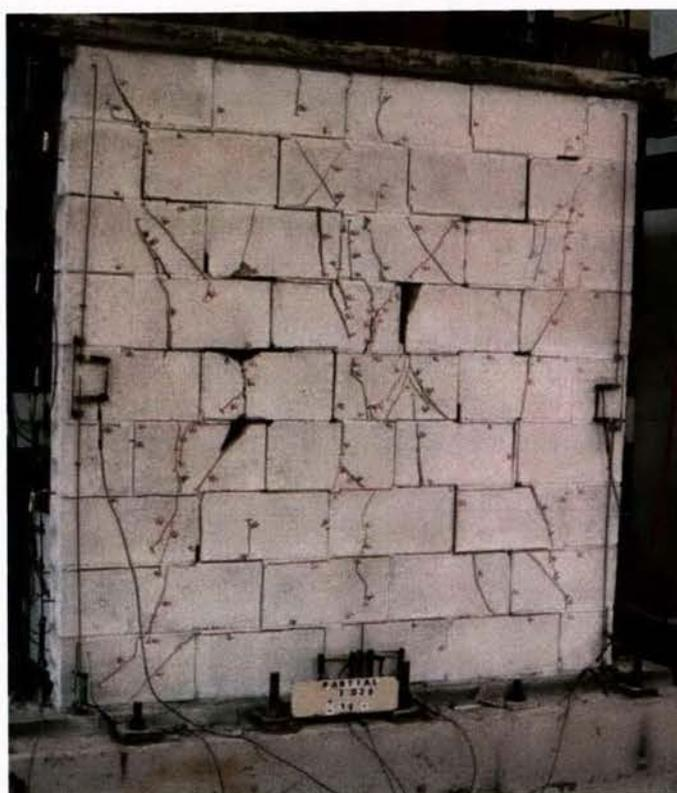
Photo 30 Condition of test wall after first cycle to  $\pm 16$  mm displacement.
