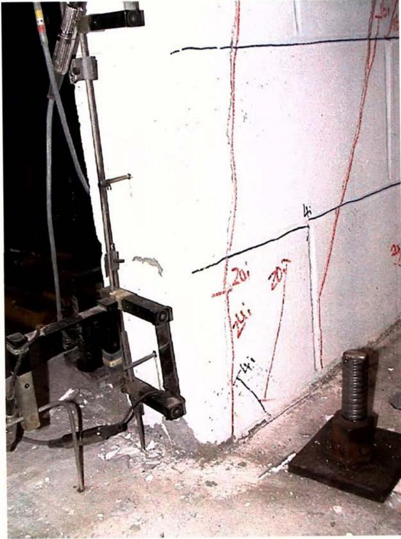
Photo 41 Condition of test wall after first cycle to  $\pm 24$  mm displacement.
