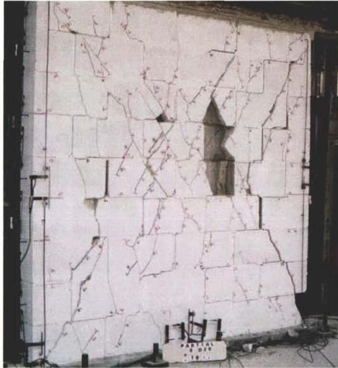
Photo 27 Wall condition after second cycle to  $\pm 10$  mm displacement.
