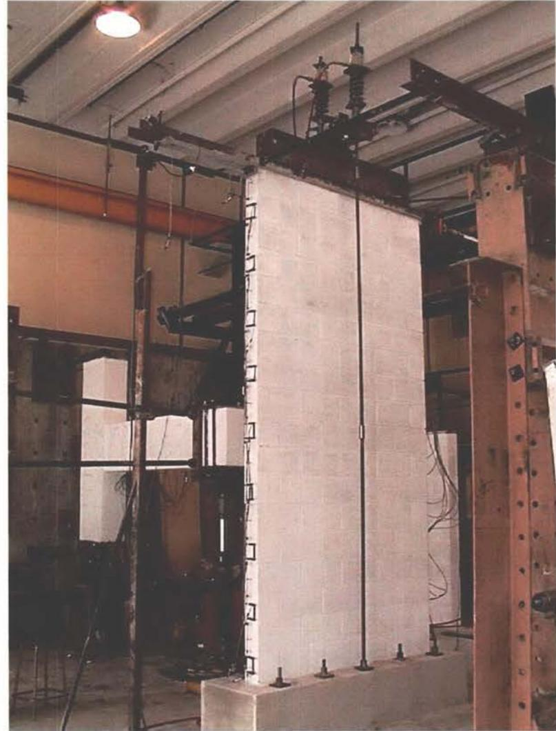
Photo 38 Test set-up for Wall 9.
