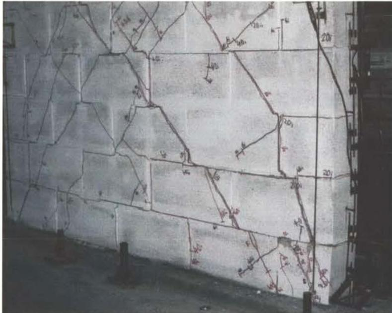
Photo 11 Compression toe degradation at +10 mm displacement.
