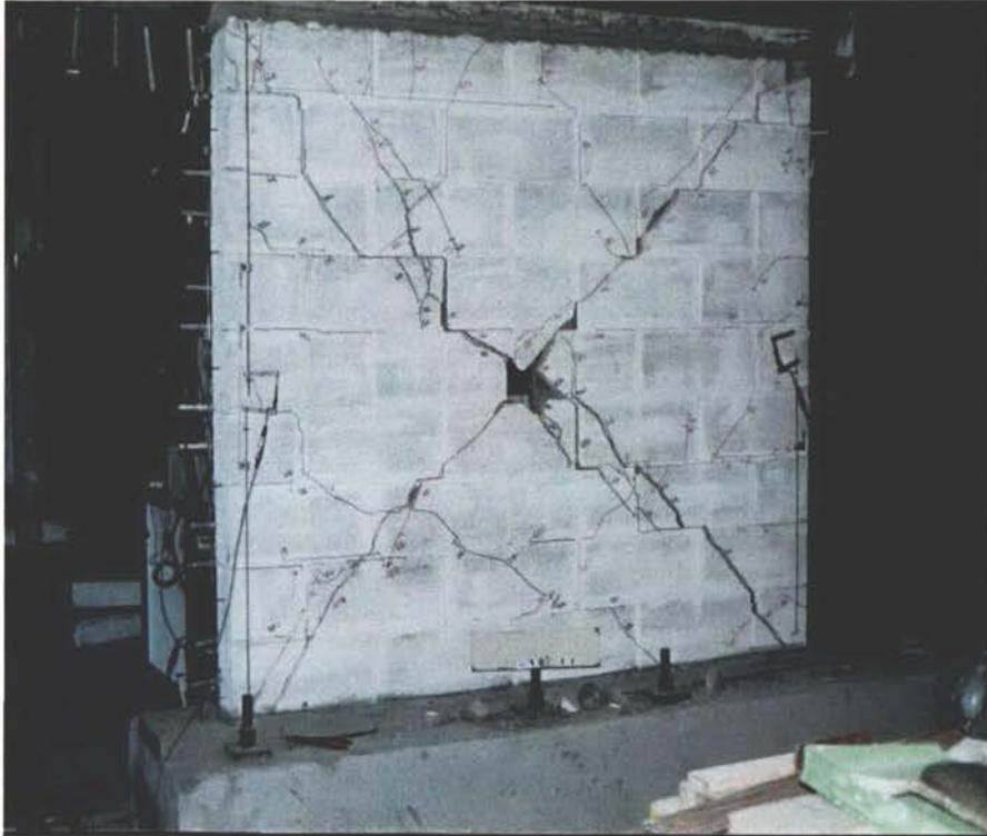
Photo 15 Crushing of masonry at second cycle of -10 mm displacement.
