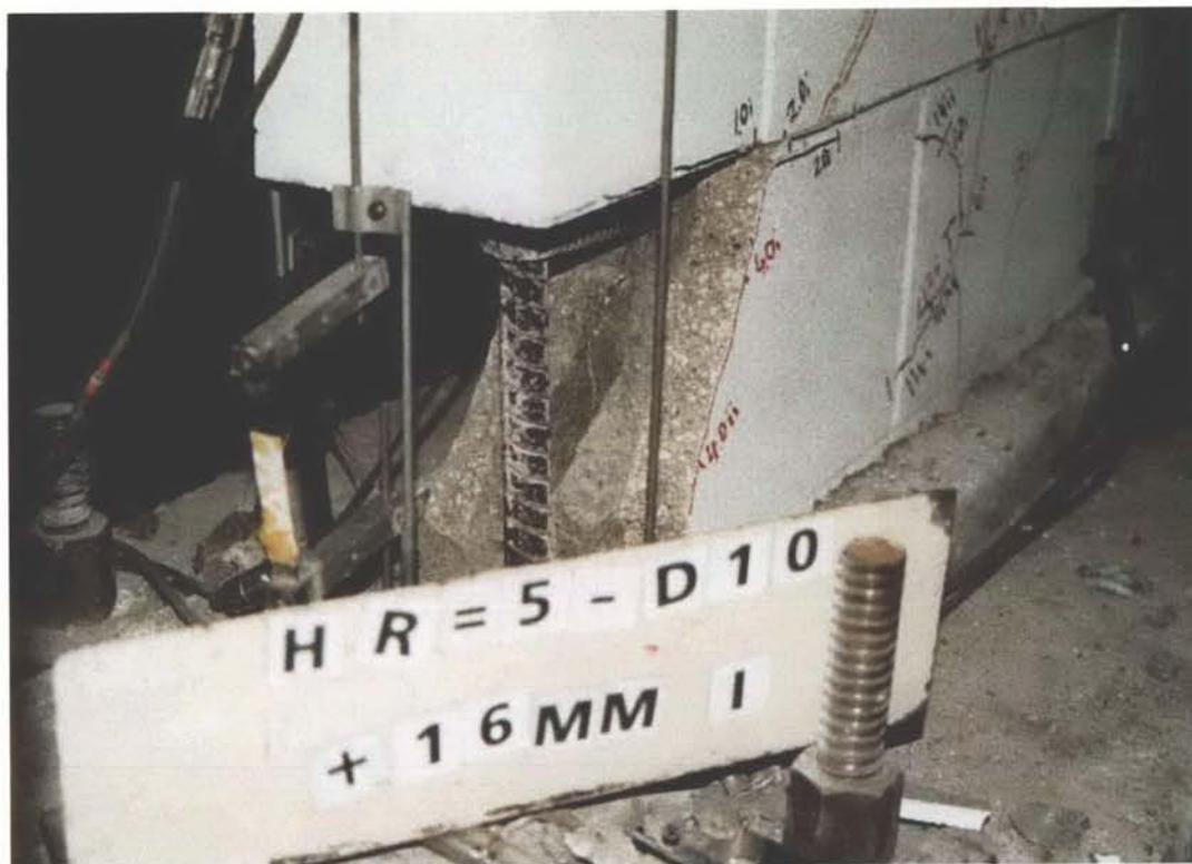
Photo 20 Wall toe condition after first push cycle to 16 mm displacement.
