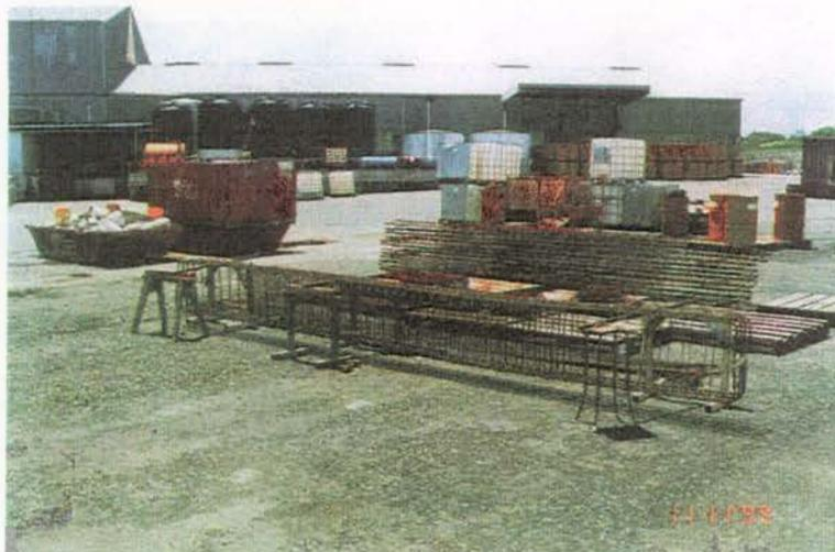
Figure 4-11 Reinforcement Cage in Upright Position
