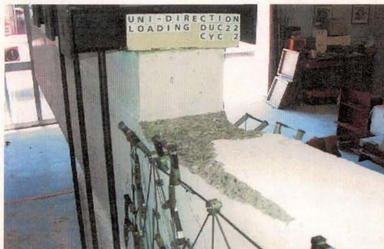
Figure C-44 Spalling of Cover Concrete (Ductility 22)
