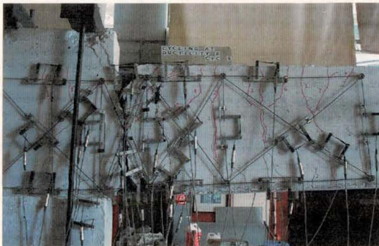
Figure C-37 Test Subassembly Condition at Ductility 8 (Cycle 6)
