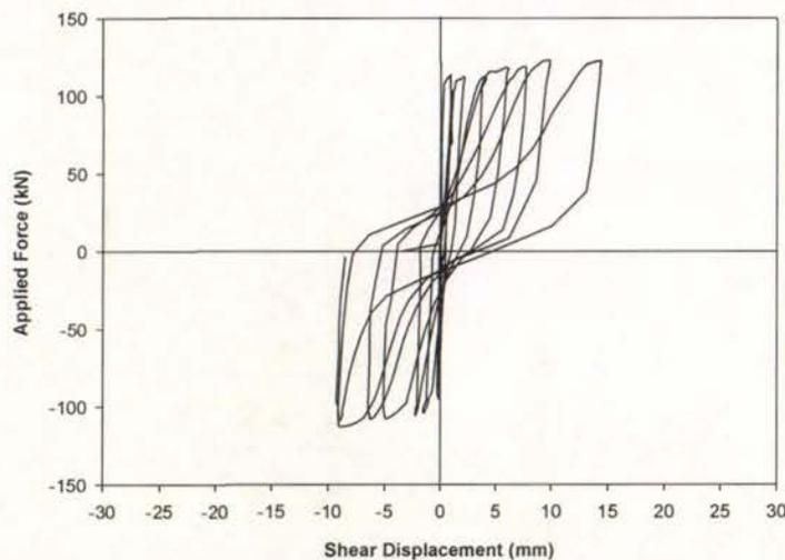
Figure C-4(b) Shear Displacement Component
