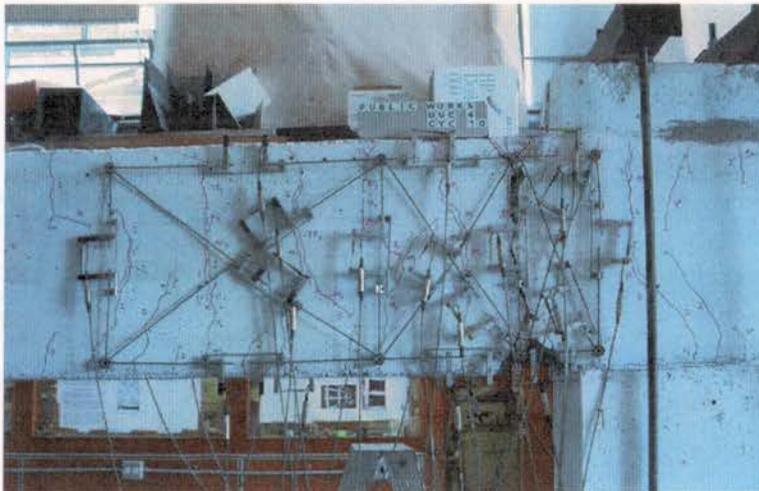
Figure C-23 Test Subassembly Condition at Ductility 4 (Cycle 10)
