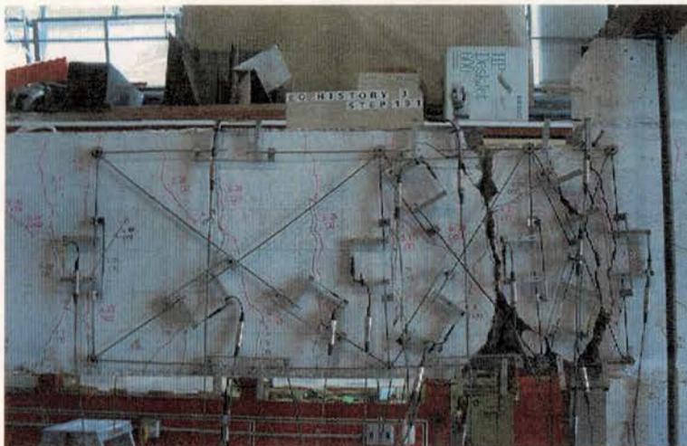
Figure C-65 Test Subassembly Condition at Conclusion of Acceleration History C
