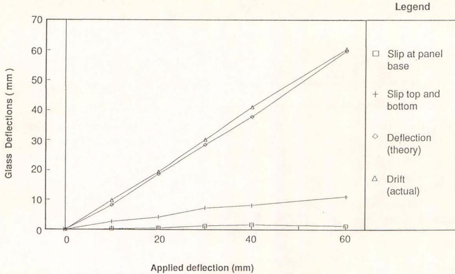
Figure 18 Components of Inter-storey deflection (First Panel) (Wall NG)
