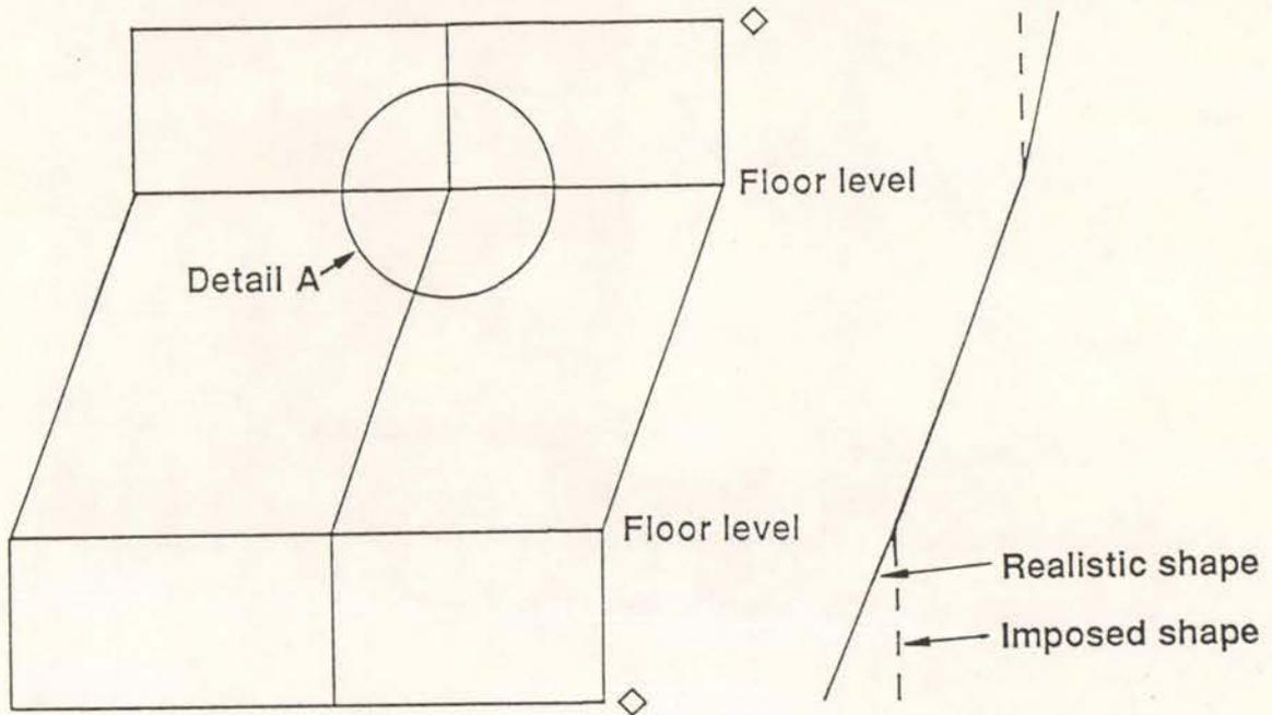
(a) Deformed shape imposed
