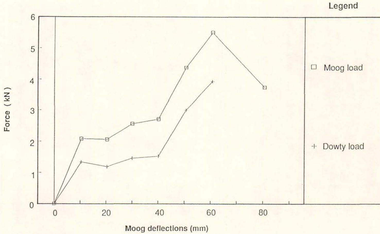
Figure 31 Peak actuator loads versus Moog deflection (Walls4)
