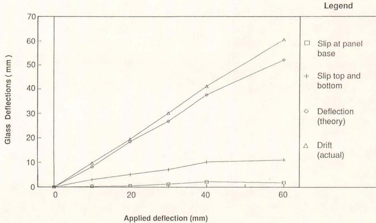
Figure 19 Components of Inter-storey deflection (Second Panel) (Wall NG)
