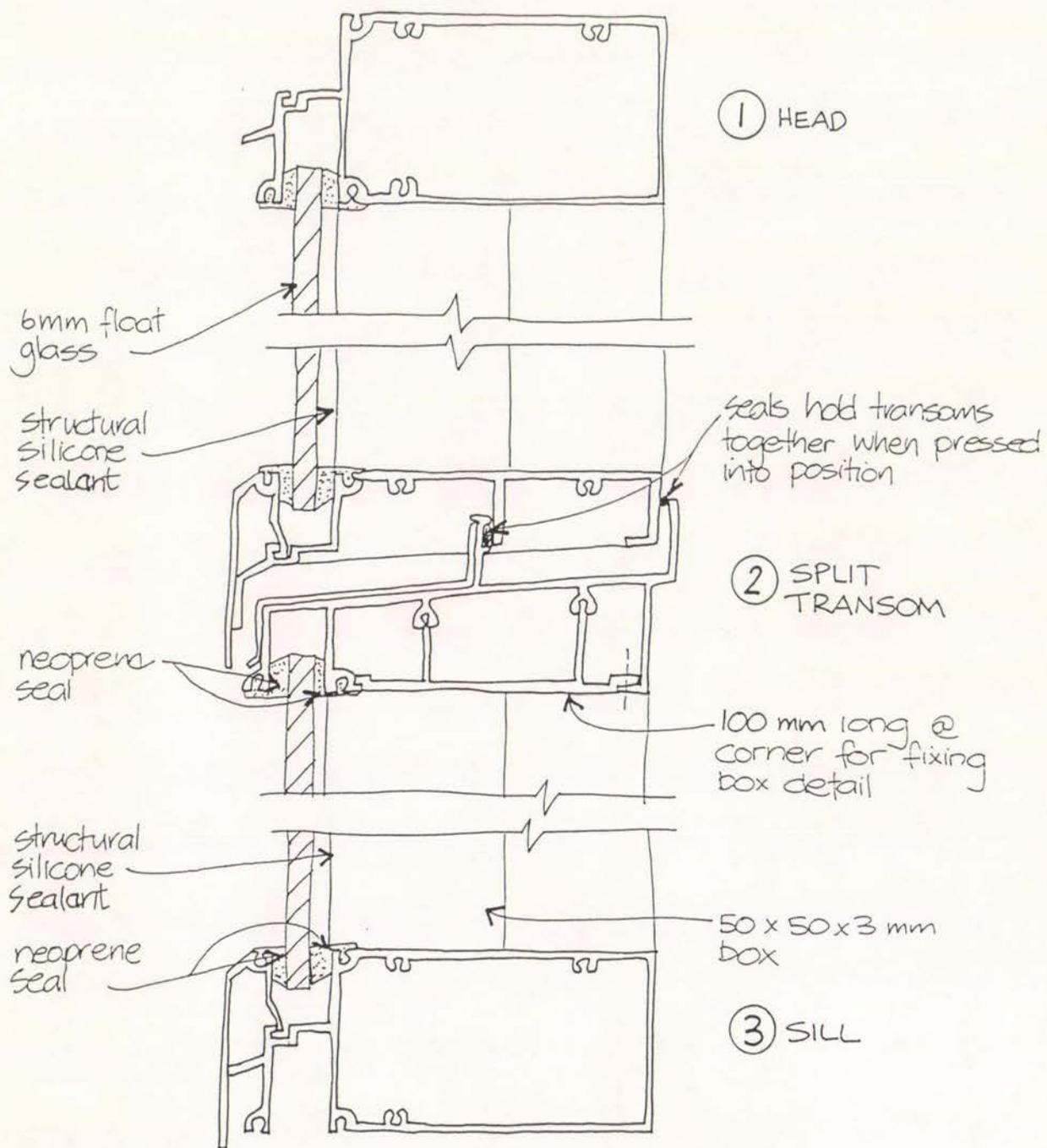
Figure 9b Cross-section through transoms (Wall S2)
