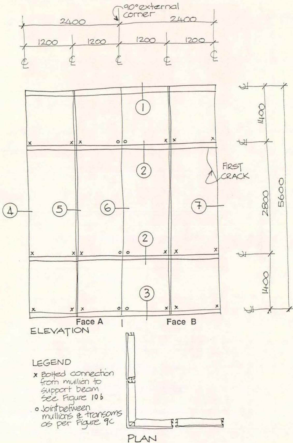
Figure 9a Dimensions of two sided silicone system (Wall S2) & location of first crack during testing
