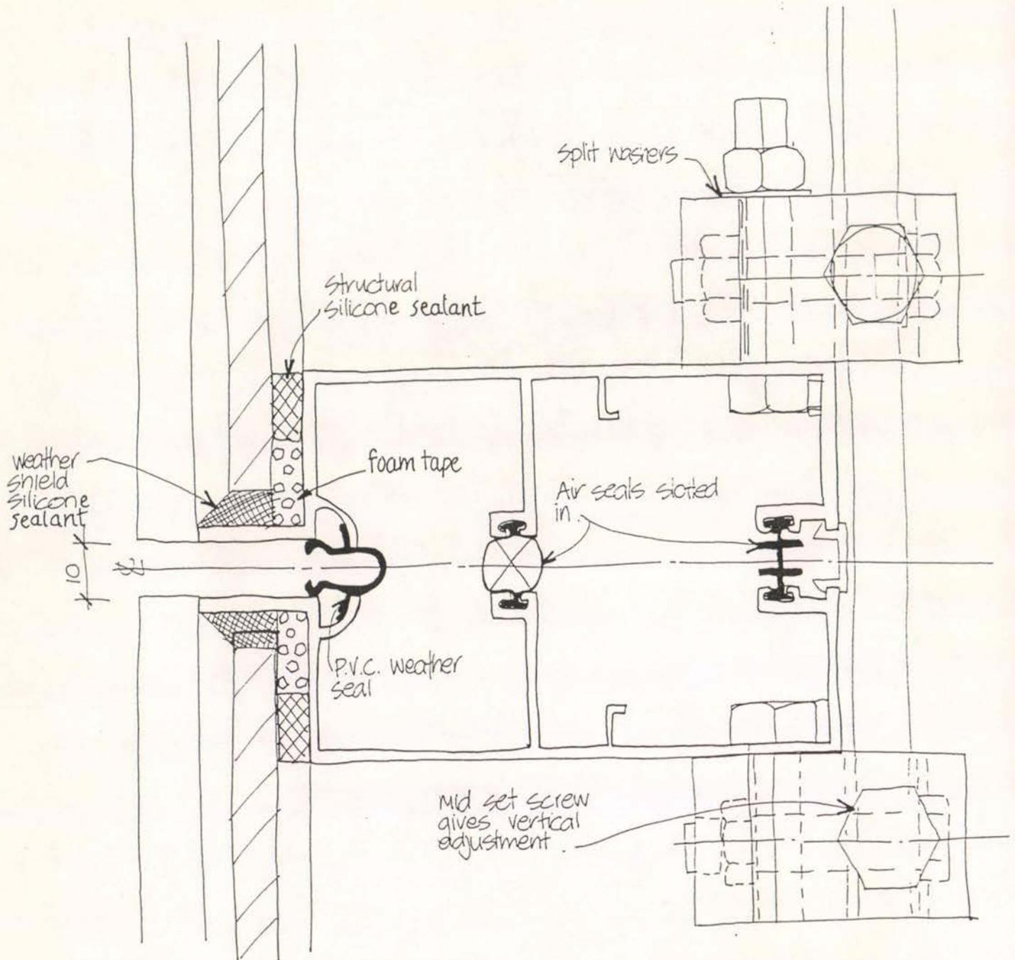
Figure 9d Detail 5 Cross-section through mullions showing connection details(Wall S2)
