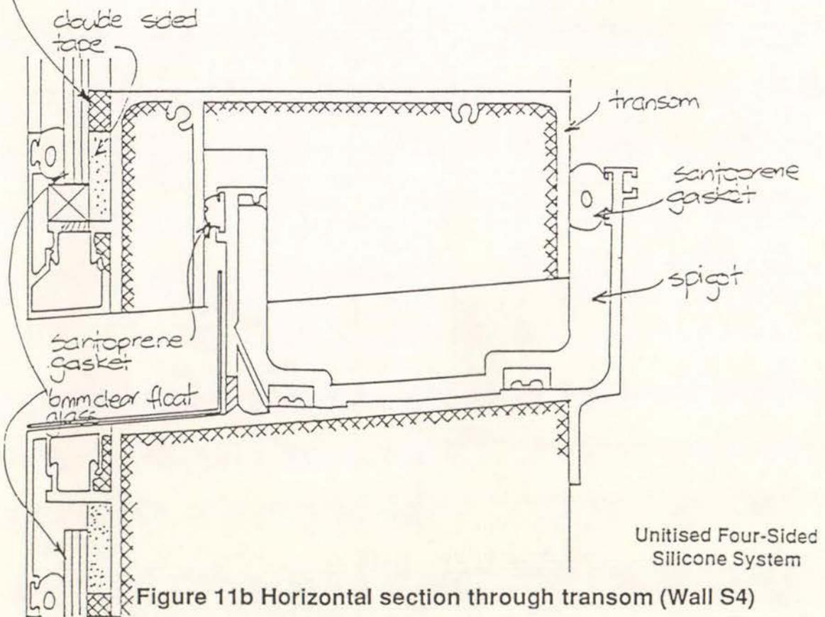
Figure 11b Horizontal section through transom (Wall S4)
