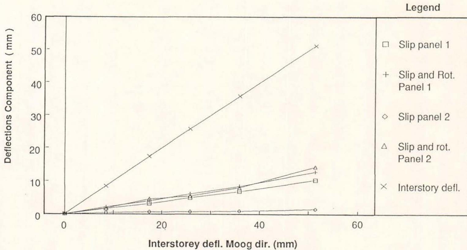
Figure 25 Deflection due to glass movement in silicone sealant (Wall S2)
