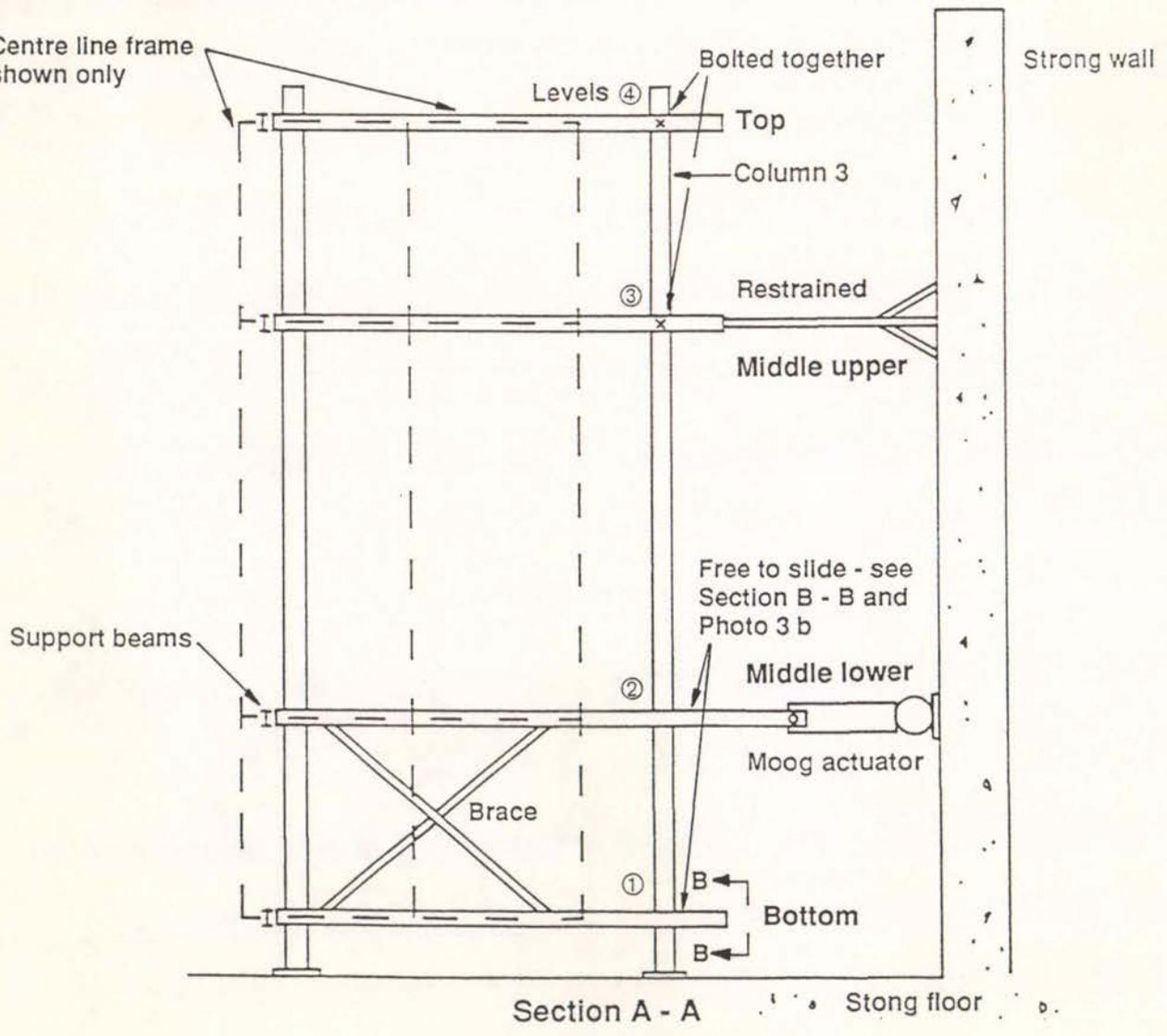
Figure 1 General test set-up.
