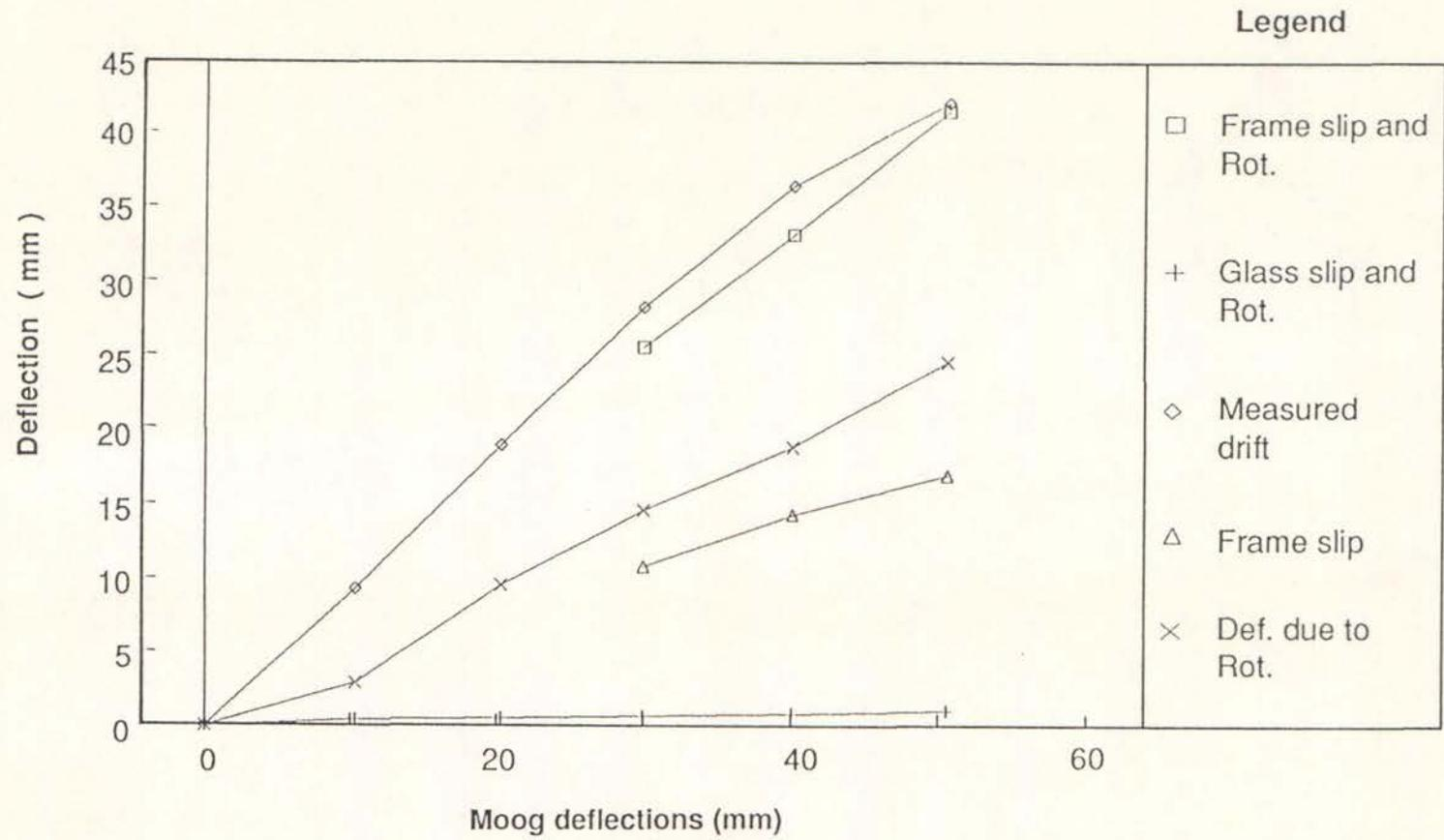
Figure 34 Components of applied deflection (Walls4)
