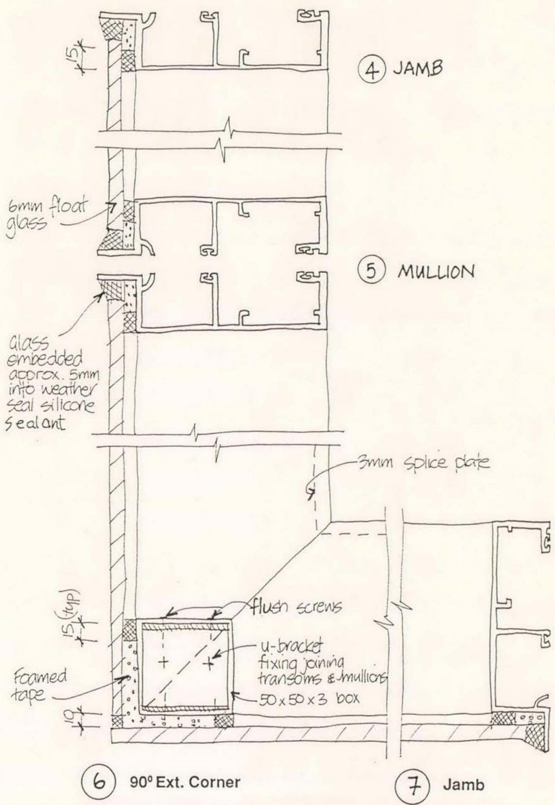
Figure 9c Cross-section views through mullions (Wall S2)
