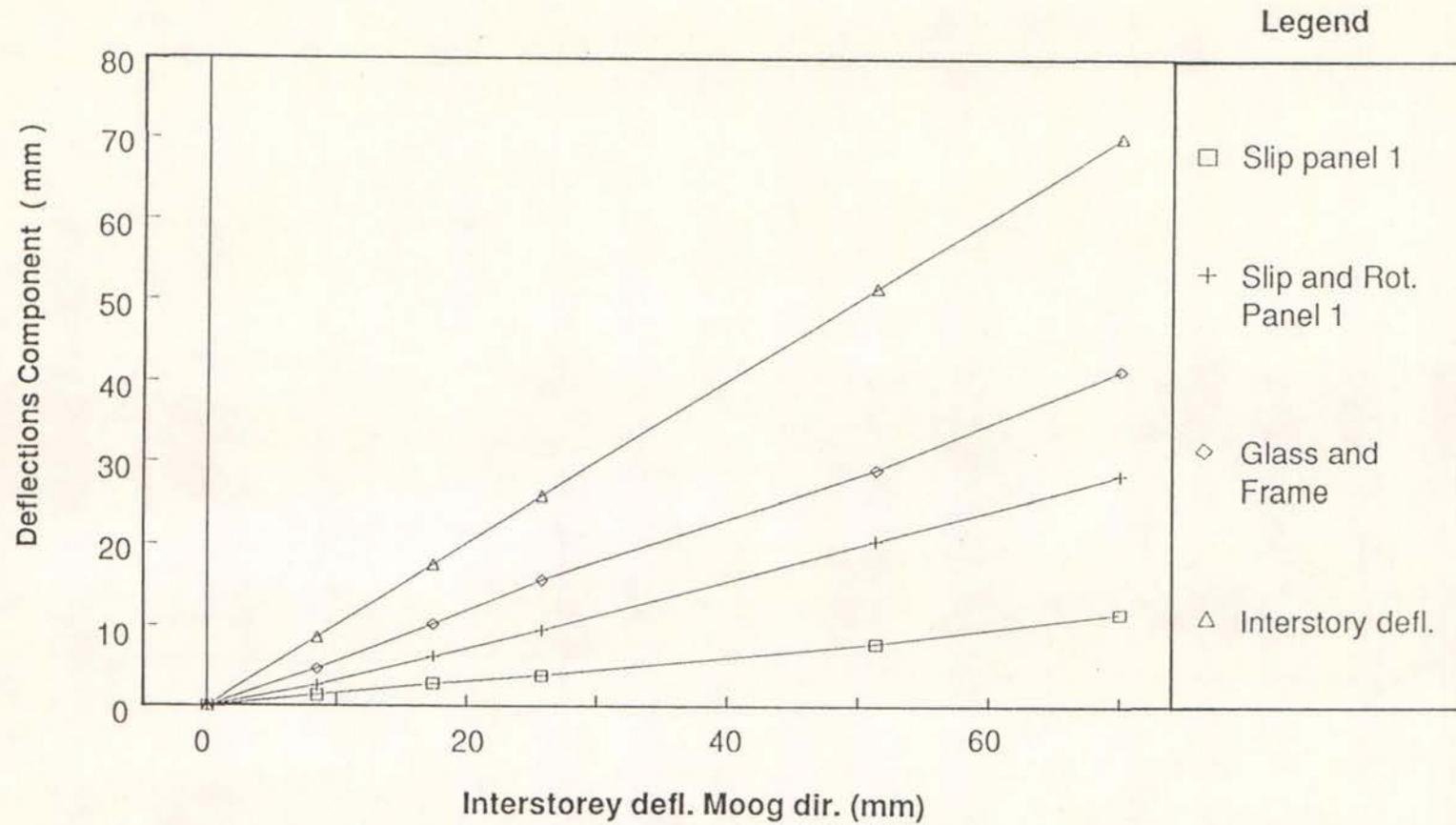
Figure 26 Deflection due to glass movement and frame movement ( Wall S2 )
