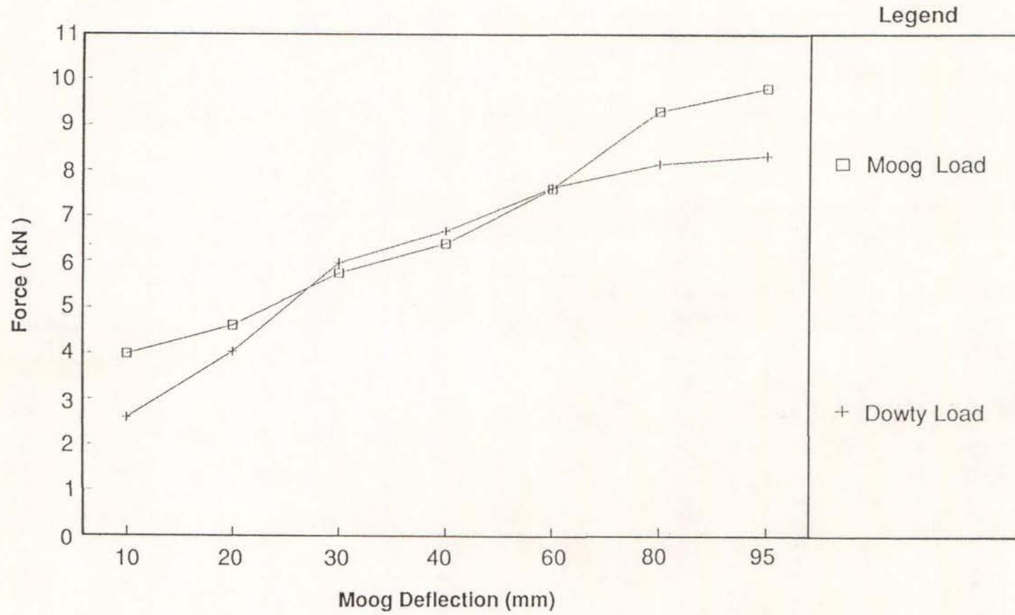
Figure 14 Peak actuator loads versus Moog deflection ( Wall NG )
