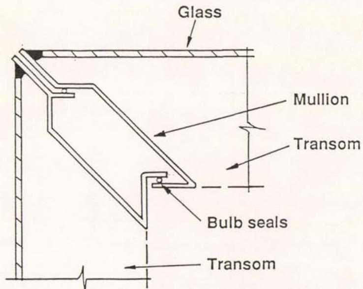
Figure 11d Plan - Preferred site corner detail using split mullion (Wall S4)
