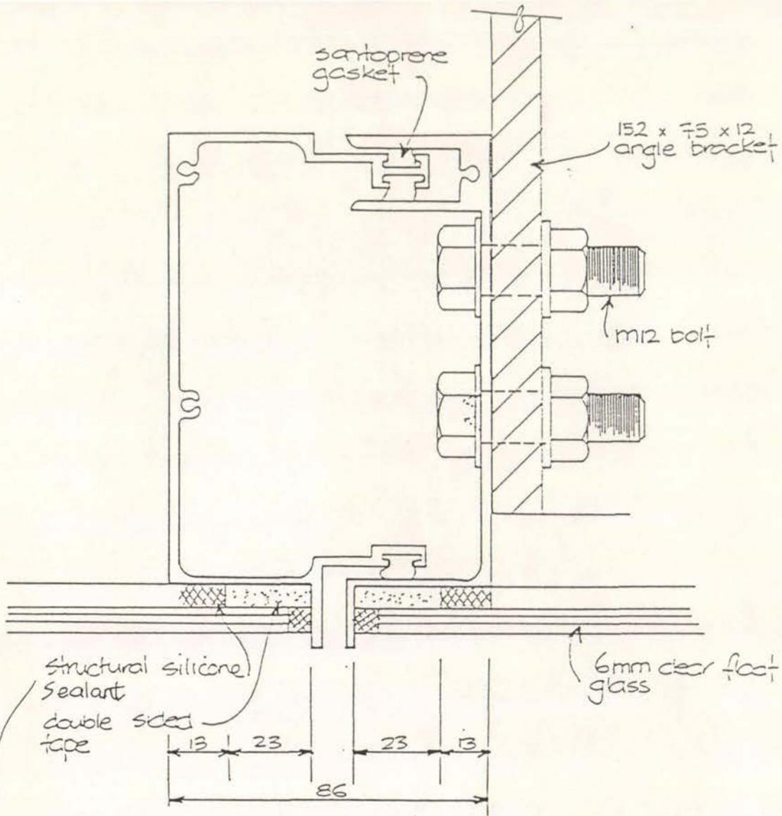
Figure 11a Vertical section through mullion (Wall S4)
