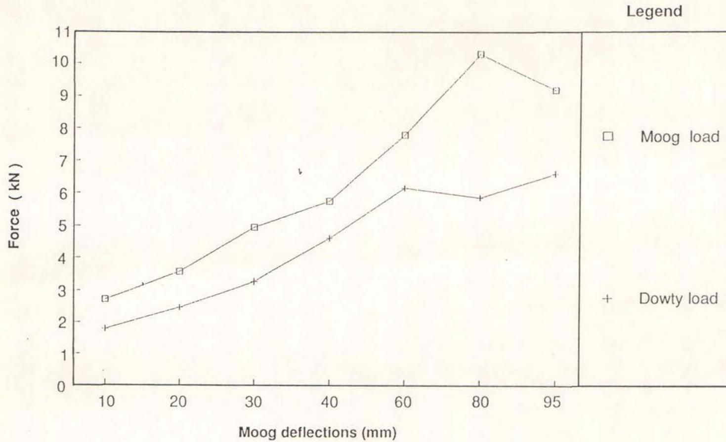
Figure 22 Peak actuator loads versus Moog deflection (Wall S2)
