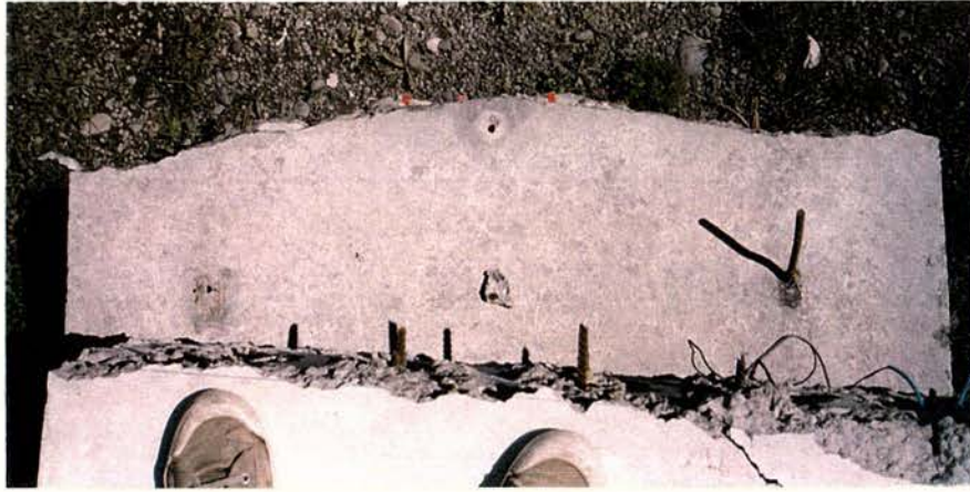
Fig. 3.27 End view of hollow core unit, showing inclined planes of fracture caused by combined shear and tension at the support
