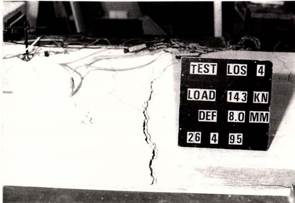
Fig. 3.66 Crack through composite topping at 8mm horizontal displacement, corresponding with the onset of topping mesh fracture
