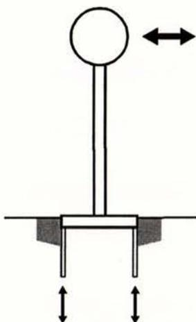
Figure 1. Earthquake induced axial loads on bored piles.
