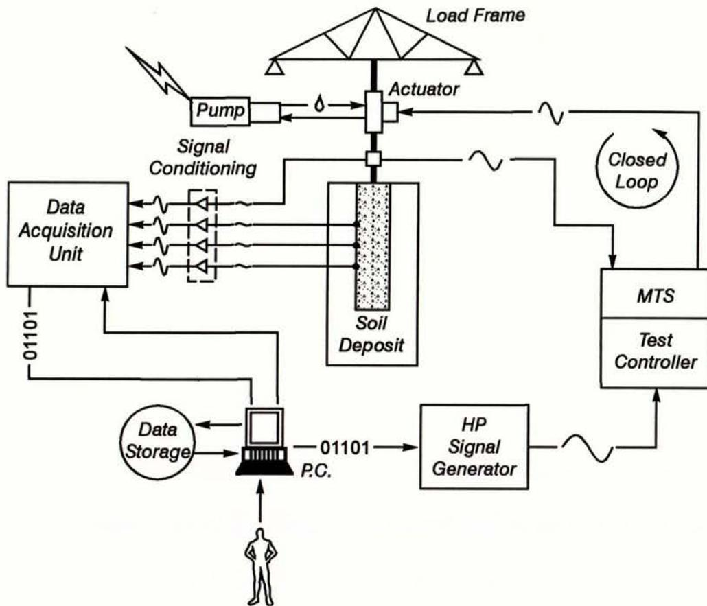
Figure 19. The overall load test system
