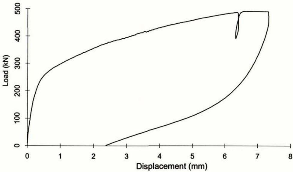
Figure 22. Load versus displacement for monotonic uplift load test EQC04
