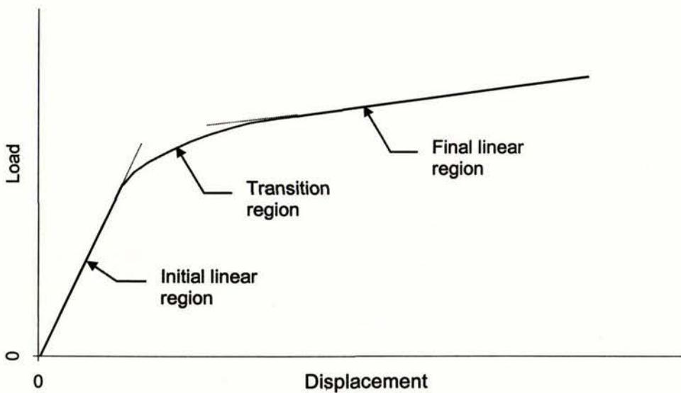
Figure 23. Regions of load-displacement curve.
