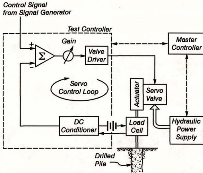
Figure 18. Servo control system.
