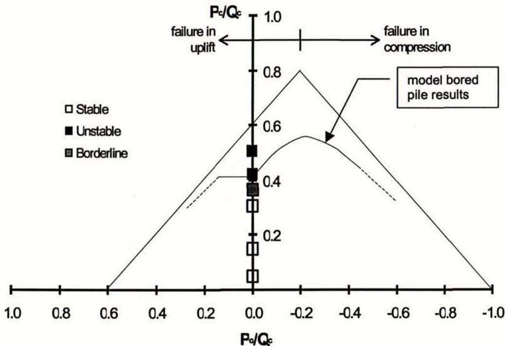
Figure 28. Cyclic stability diagram for full-size bored piles.
