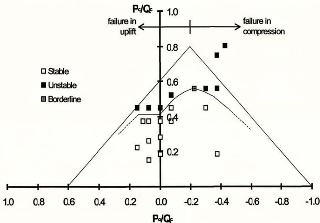
Figure 4. Cyclic stability diagram for model bored piles with simulated earthquake loading.
