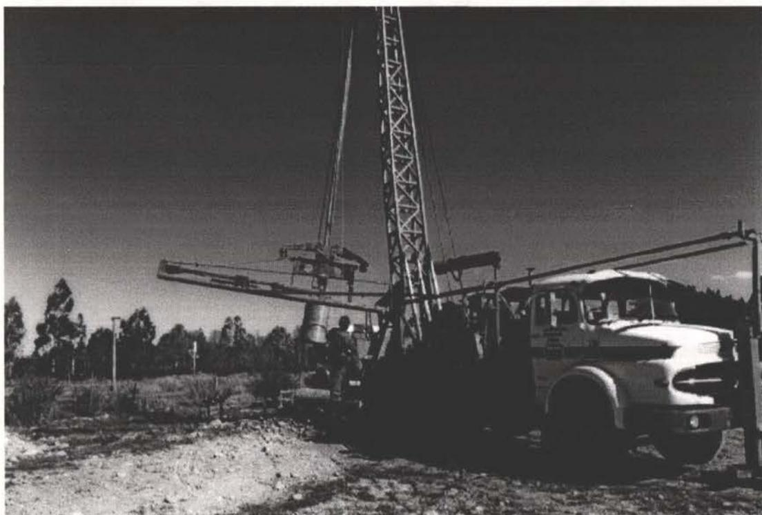
Figure 11. Truck mounted Calweld bucket auger rig.
