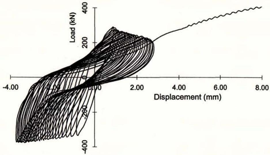
Figure 26. Load versus displacement for test EQC07B (LRL = 0.70)
