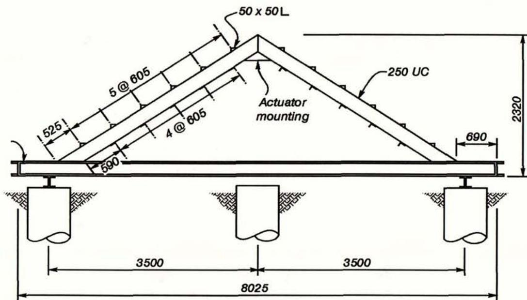
Figure 16. Loading truss details.
