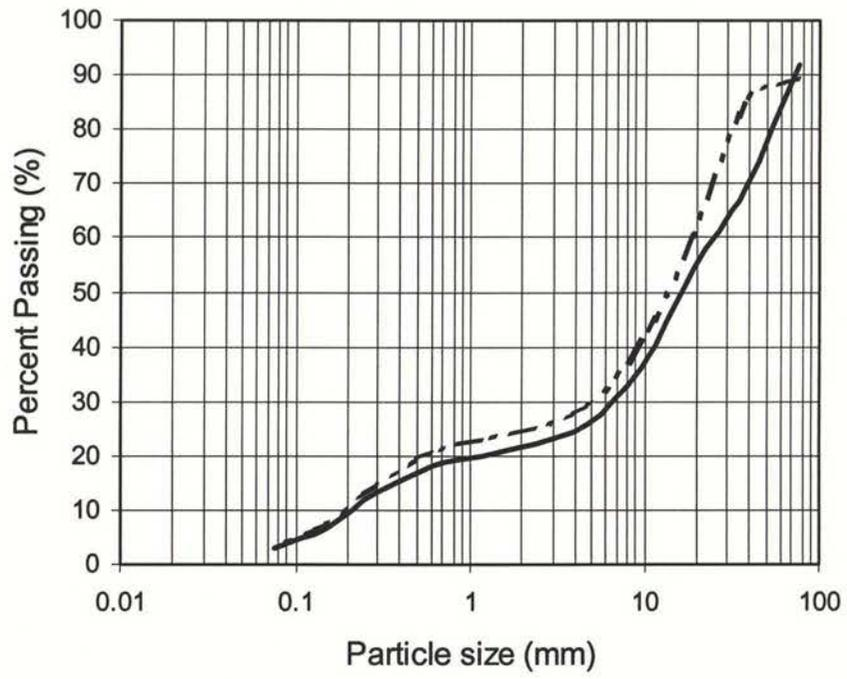
Figure 9. Particle gradation curves for test soil.
