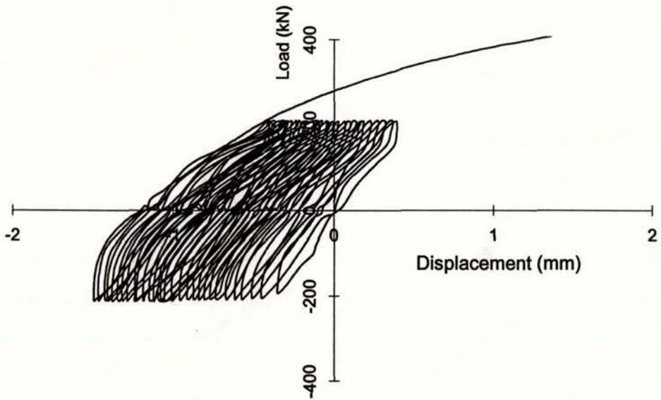
Figure 27. Load versus displacement for test EQC09B (LRL = 0.50)
