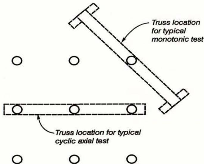
Figure 15. Truss layout for monotonic uplift and cyclic load tests.
