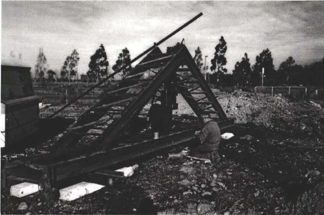
Figure 17. View of loading truss and actuator.
