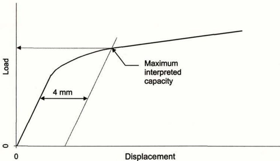
Figure 24. Uplift slope tangent method.
