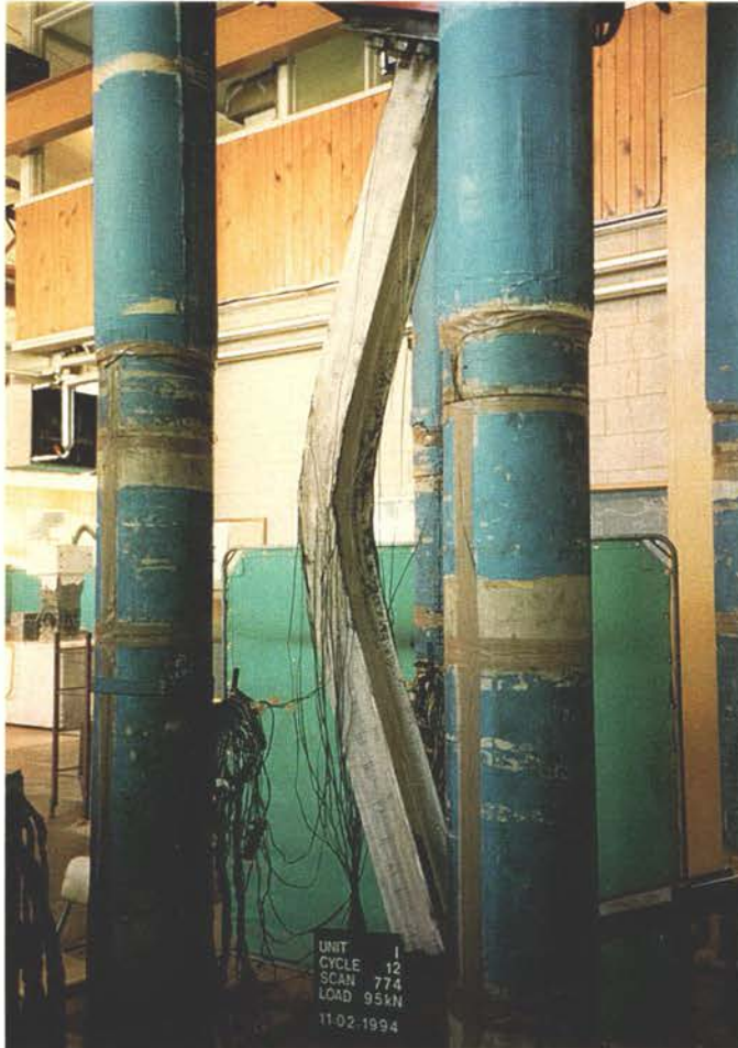
(a) Overall view at maximum compression of cycle 12
