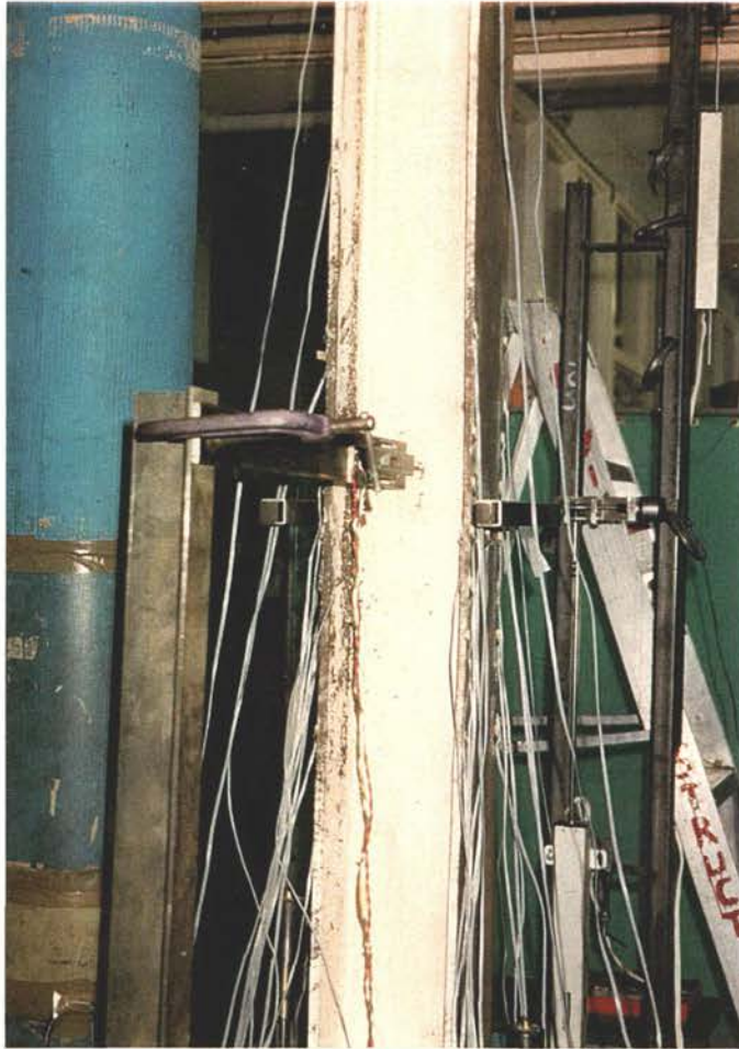
(c) Restraightening of local buckling in cycle 9
