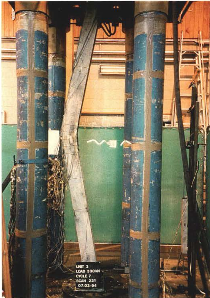
(a) Overall view at maximum compression of cycle 7
