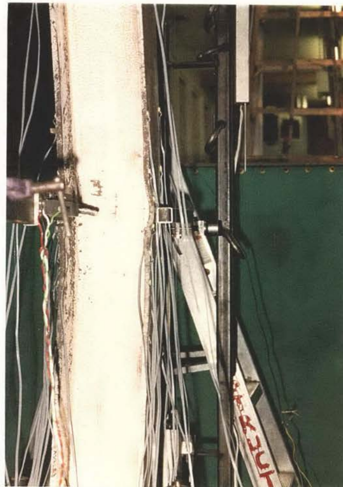
(b) Local buckling at centre hinge in cycle 8
