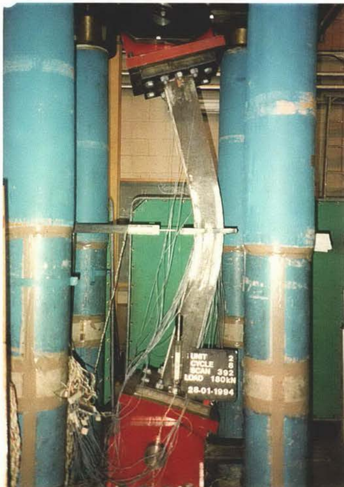
(a) Overall view at maximum compression of cycle 8
