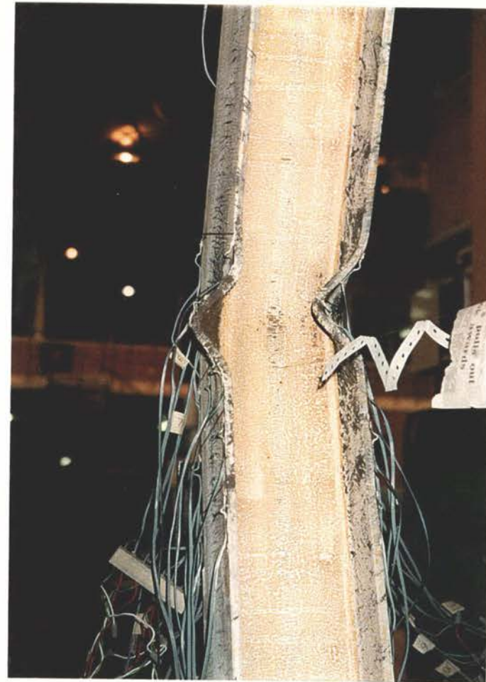
(f) Local buckling at centre hinge in cycle 8
