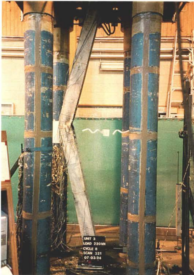
(e) Overall view at maximum compression of cycle 8
