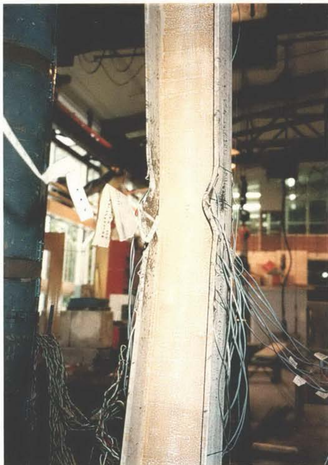
(c) Local buckling at centre hinge in cycle 7
