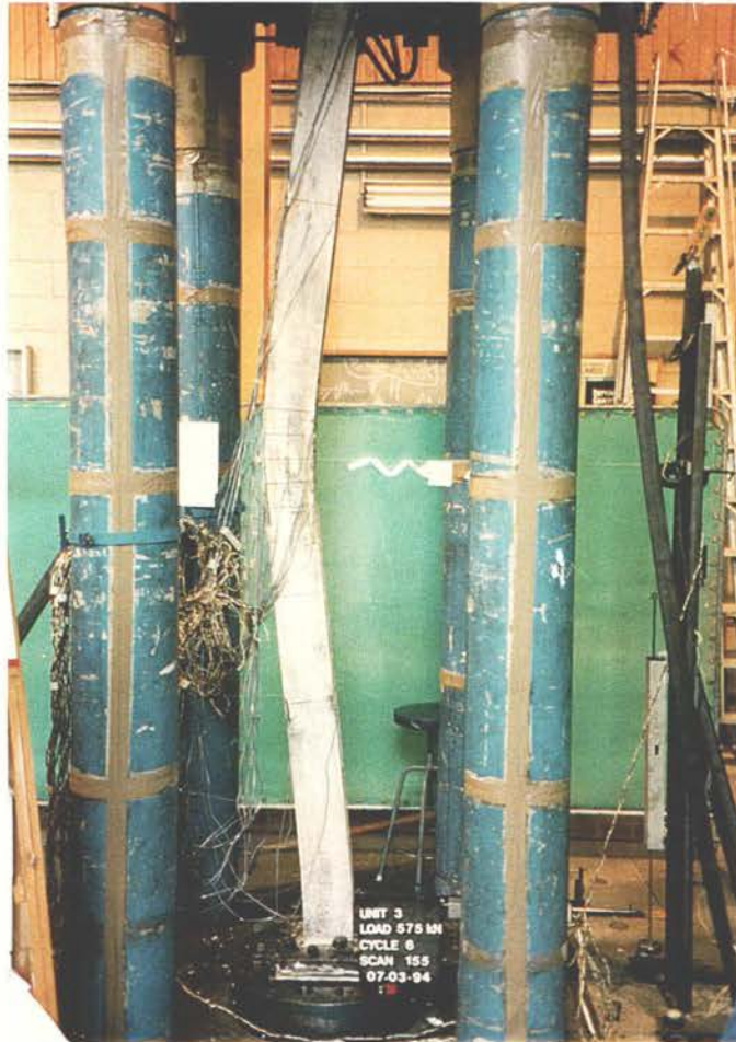
(a) At maximum compressive axial displacement
