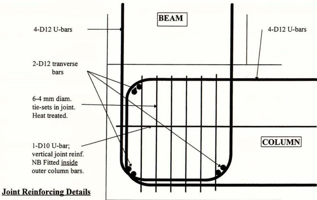
**Figure 2: Knee Joint 2 designed to 1995 Standard, with small diameter bars (D12 U-bars).**
