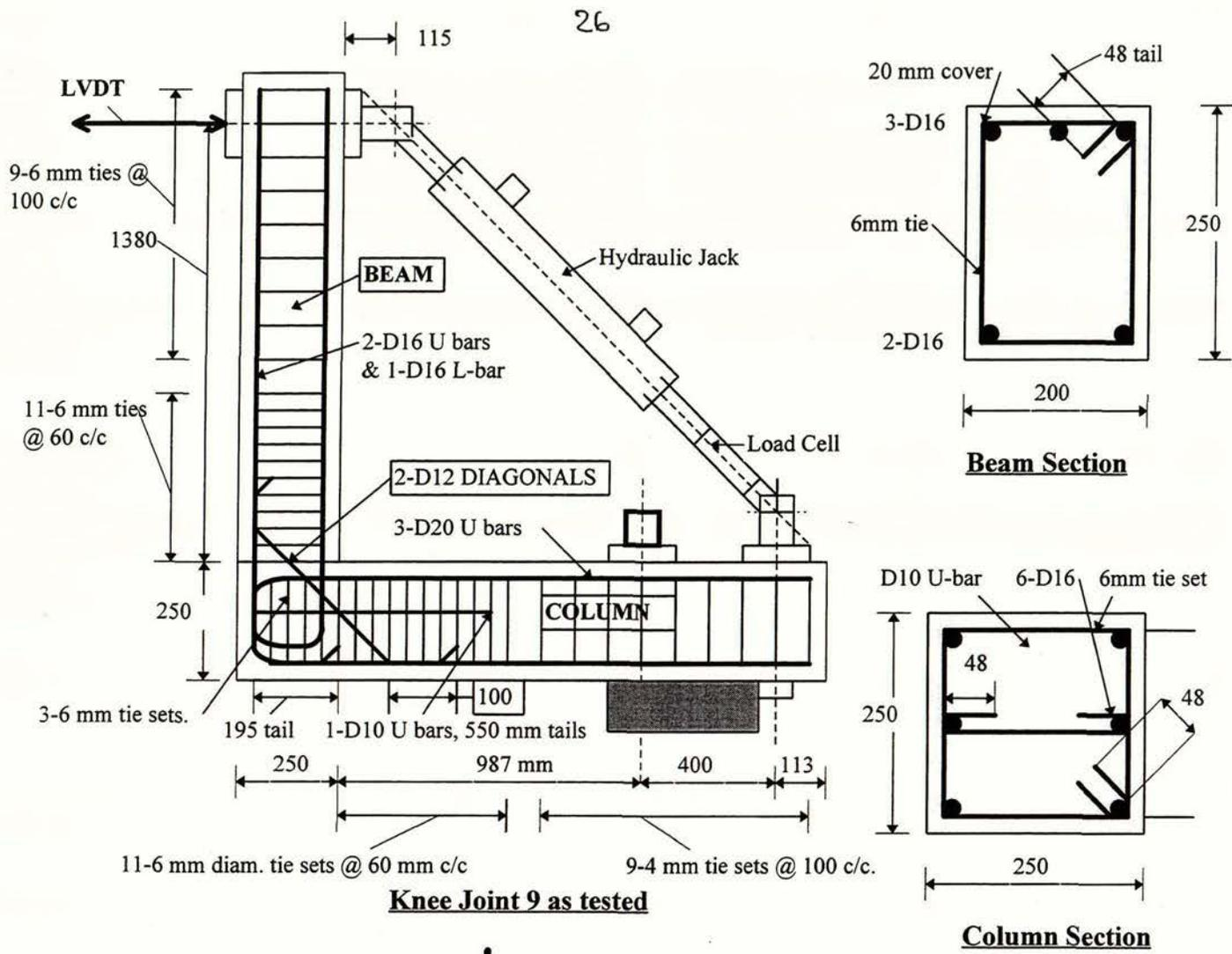
**Figure 9: Knee Joint 9 designed to 1995 Standard with unequal top and bottom beam bars plus two extra diagonal bars.**
