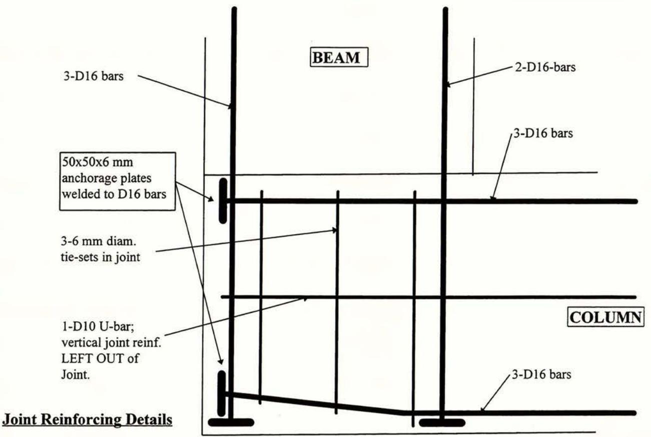
**Figure 46: Knee Joint 11 with anchorage plates. 3 Transverse joint ties included.**
