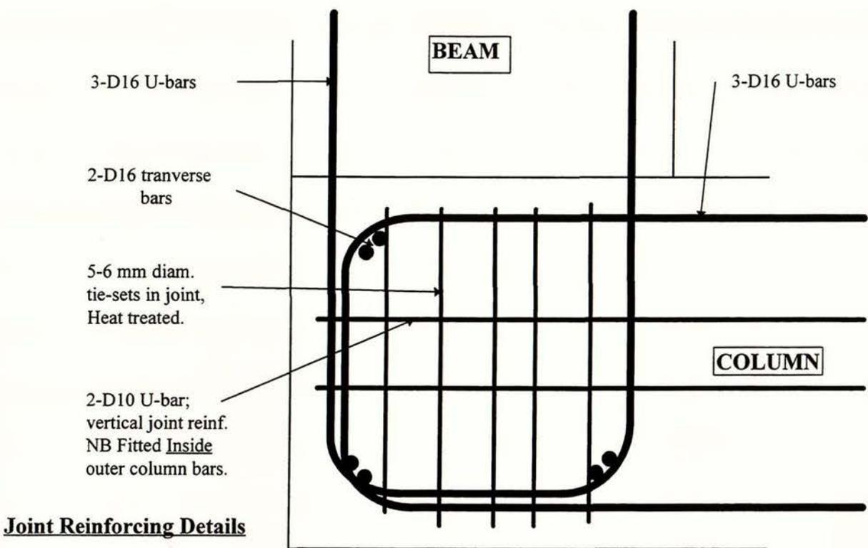
**Figure 3: Knee Joint 3 designed to 1995 Standard with D16 U-bars.**
