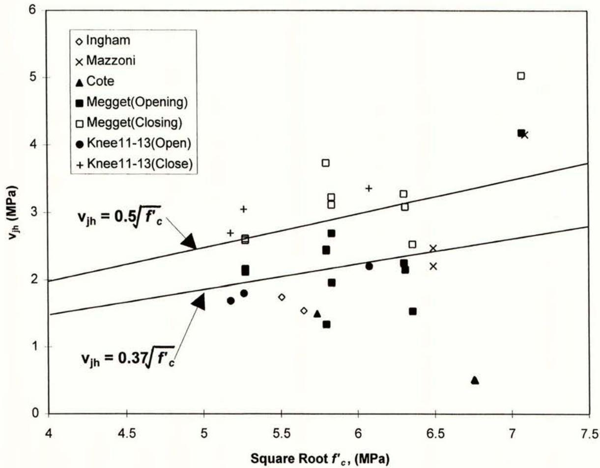
Figure 58: Maximum Joint Shear Stress versus Square Root of Concrete Compressive Stress for all cyclic loaded beam-column knee joint tests.
