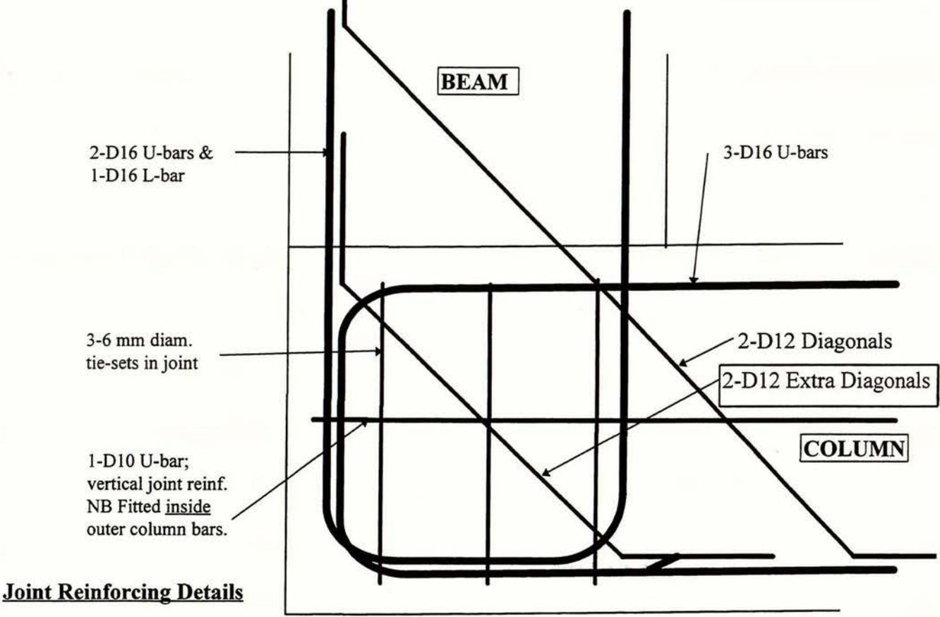
**Figure A1: Knee Joint 9 designed to 1995 Standard plus extra diagonal bars through joint.**
