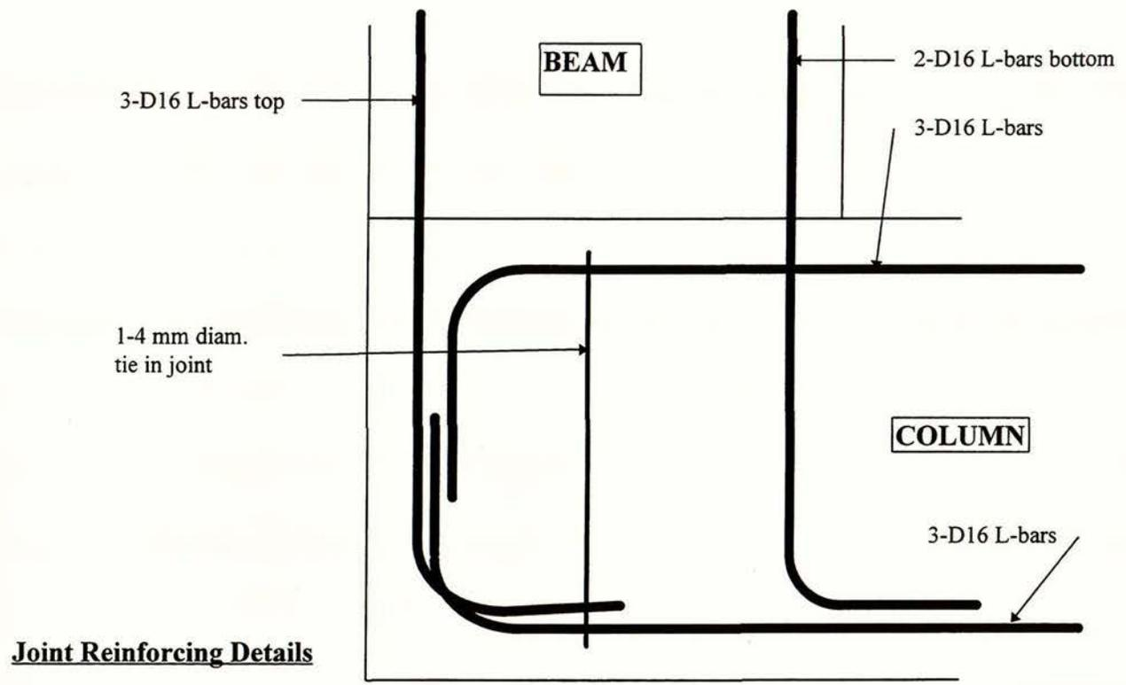
Figure 8: Knee Joint 8 designed to 1960's Code with deformed main bars.
