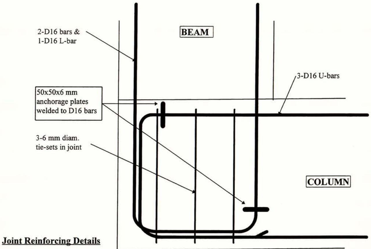
**Figure 48: Knee Joint 13 with an anchorage plate on each U-bar. 3 tranverse joint ties.**
