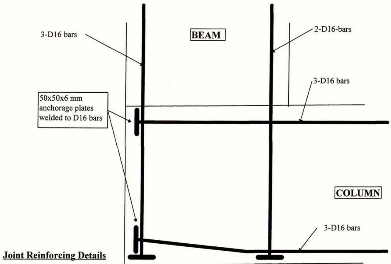
**Figure 47: Knee Joint 12 with anchorage plates and no joint shear reinforcing.**
