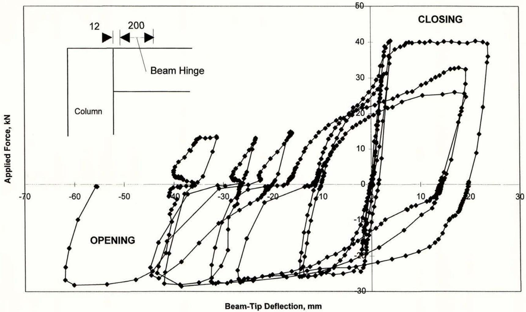
FIGURE 38: KNEE 10 Applied Force - Beam zone 2 Deflection, 212 mm out from the column face, calculated at the beam-tip.
