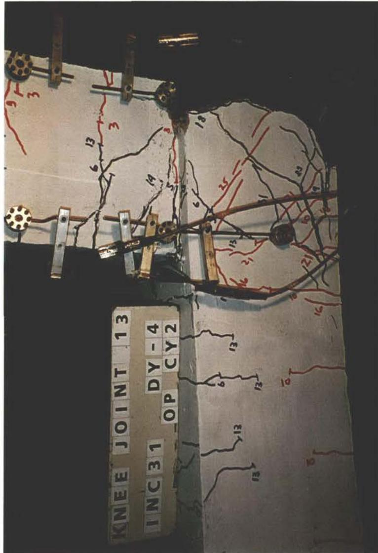
FIGURE 56: Knee 13, U-bars & anchorage plates, at second cycle to opening ductility -4.
