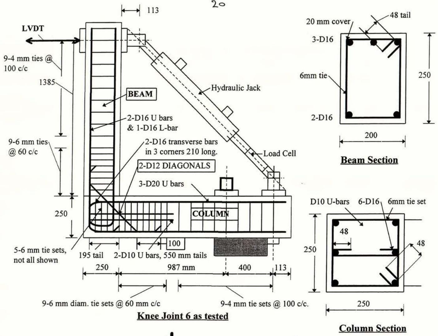
**Figure 6: Knee Joint 6 designed to 1995 Standard plus two extra diagonal bars.**
