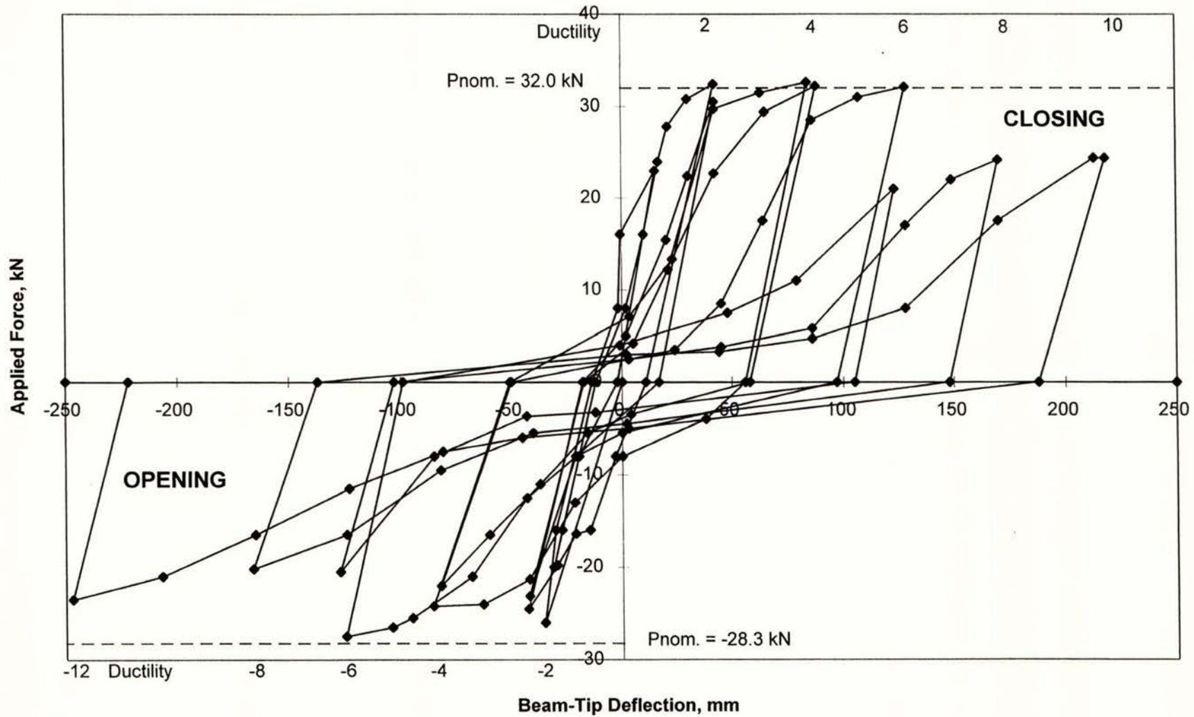
**FIGURE 18: KNEE 2 Flexure +Axial, Shear deformations and Measured Beam-Tip Deflections at cycle peaks.**
