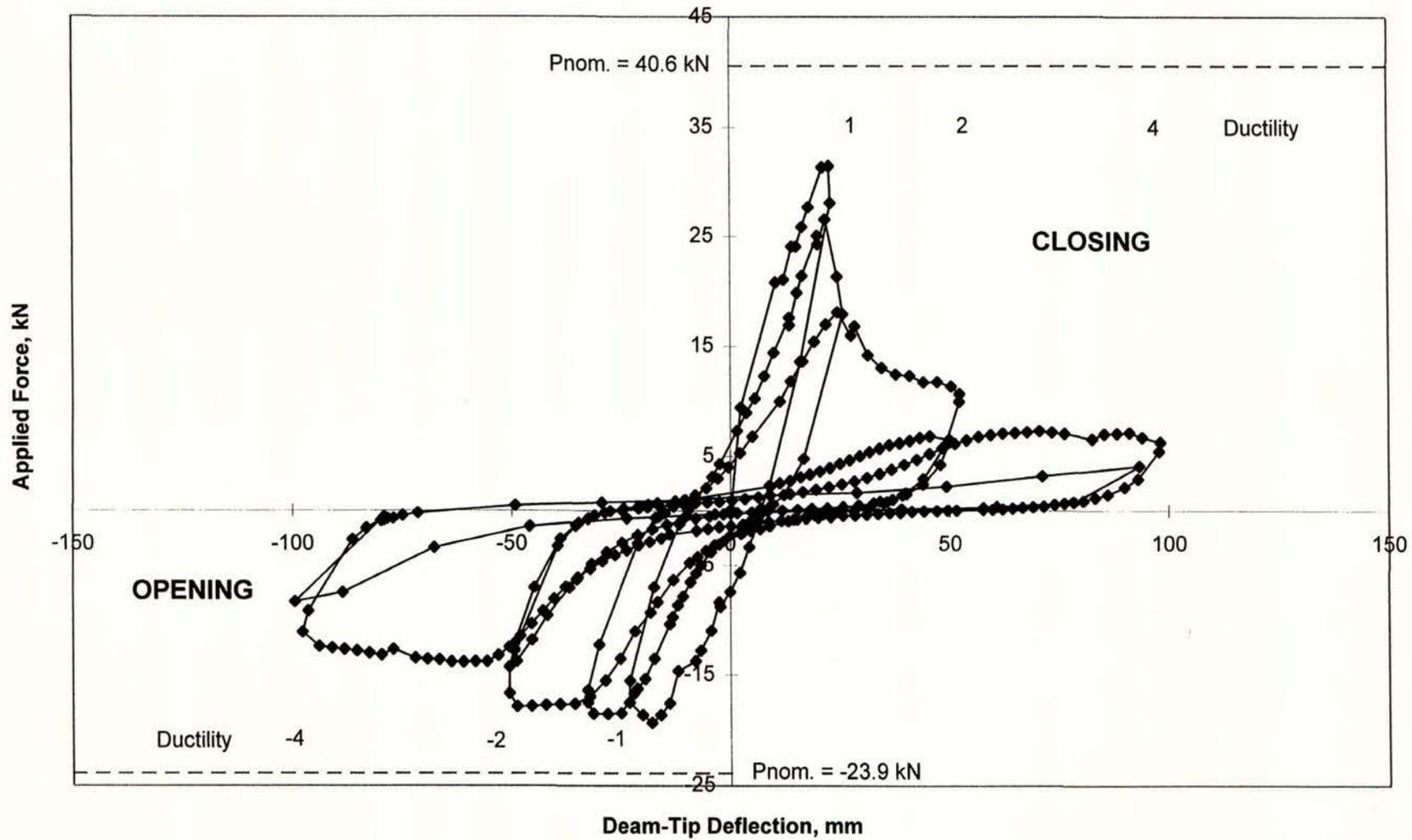
**FIGURE 45: KNEE 8 Flexure+Axial & Shear Deformations and Measured Beam-Tip Deflections at cycle peaks.**
