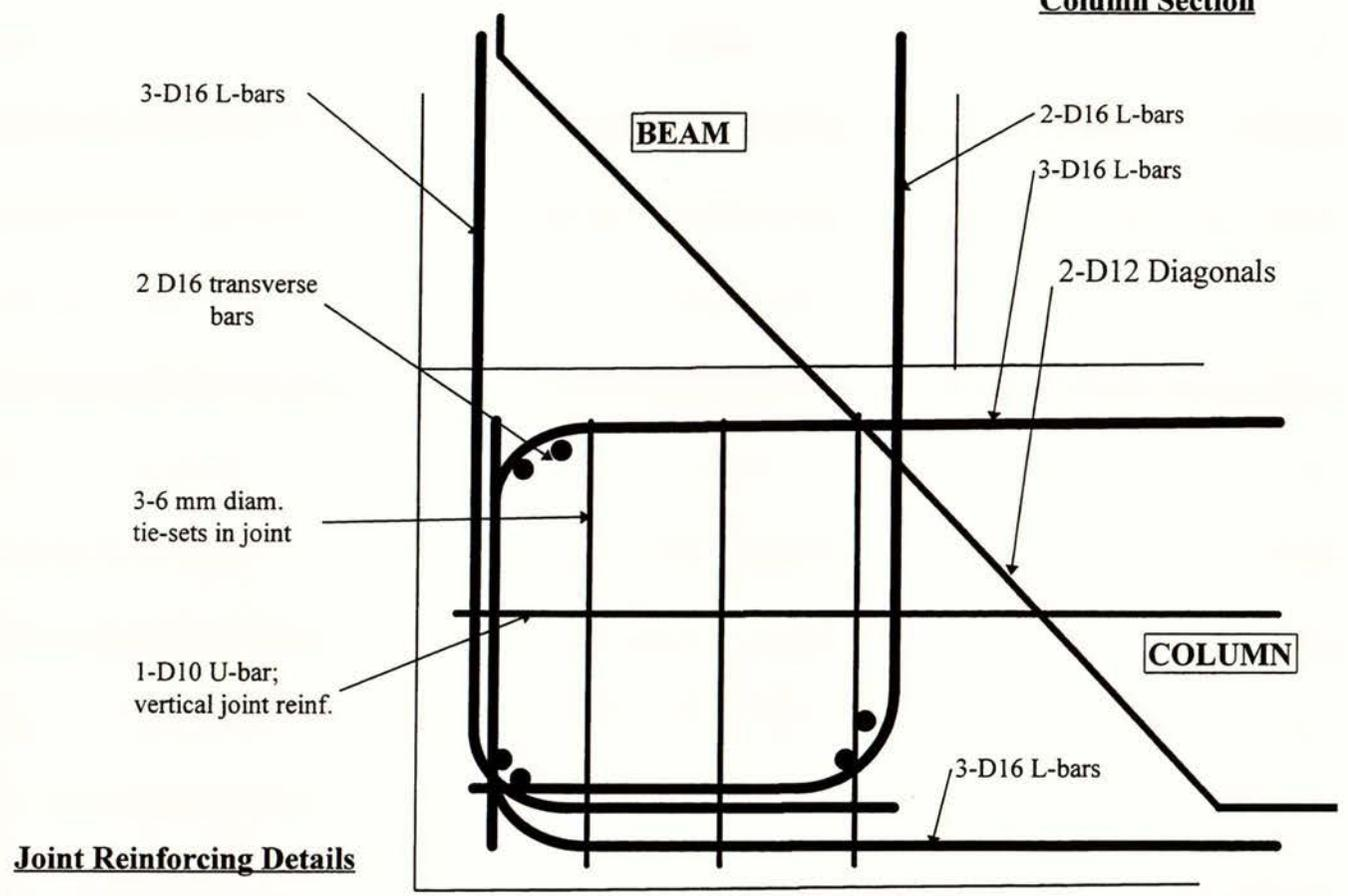
**Figure 10: Knee Joint 10 designed to 1995 Standard; main bars with standard hooks, plus two extra diagonal bars.**
