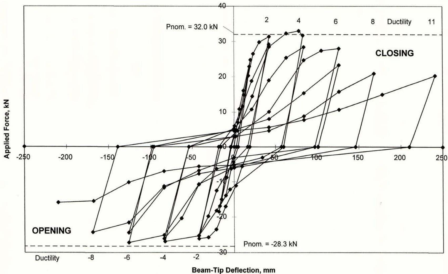
**FIGURE 14: KNEE 1 Flexure+Axial, Shear deformations and Measured Beam-Tip Deflection at cycle peaks.**
