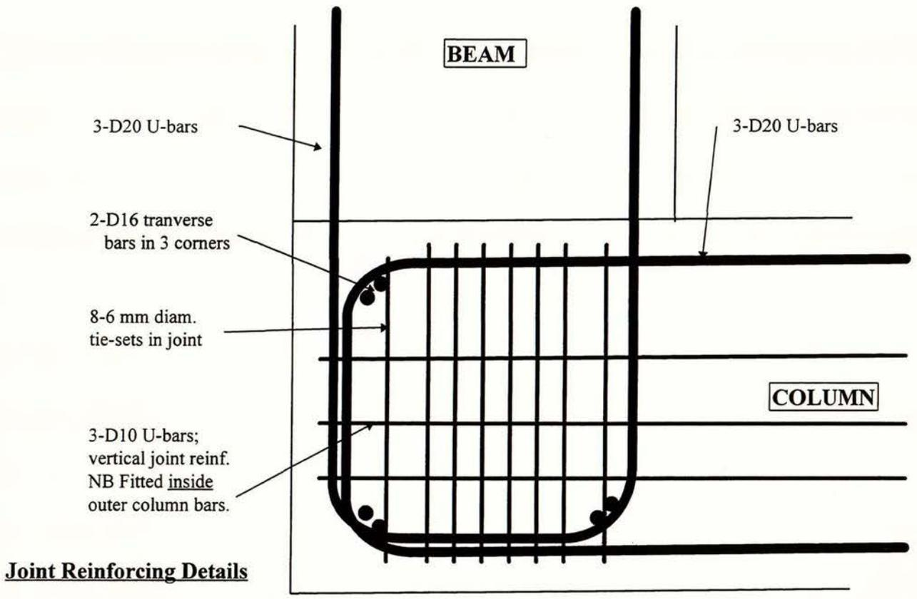
**Figure 7: Knee Joint 7 designed to 1995 Standard with D20 U-bars.**
