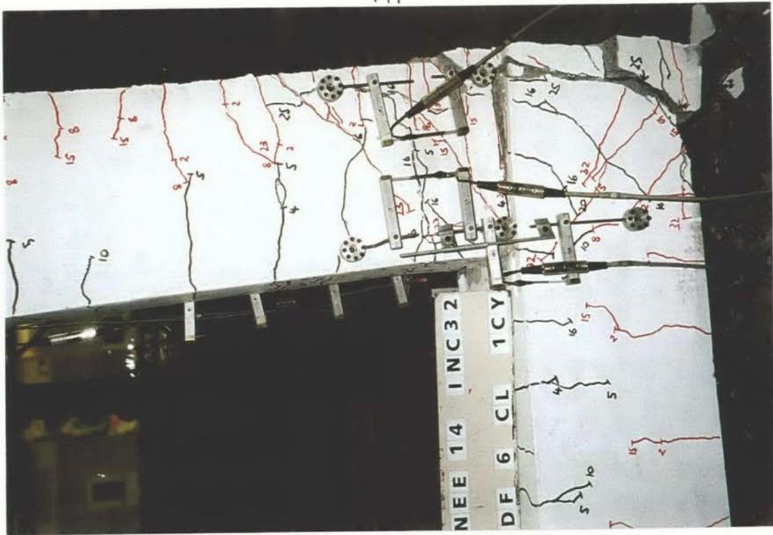
FIGURE A3: Knee 14 at first cycle to closing ductility 6.
