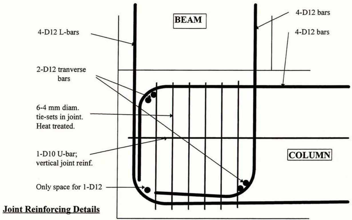
Figure 1: Knee Joint 1 designed to 1995 Standard, with small diameter bars (D12 standard hooks).
