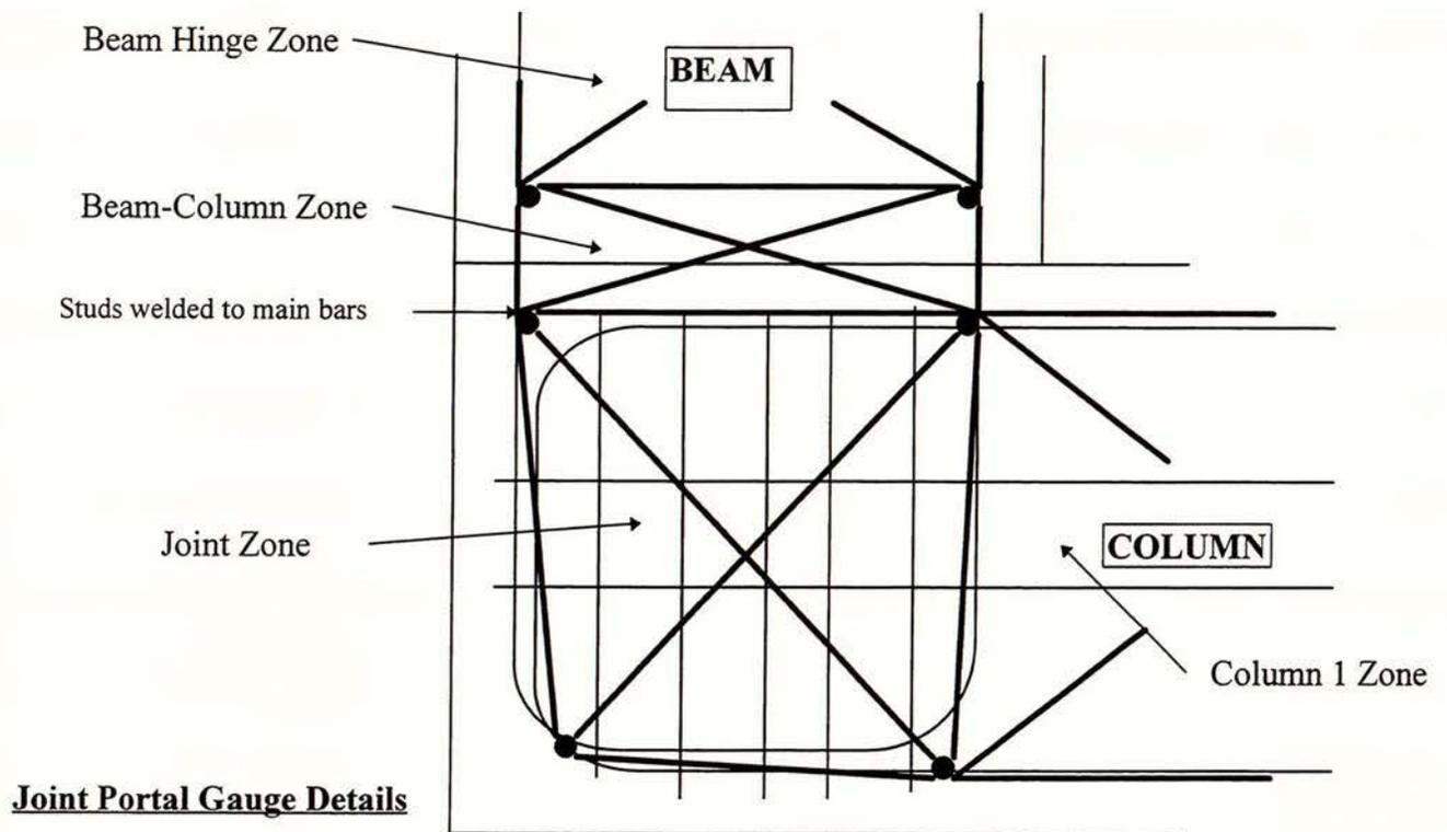
**Figure 11 Portal Transducer Gauge Positions on studs welded to main reinforcing bars.**
