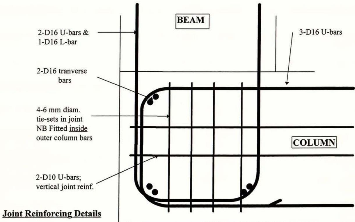
**Figure 4: Knee Joint 4 designed to 1995 Standard. U-bars with 1 extra top beam bar.**
