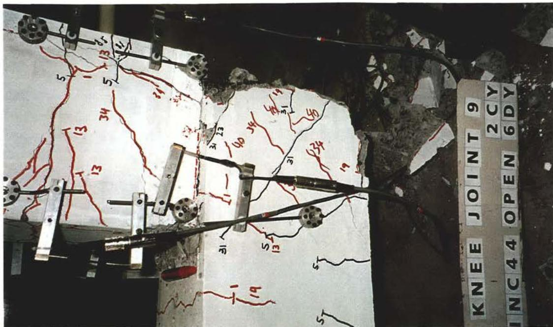
FIGURE 32: Knee 9 at second cycle to opening ductility -6.
