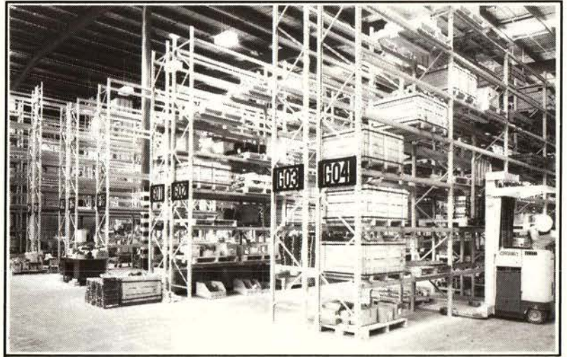
Figure 7.9 Note the height of these storage units in an Auckland warehouse and their substantial loading. Clearly stability in an earthquake is in question.
