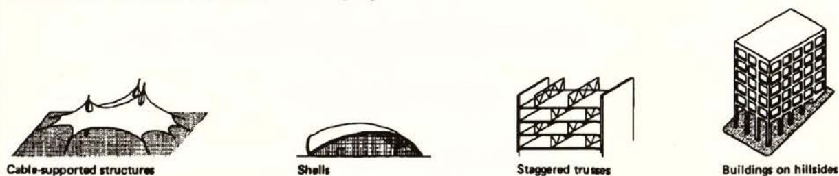
Figure 2.3 Graphic interpretation of irregular structures or framing systems from the Commentary to the SEAOC Recommended Lateral Force Requirements and Commentary.
